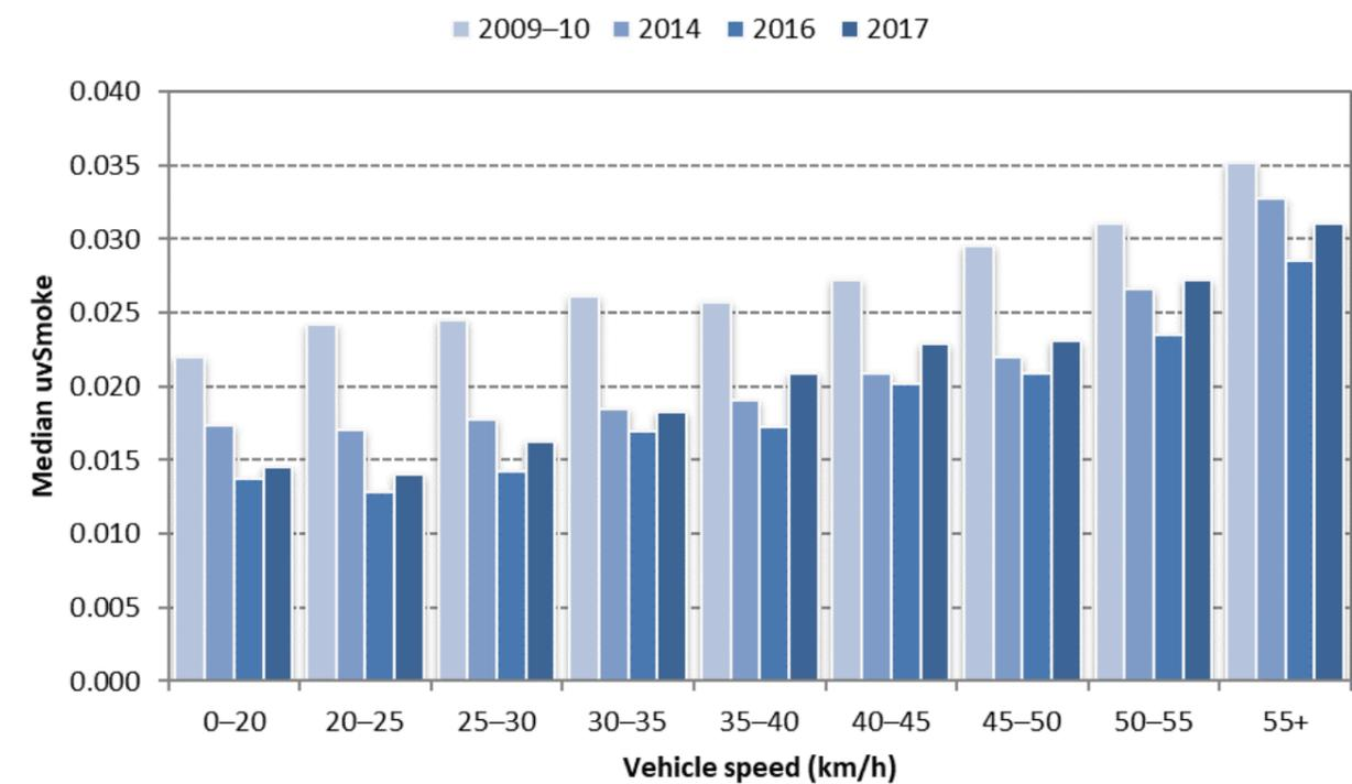
Figure 6: Median emissions over time per vehicle speed
