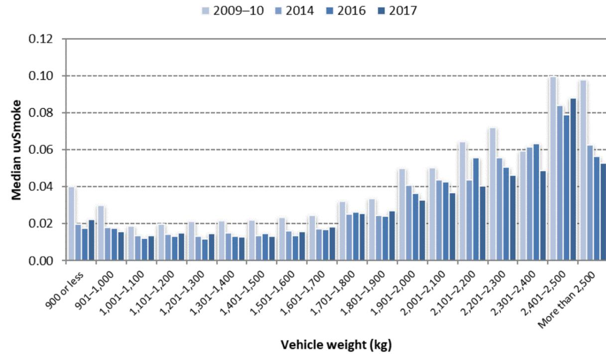
Figure 11: Median emissions over time per vehicle weight range
