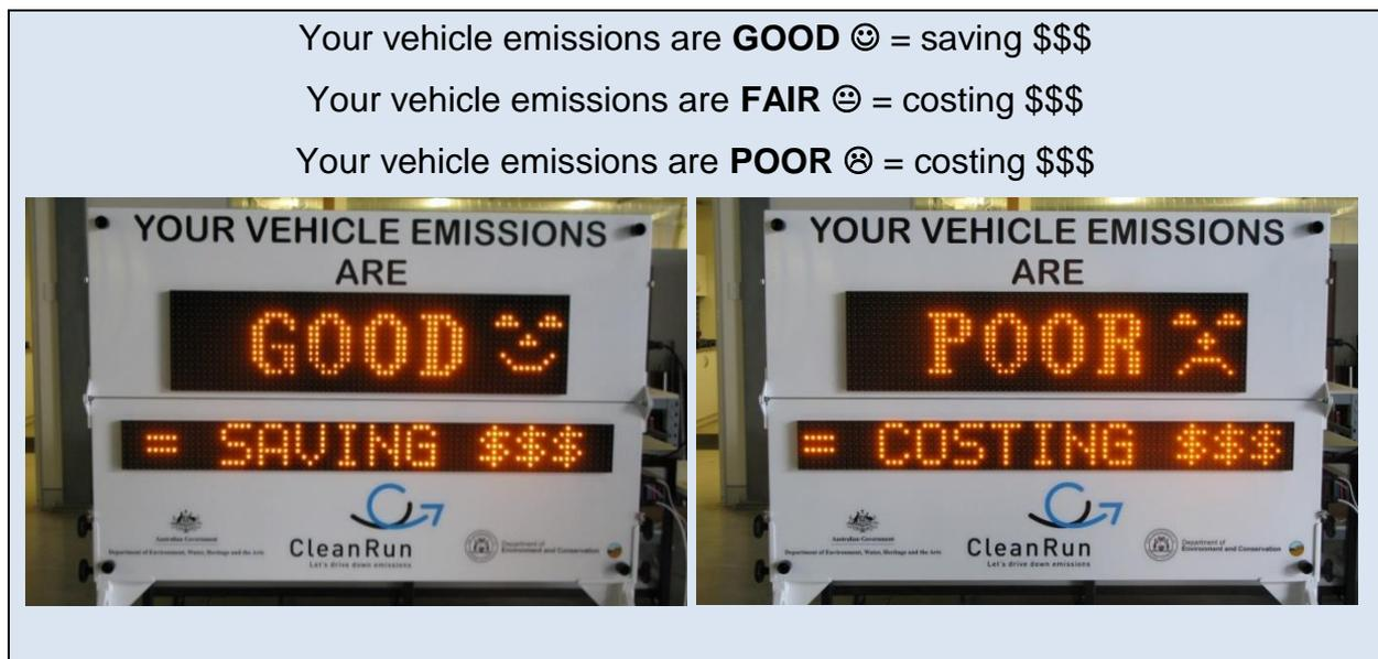
Figure 3: CleanRun smart sign vehicle emissions performance feedback display
