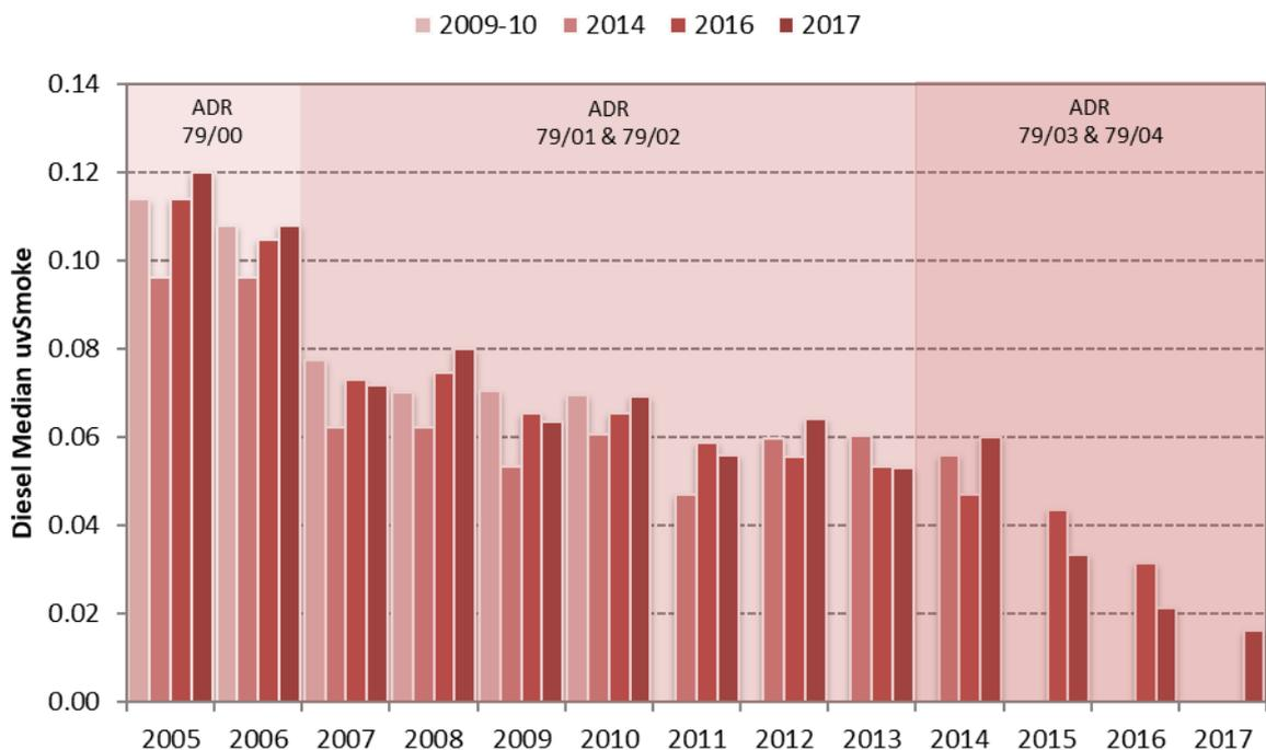
Figure 15: Median smoke emissions over time per year of manufacture
