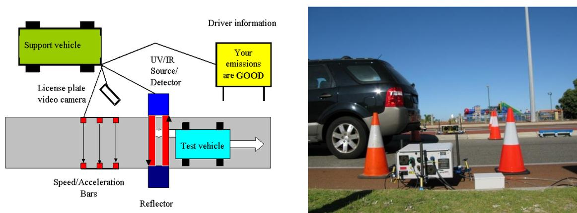
**Figure 1. Schematic diagram of the RSD monitoring equipment<sup>4</sup> (left) and RSD source/detector and reflector in operation<sup>5</sup> (right)**
