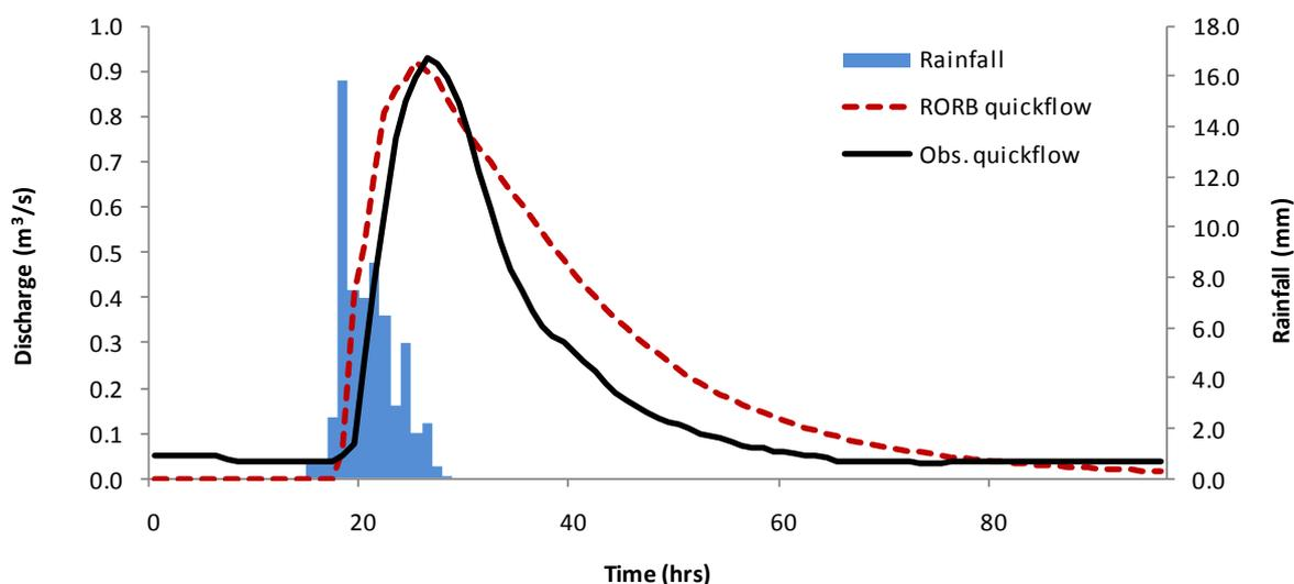
*Figure B-6: RORB modelled and observed flows for Peel Main Drain (August 1994)*
