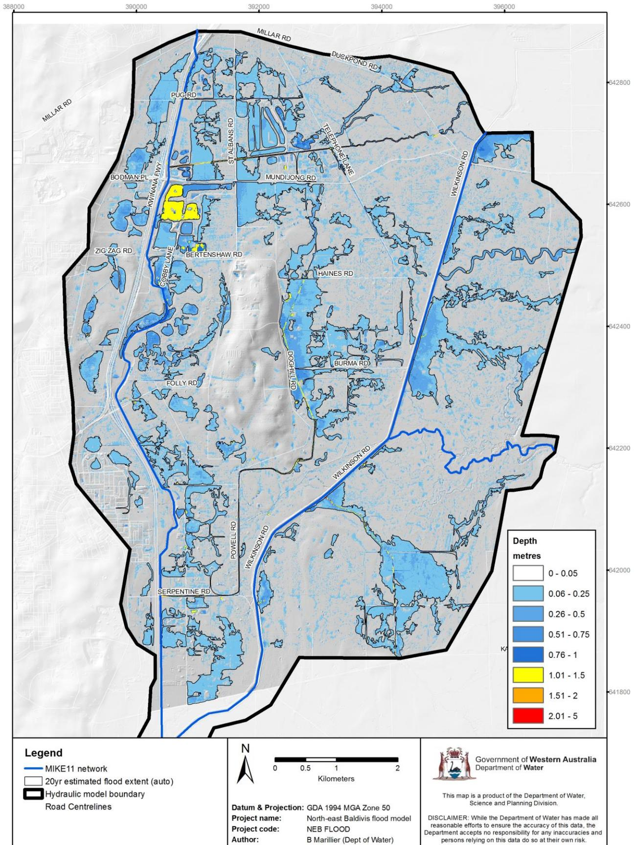
Figure D-3: 20 yr maximum flood levels, refer to long-sections for levels in drains
