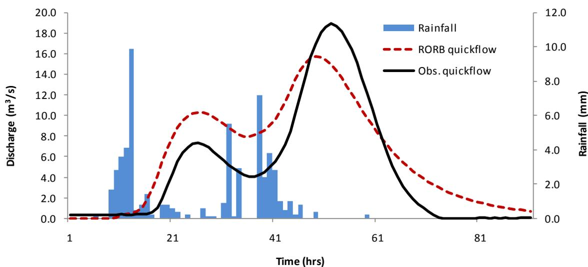
Figure B-14: RORB modelled and observed flows for Serpentine River (August 2005)
