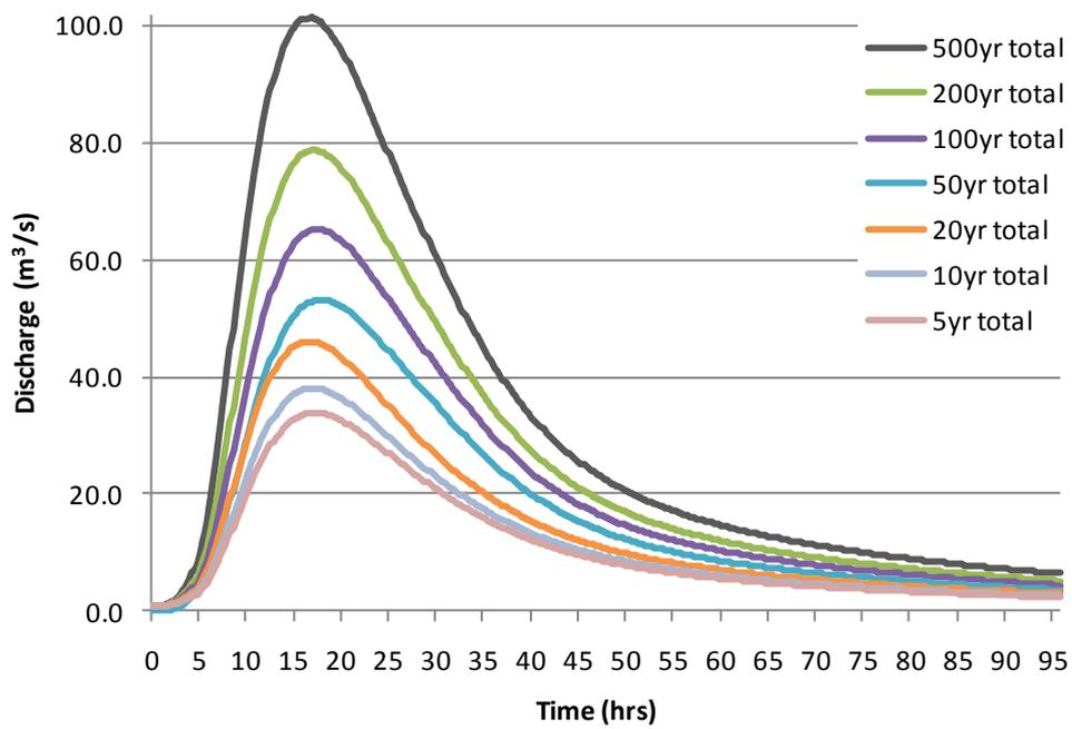
Figure 4-10: Serpentine RORB design flows at Lowlands for the 24 hr duration for various ARIs
