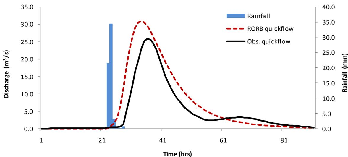
Figure B-13: RORB modelled and observed flows for the Serpentine River (August 2002)
