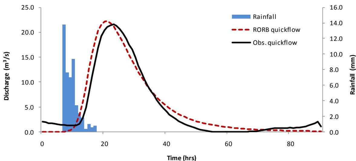
Figure B-12: RORB modelled and observed flows for Serpentine River (July 2000)
