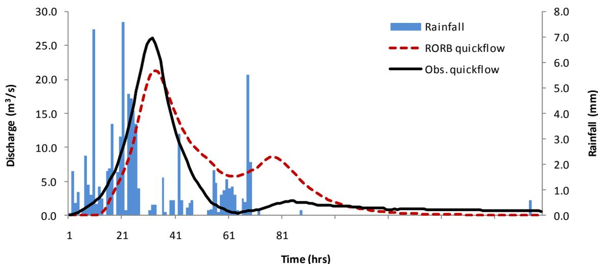
Figure B-15: RORB modelled and observed flows for the Serpentine River (July 2007)
