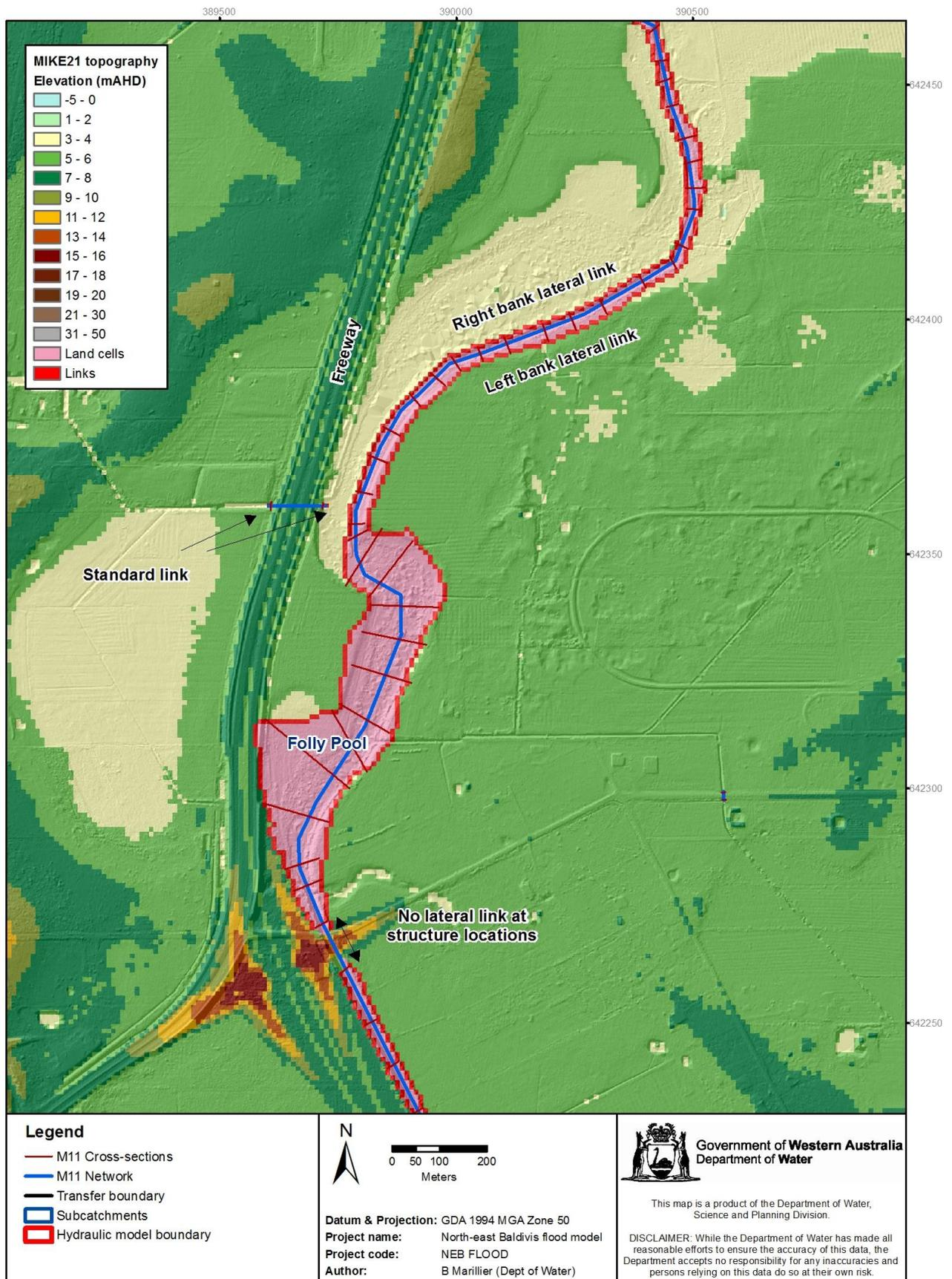
Figure 5-7: Example of lateral and standard links for a section of Peel Main Drain near Folly Pool
