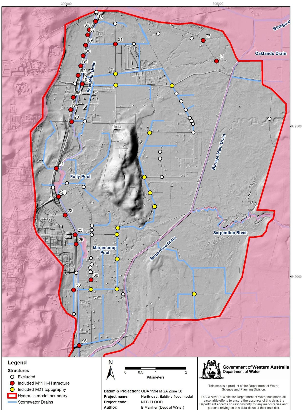
Figure 5-6: Structures included and excluded from the hydraulic model
