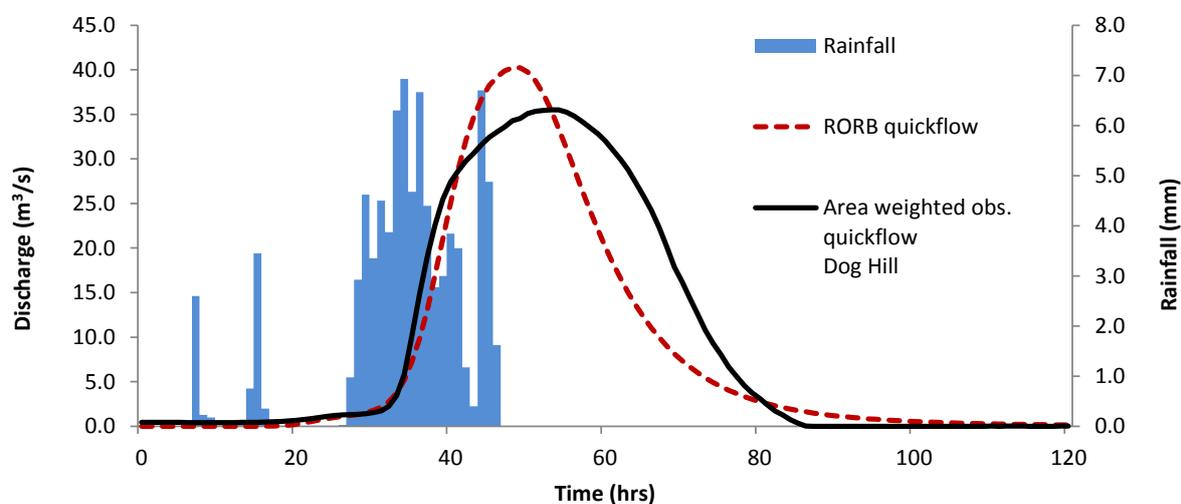
*Figure B-10: RORB modelled and area-weighted observed flows for Serpentine River, Lowlands (July 1988)*
