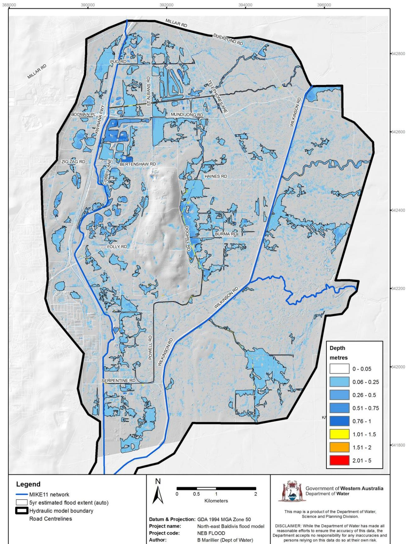
Figure D-1: 5 yr maximum flood levels, refer to long-sections for levels in drains
