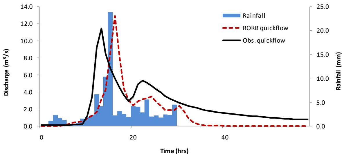
Figure B-9: RORB modelled and observed flows for Serpentine River, Mundlimup (July 1987)
