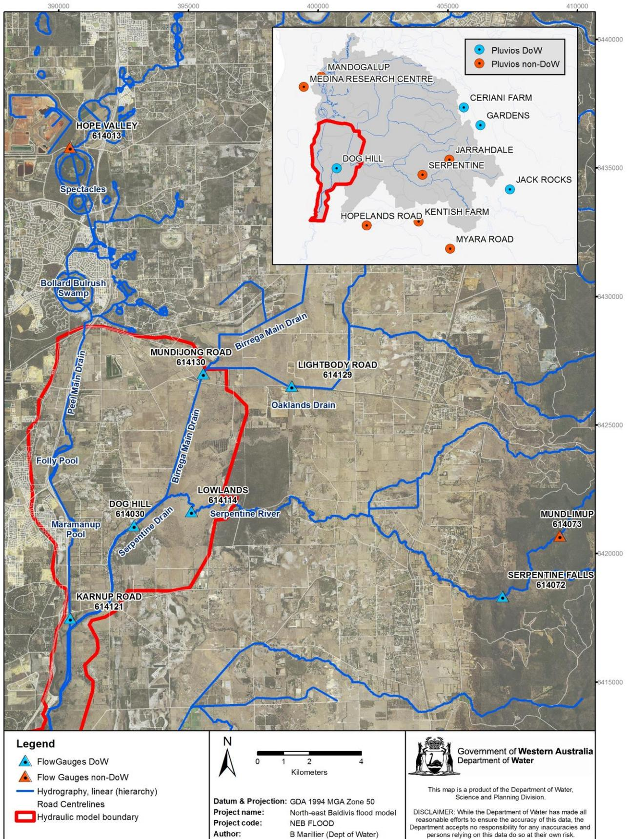
Figure 2-1: Locations of pluviographs and flow gauges used in the floodplain study
