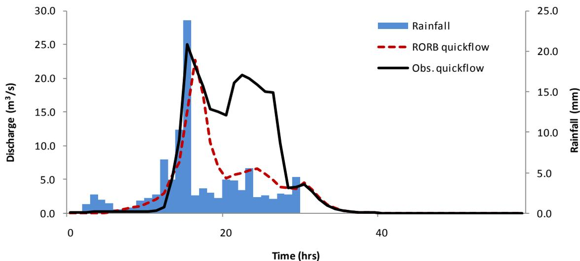
Figure B-8: RORB modelled and observed flows for Serpentine River, Serpentine Falls (July 1987)
