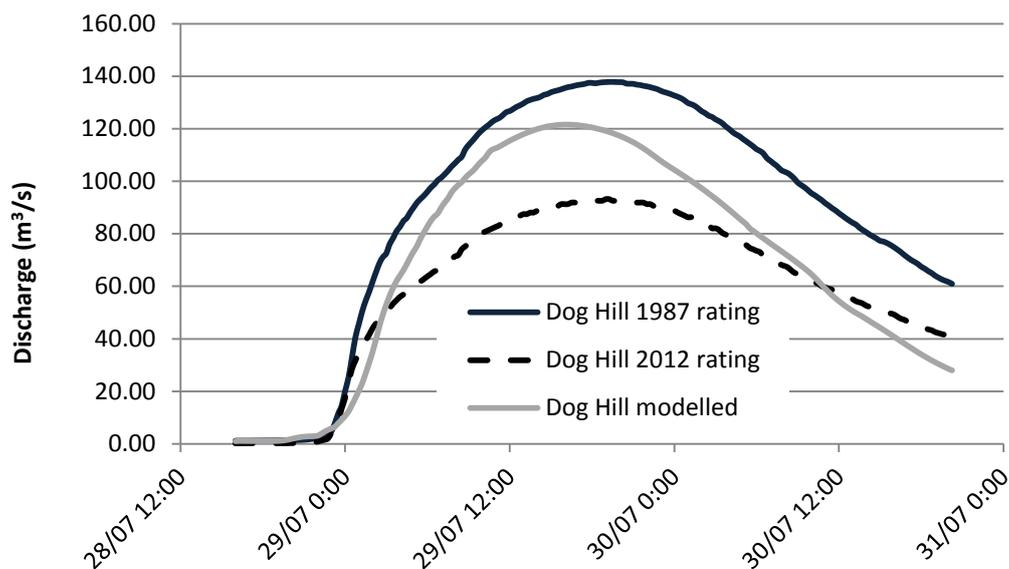
Figure 5-9: Modelled discharge and discharge estimated from the 1987 and 2010 rating curves at Dog Hill for the 1987 calibration event
