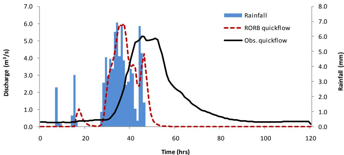
Figure B-11: RORB modelled and observed flows for Serpentine River, Mundlimup (July 1988)
