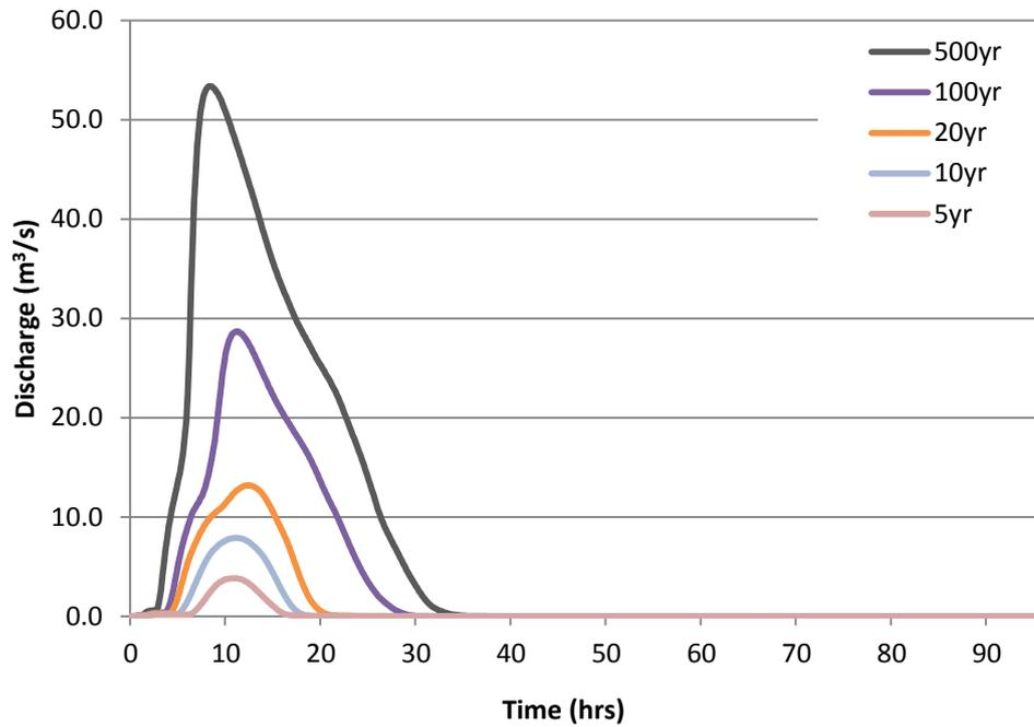
Figure 4-12: Overland flow adjacent to Oaklands Drain, sourced from the Birrega and Oaklands hydraulic model
