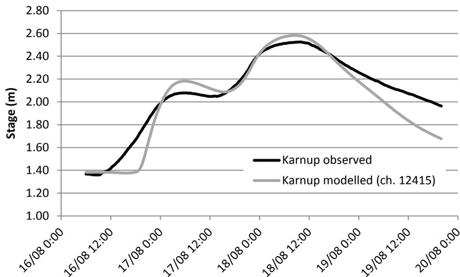
Figure 5-10: Modelled and observed stage at Karnup Road for the 2005 calibration event
