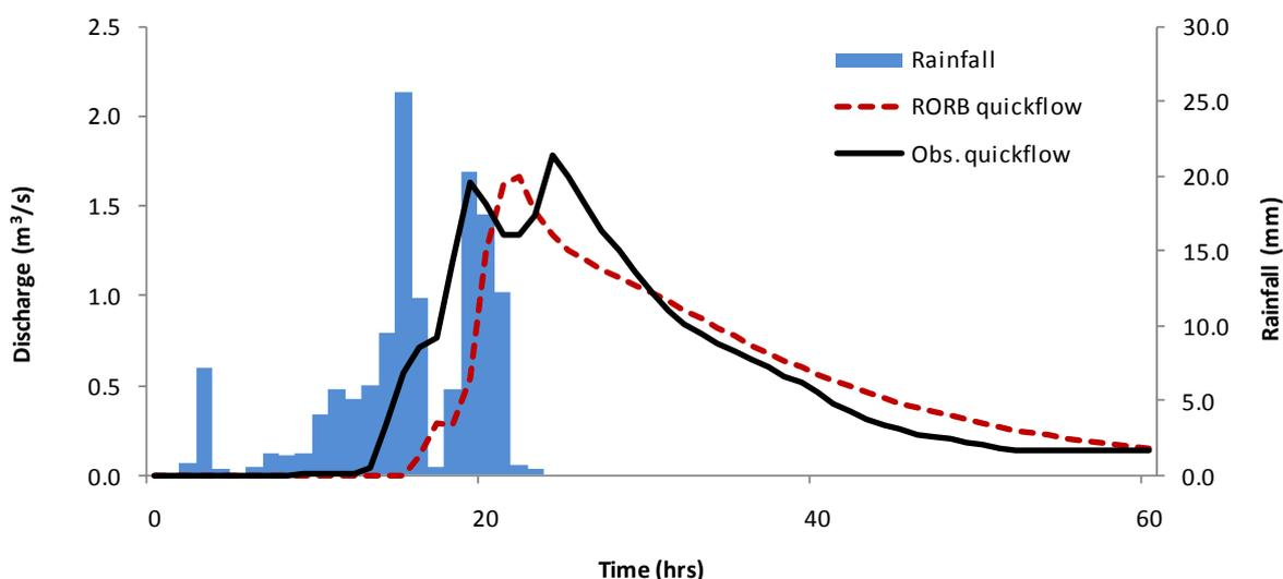
Figure B-5: RORB modelled and observed flows for the Peel Main Drain (February 1992)
