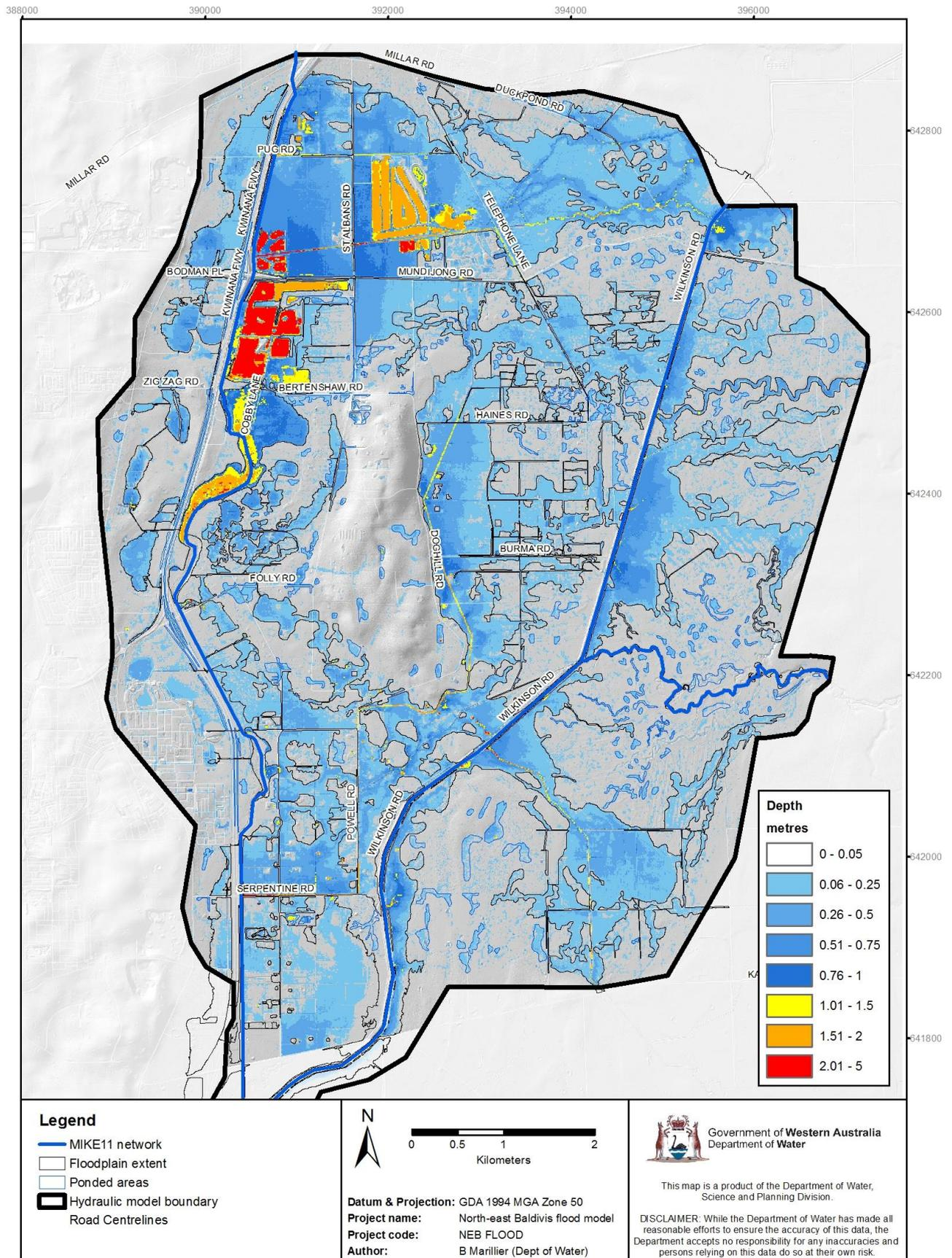
Figure D-4: 100 yr maximum flood levels, refer to long-sections for levels in drains
