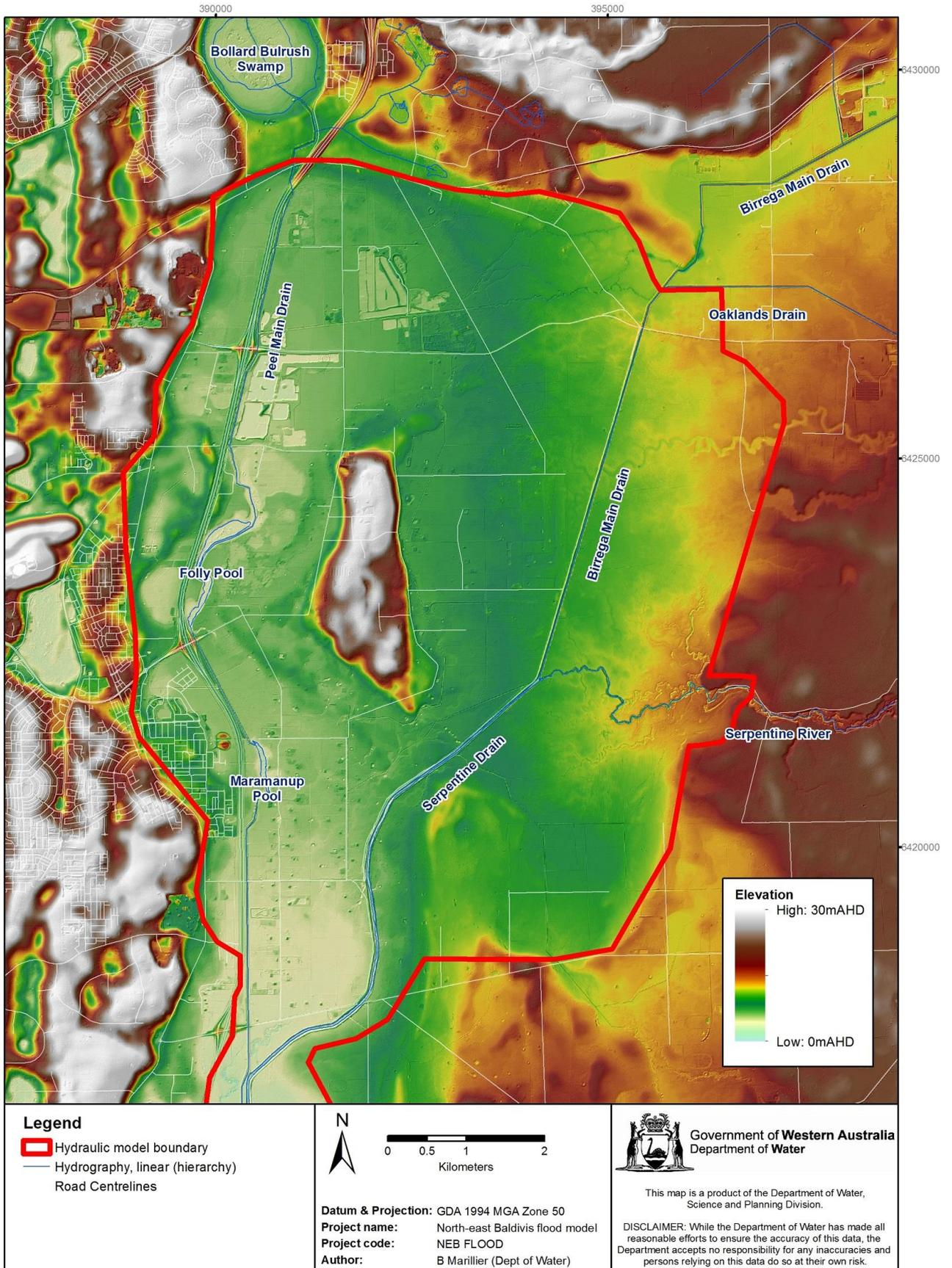
Figure 2-2: Digital elevation model (DEM) derived from LiDAR data
