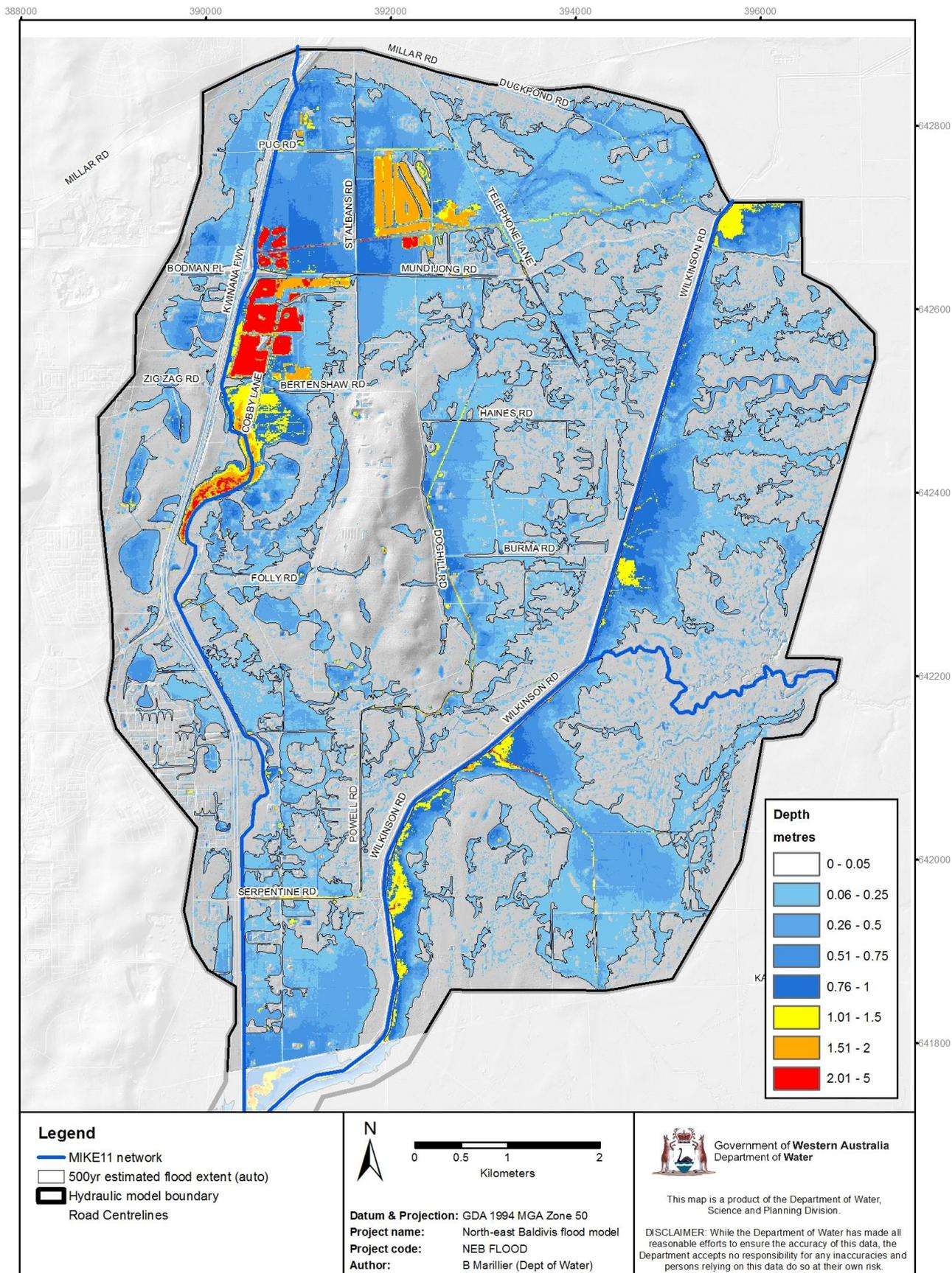
Figure D-5: 500 yr maximum flood levels
