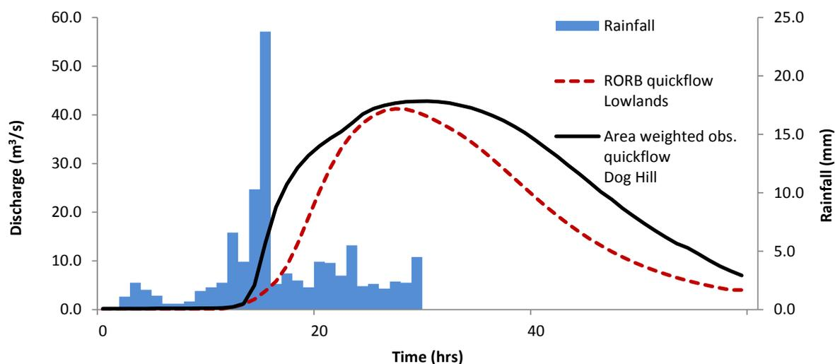
Figure B-7: RORB modelled and area-weighted observed flows for Serpentine River, Lowlands (July 1987)
