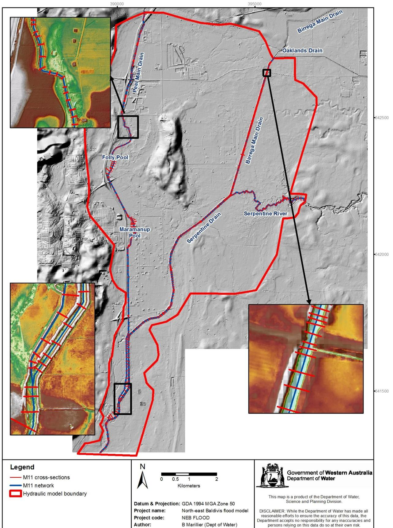
Figure 5-5: MIKE 11 channel network, cross-sections and structure locations – insets show gaps in levees, and the confluence of Serpentine and Peel Main Drains
