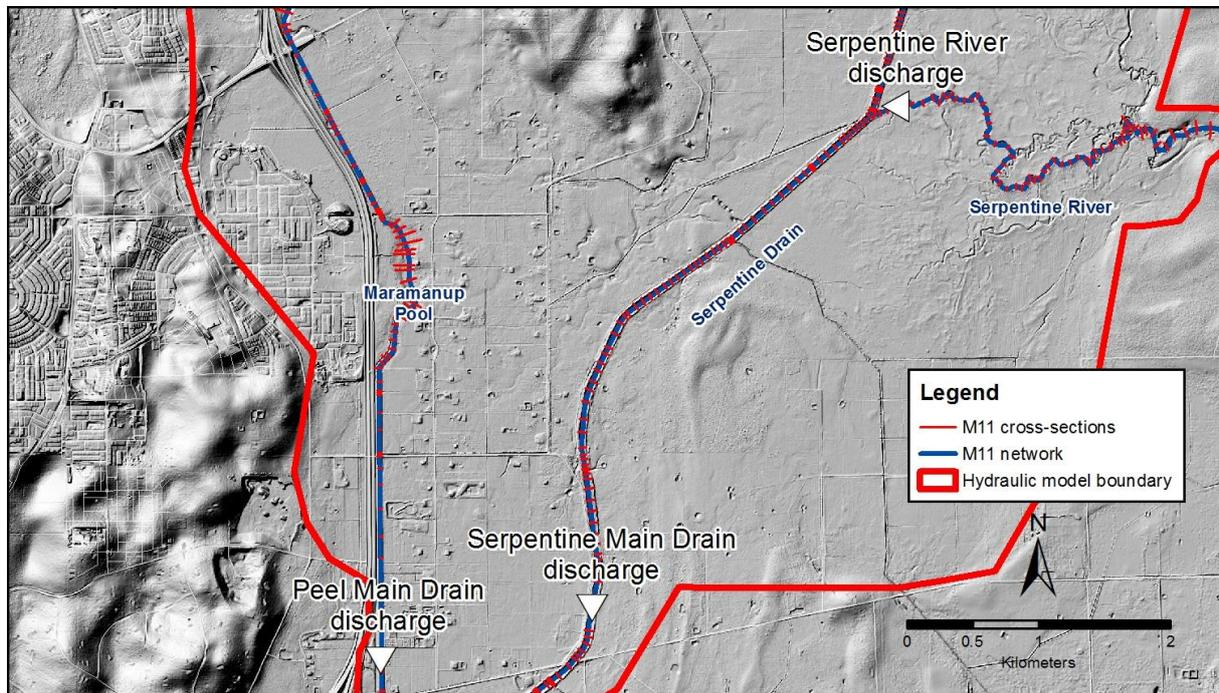
Figure F-1: Locations of discharge hydrograph extractions
