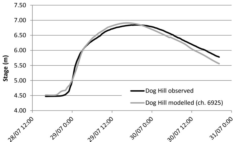
*Figure 5-8: Modelled and observed stage at Dog Hill for the 1987 calibration event*
