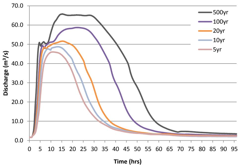
Figure 4-11: Design flows (channelised flow only) from the Birrega Main Drain, sourced from the Birrega and Oaklands hydraulic model
