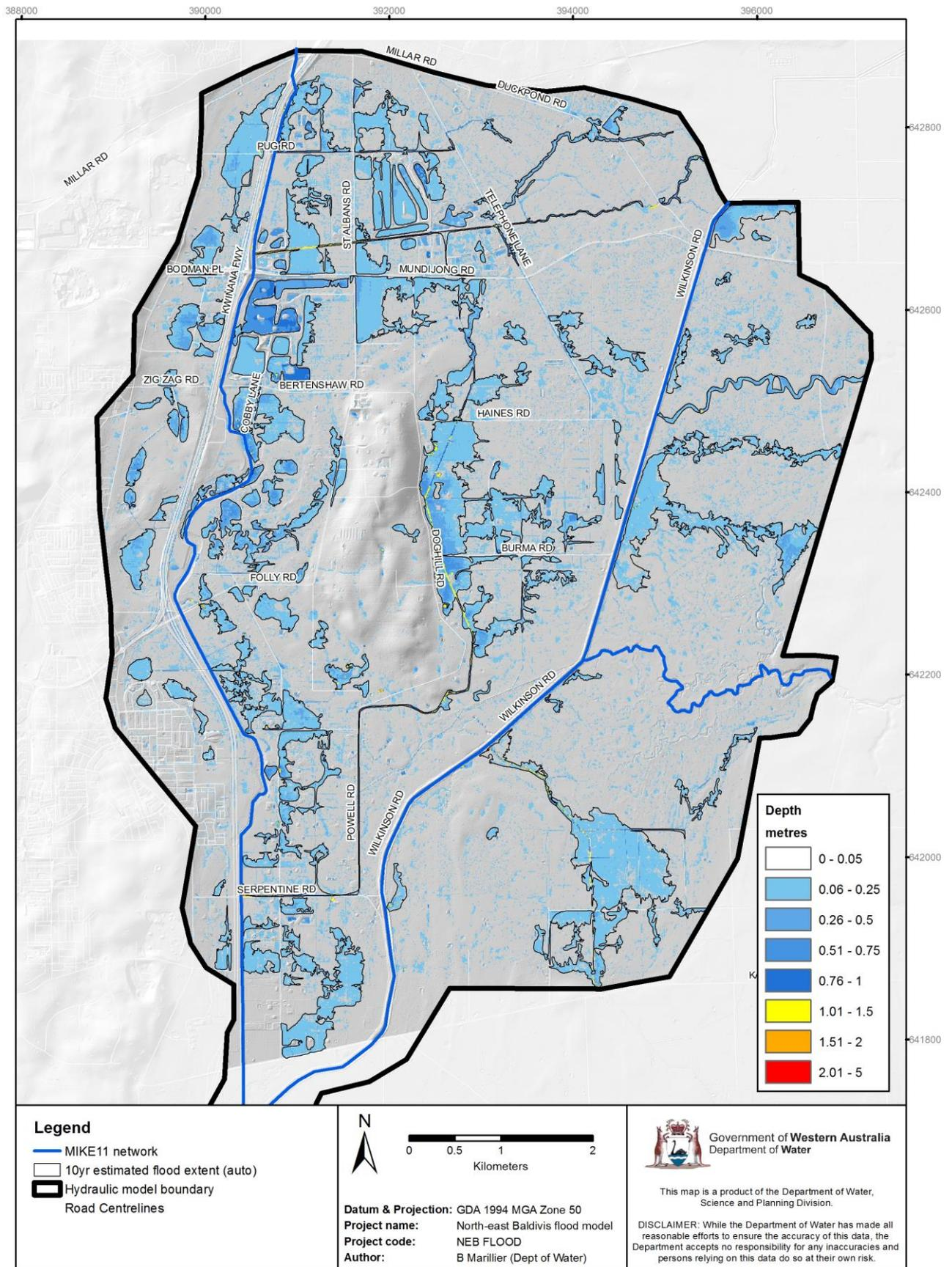
Figure D-2: 10 yr maximum flood levels, refer to long-sections for levels in drains
