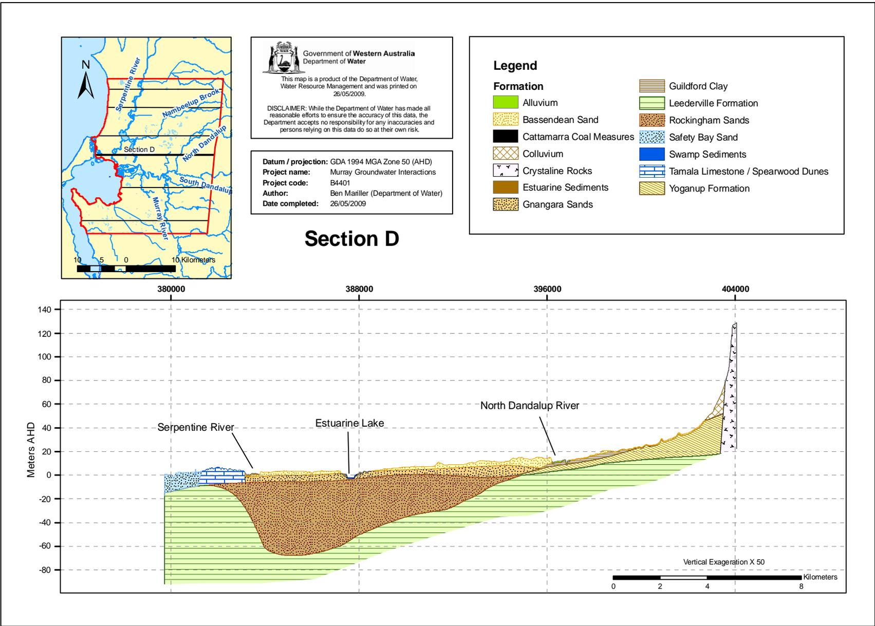
Figure 4-13: Cross section D: Superficial and Leederville Formations
