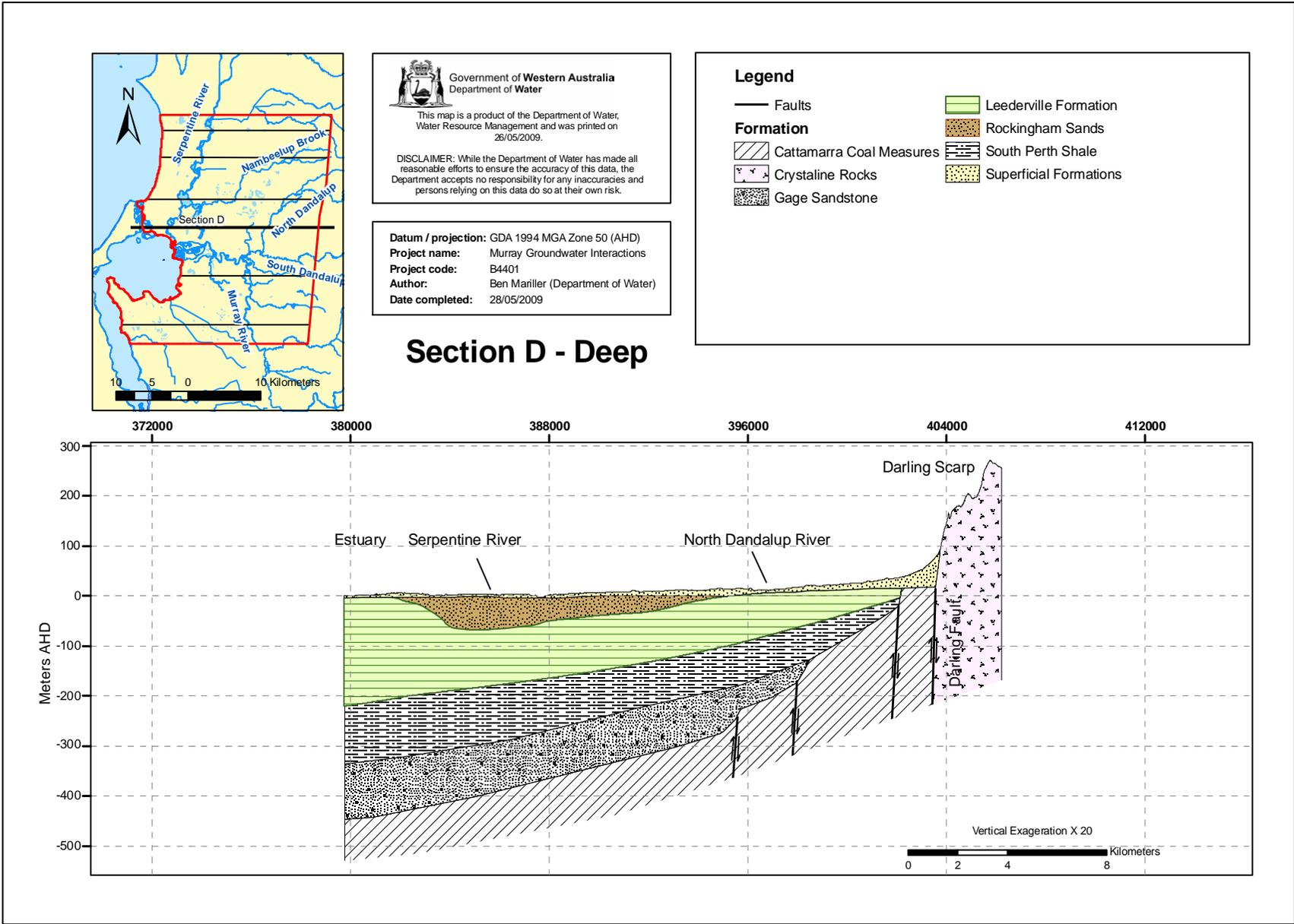
Figure 4-16: Cross section D: Deeper formations
