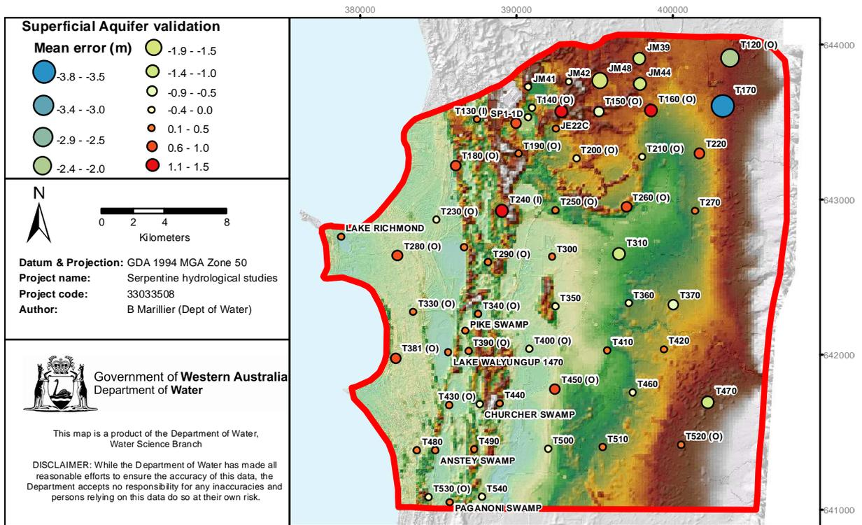
Figure 4-8 Distribution of mean error (observed minus modelled heads) for the Superficial Aquifer for the validation period
