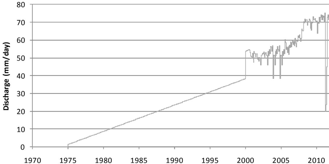
Figure 3-9 Time-series of wastewater infiltration rates near the Spectacles Wetlands
