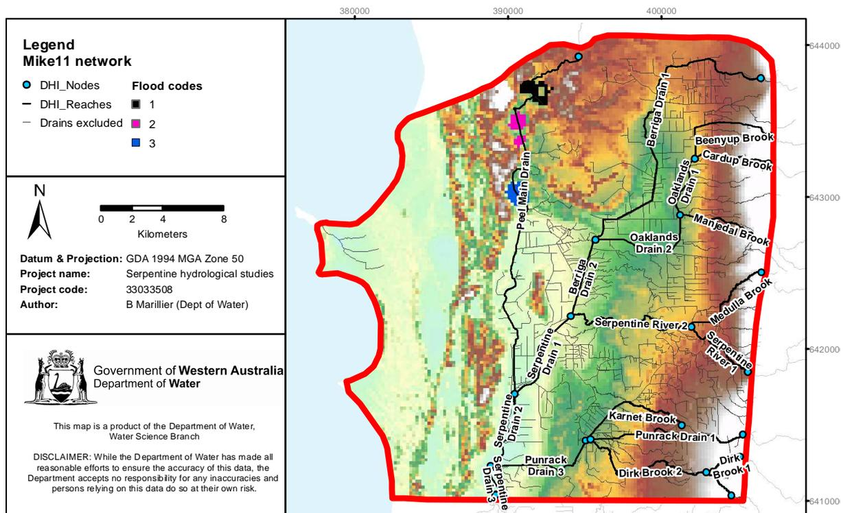
Figure 3-7 Mike 11 network: fine grey lines show drainage that was not included in the network (these drains were included in the saturated zone drainage model)
