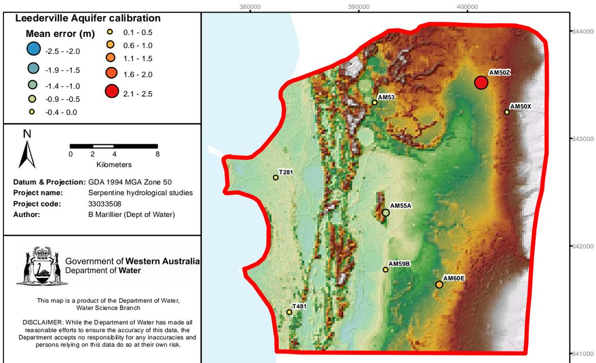
Figure 4-6 Distribution of mean error (observed minus modelled heads) for the Leederville and Rockingham aquifers for the calibration period
