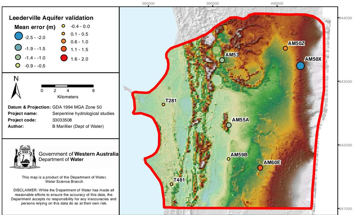
Figure 4-10 Distribution of mean error (observed minus modelled heads) for the Leederville and Rockingham aquifers for the validation period
