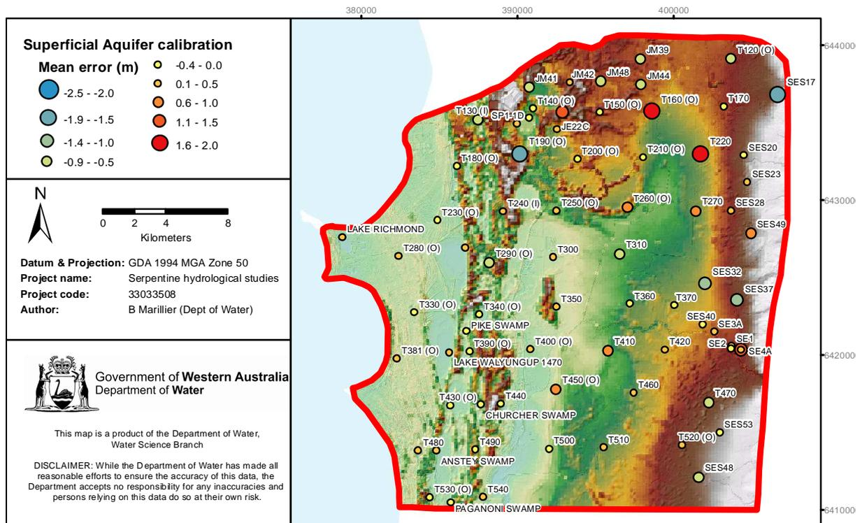
Figure 4-4 Distribution of mean error (observed minus modelled heads) for the Superficial Aquifer for the calibration period
