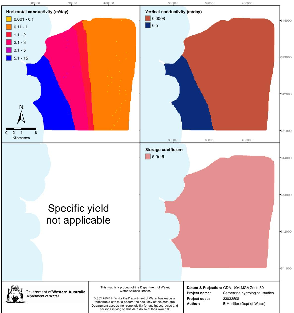
Figure 4-20 Distributed hydraulic parameters for the third computational layer ( $K_h$ ,  $K_z$ ,  $S_c$ )
