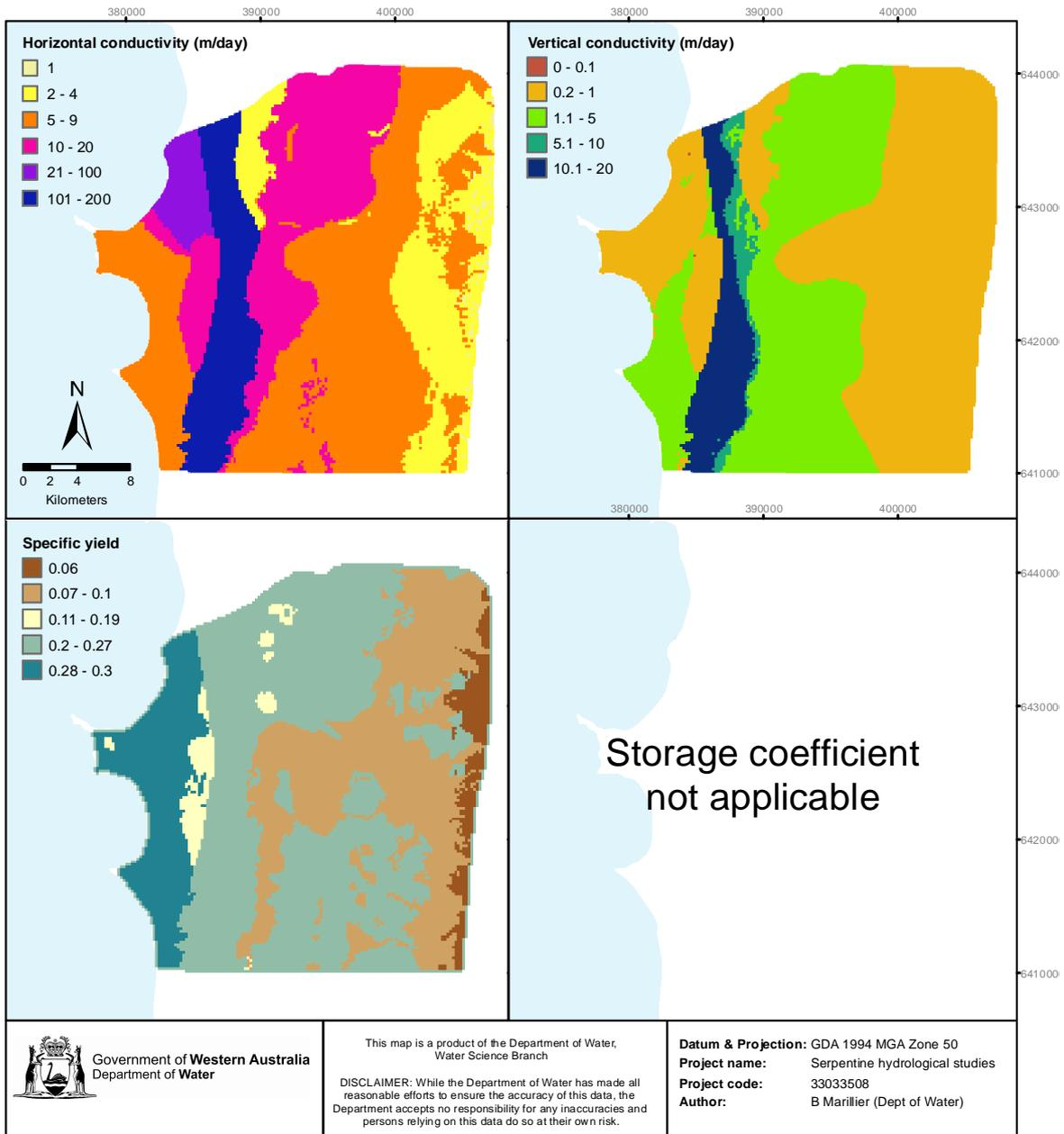
Figure 4-18 Distributed hydraulic parameters for the first computational layer ( $K_h$ ,  $K_z$ ,  $S_y$ )
