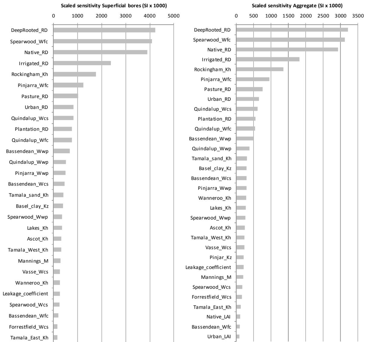
Figure 6-1 Sensitivity coefficients for the Superficial Aquifer and aggregate function objective functions
