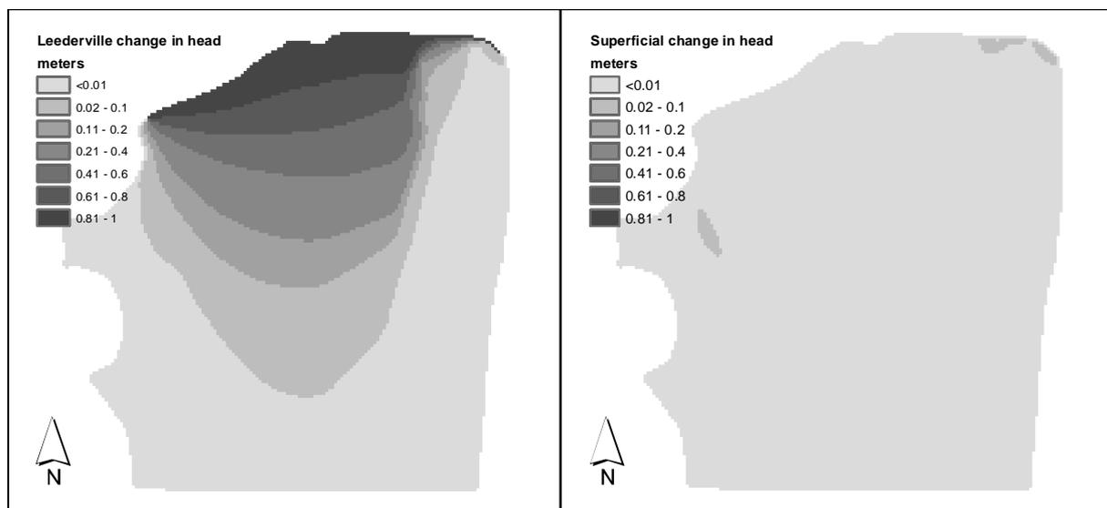
Figure 6-14 Sensitivity of head to Leederville boundary conditions in the first and third computational layers
