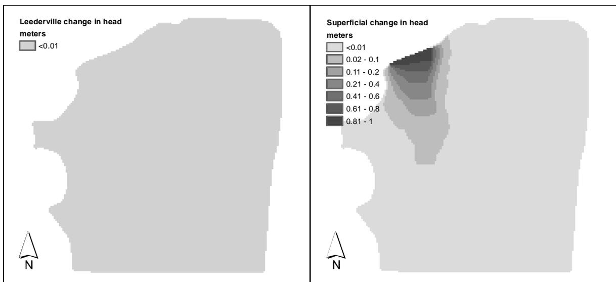
Figure 6-12 Sensitivity of head to Superficial boundary conditions in the first and third computational layers
