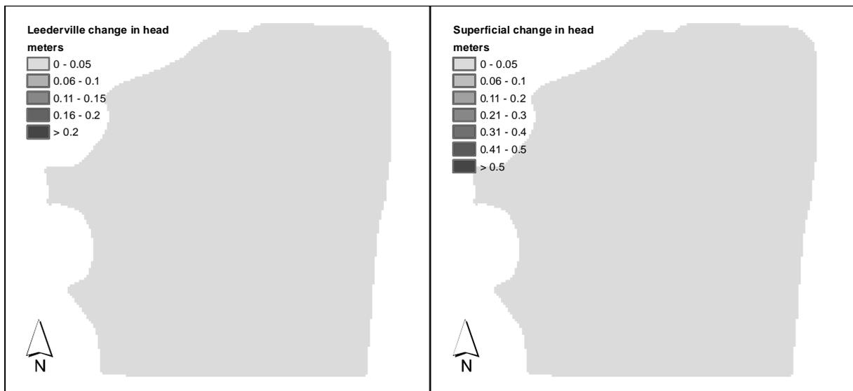
Figure 6-8 Sensitivity of head to river flows in the first and third computational layers
