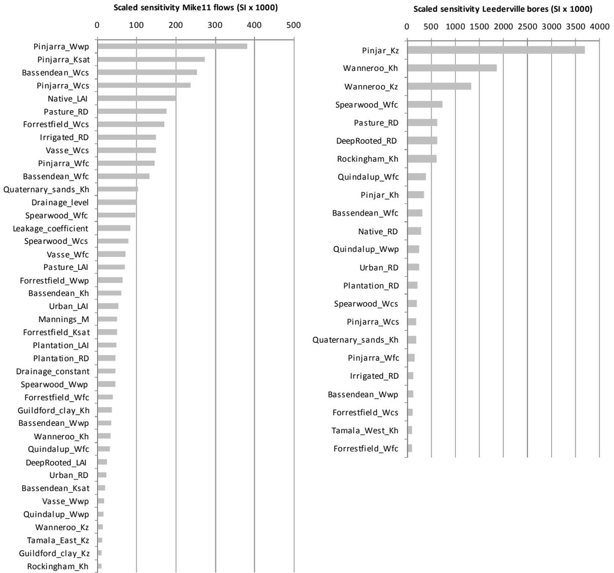
Figure 6-2 Scaled sensitivity values for the Mike11 and Leederville Aquifer objective functions
