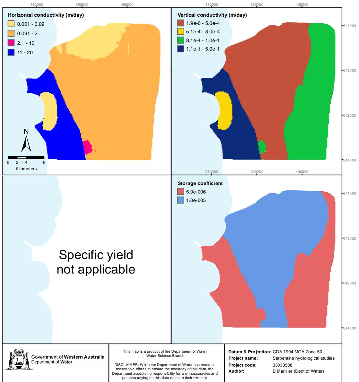
Figure 4-19 Distributed hydraulic parameters for the second computational layer ( $K_h$ ,  $K_z$ ,  $S_c$ )
