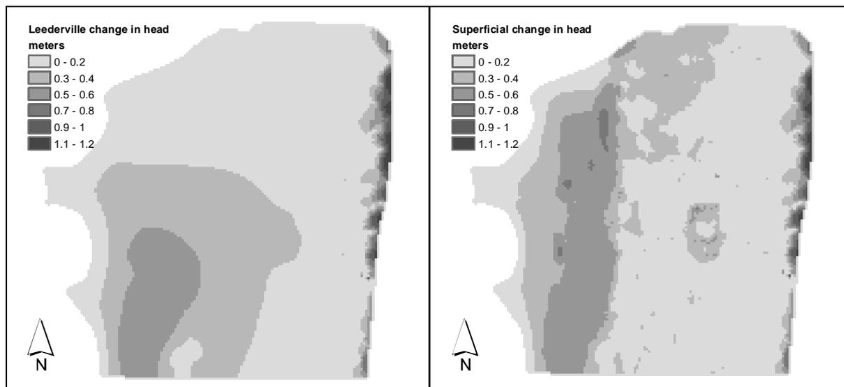
Figure 6-6 Sensitivity of head to  $ET_0$  in the first and section computational layers
