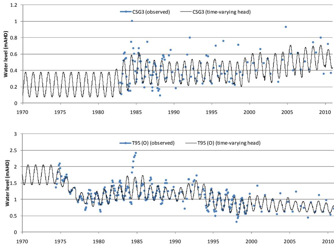
Figure 3-28 Time-varying specified heads for the north-western and north boundaries in the first computational layer
