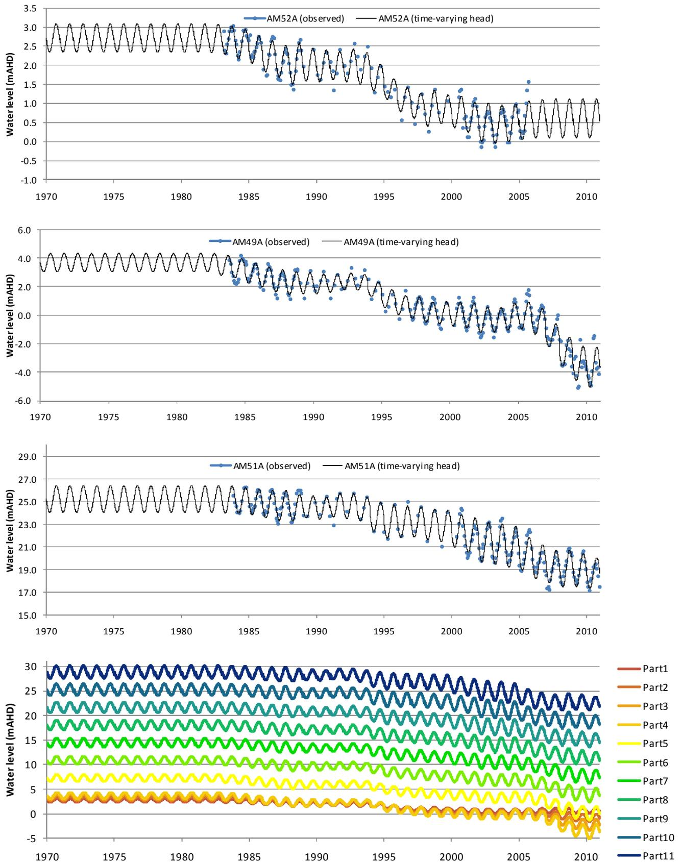
Figure 3-29 Time-varying specified heads for the northern boundary for the second and third computational layer
