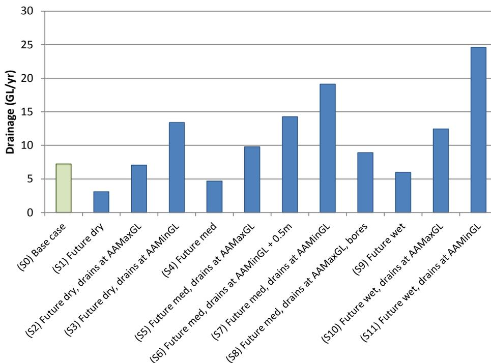
Figure 3-4 Total drainage quantity from developments for various development, drainage and climate scenarios
