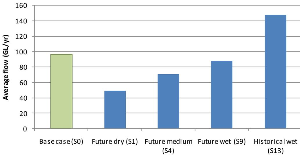
Figure 3-12 Average annual flows for the climate scenarios, based on modelled discharge from the Serpentine River at the model boundary
