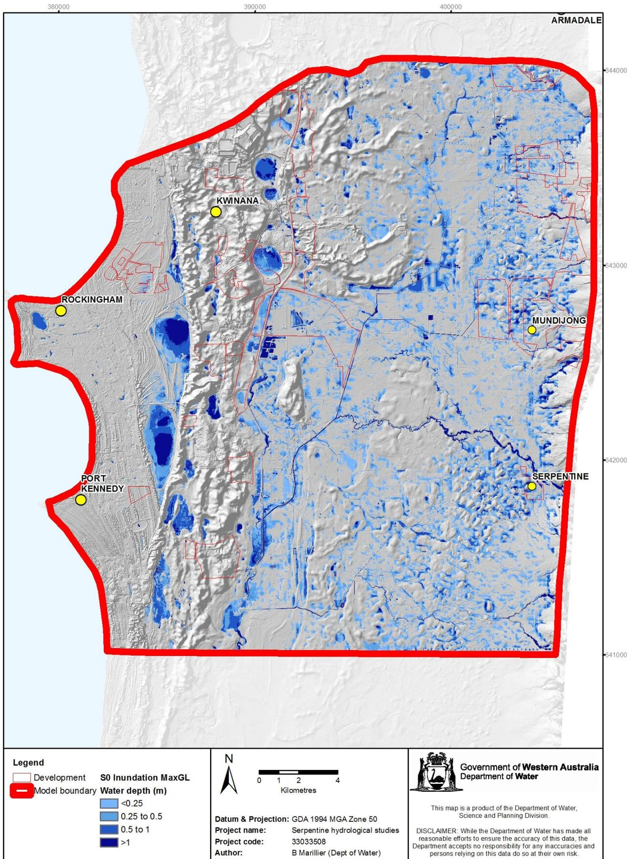
Figure 3-2 Groundwater inundation (m above surface) for the base-case (S0) scenario for 1981-2010, calculated from surface topography and MaxGL surface
