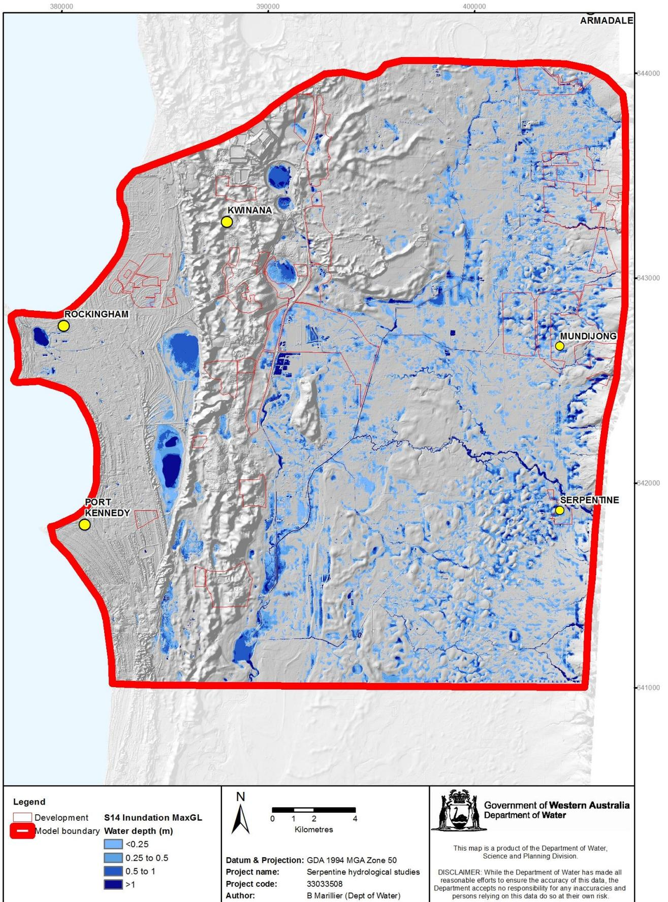
Figure B-6 Extent of inundation at MaxGL with sea-level-rise and medium climate (S14)
