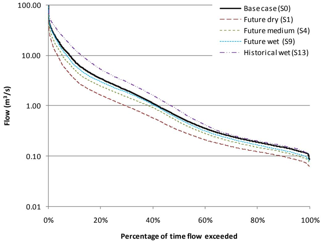
Figure 3-11 Flow duration curves for climate scenarios, based on modelled discharge from the Serpentine River at the model boundary
