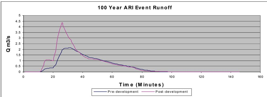
Diagram 2 Typical pre- and post-development runoff hydrograph comparison
