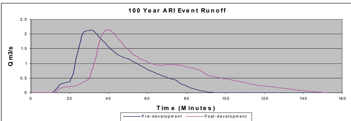
Diagram 3 Typical pre- and post-development runoff hydrograph comparison, with compensated post-development flows
