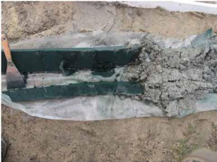
*Figure A.7 Core from HS097 before being placed in the core tray. Note the abrupt transition from the Rockingham Sand to the green-clay marker bed at 67.5 mbgl. Photo courtesy Claire Johnsen, GHD*
