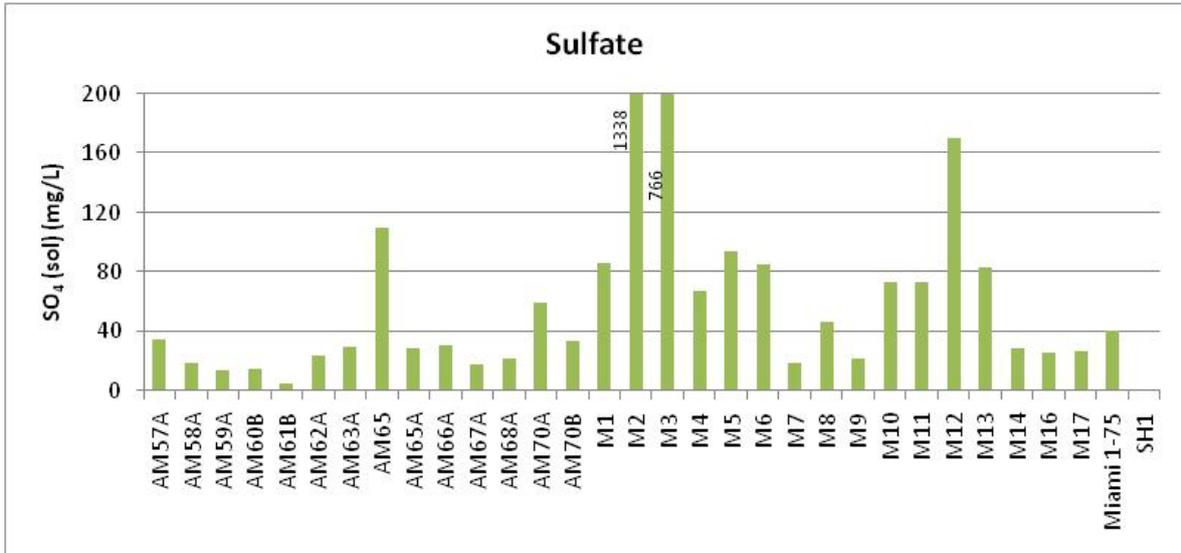
Chart B.7 Sulfate concentrations in groundwater within the Leederville Aquifer.
