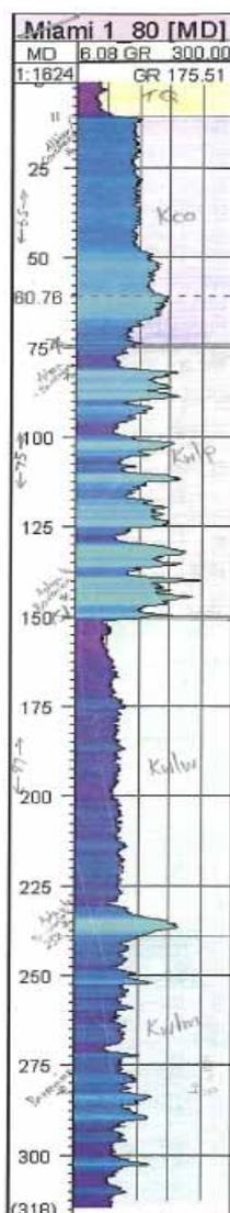
Figure A.2 Miami 1-80 gamma log. An example of how stratigraphic picks were completed manually based on gamma, resistivity logs, lithology logs and palaeontology reports where available.
