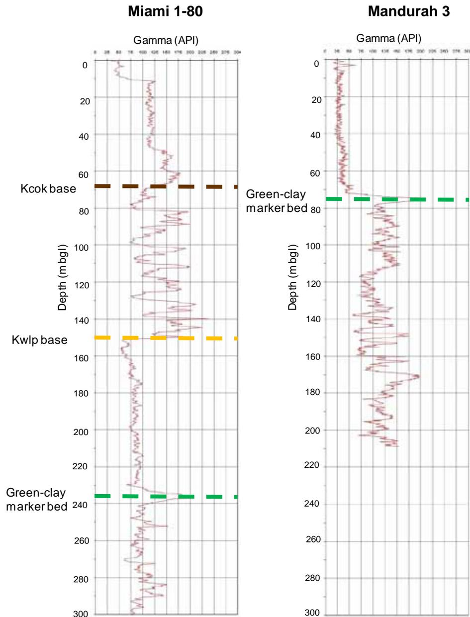
Figure A.10 Gamma and resistivity logs for Miami 1-80 and Mandurah 3 bores
