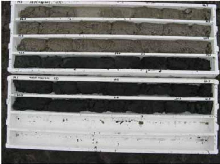
*Figure A.6 Core from bore HS104-1 between 55.5 m bgl and 61.5 m bgl, illustrating the change from the Rockingham Sand to the green-clay marker bed at 58.5 m bgl (the photo was taken late in the day, described as 'dark copper green' in the lithology logs). Photo courtesy Claire Johnsen, GHD*
