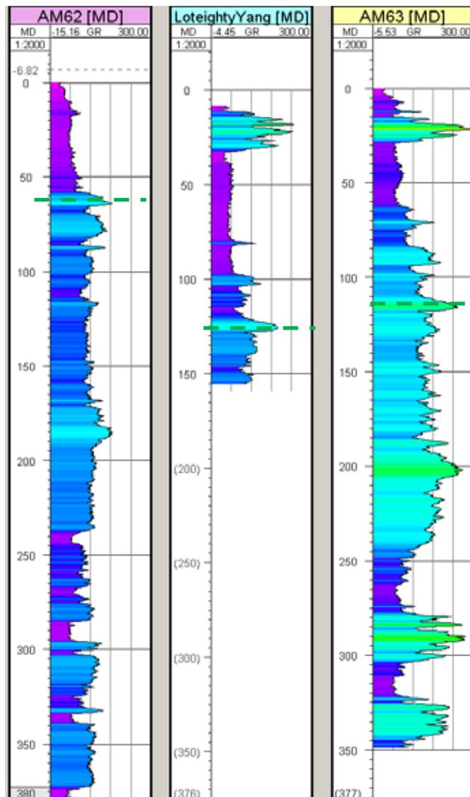
Figure A.11 Geophysical logs for AM62 (west), Yangedi Rd (centre), and AM63 (east). The Mandurah Fault is mapped between Yangedi Rd and AM62, with the formations on the east being downthrown relative to the units to the west. The green-clay marker bed is marked with the dashed green line.
