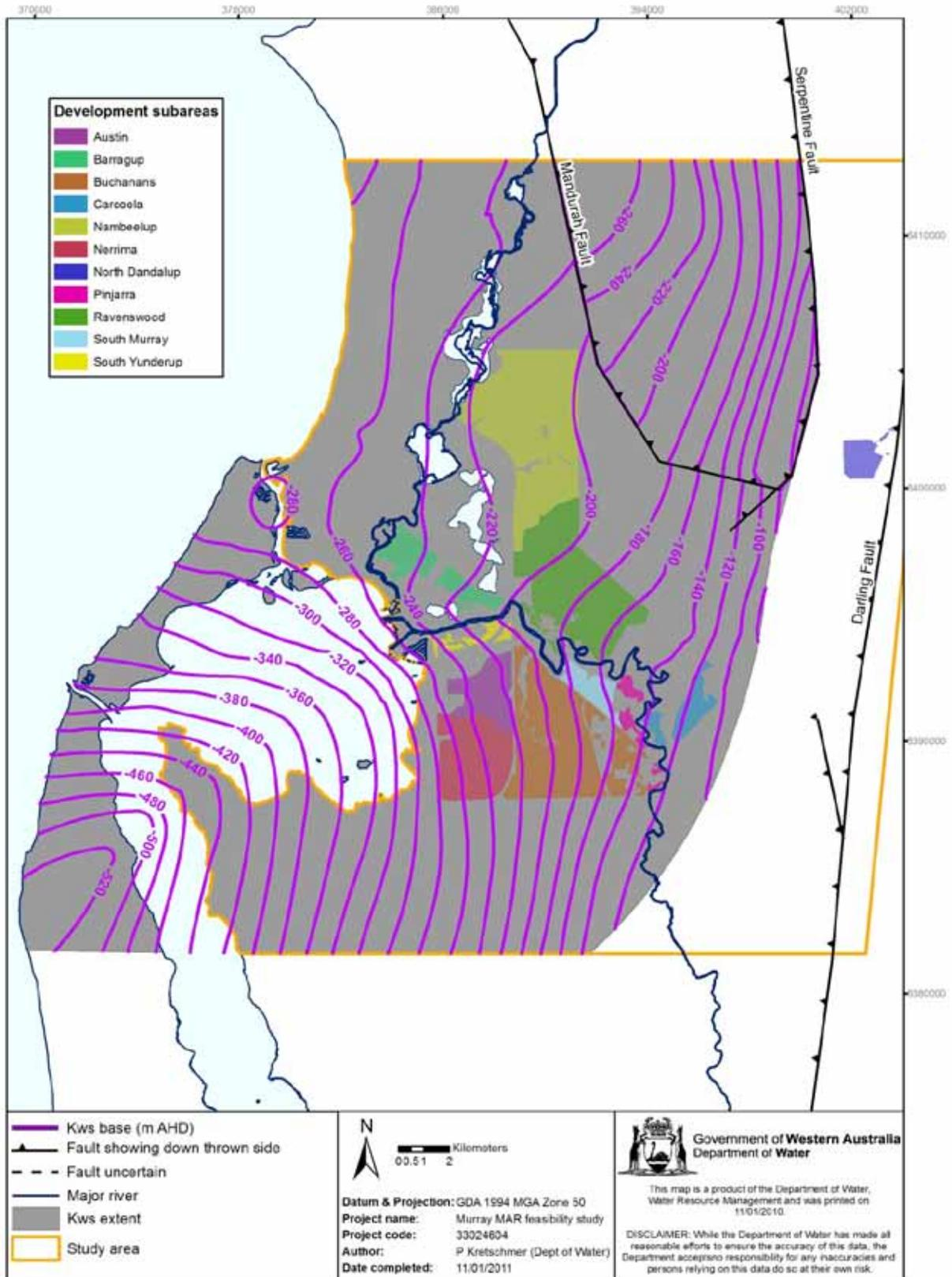
Figure A.5 Revised South Perth Shale (Kws) base contours
