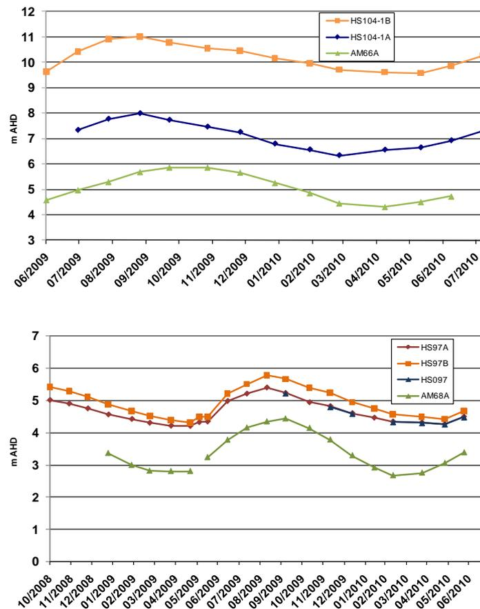
Chart 2.1 Hydrograph for the Superficial – Leederville Aquifer interaction. A) HS 104-B – Superficial Aquifer; HS104-1A – upper Leederville Aquifer; AM66A – lower Leederville Aquifer. B) HS97A; HS97B – Superficial Aquifer; HS097 – upper Leederville Aquifer; AM66A
