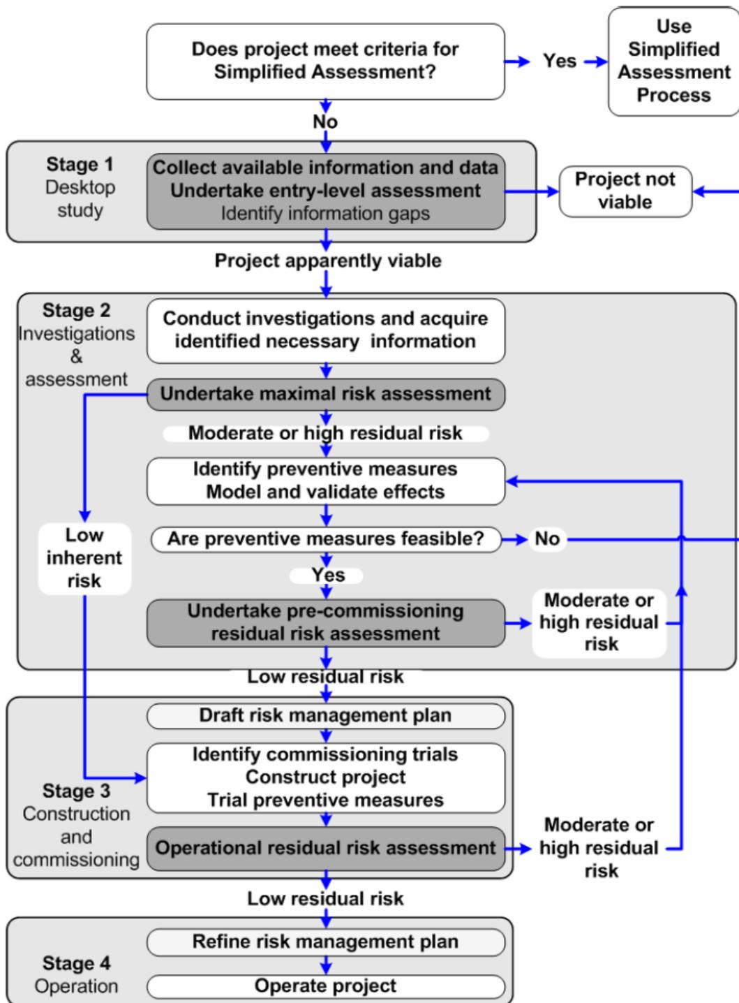
Figure 1.2 Stages of investigation for a managed aquifer recharge project (source: NRMCC 2009)
