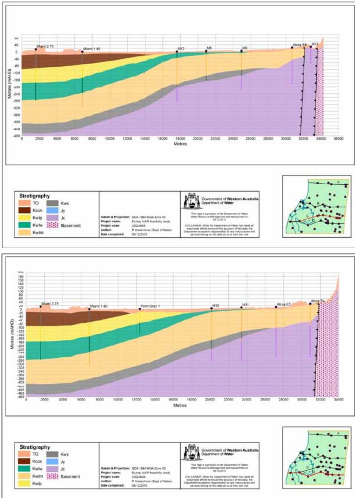
Figure 2.5 (top) and Figure 2.6 (bottom) Cross-sections of the revised geology interpretation
