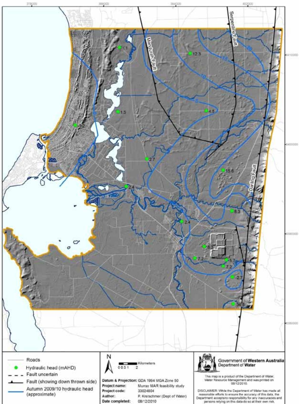
Figure 2.8 Leederville Aquifer hydraulic head contours in autumn 2009
