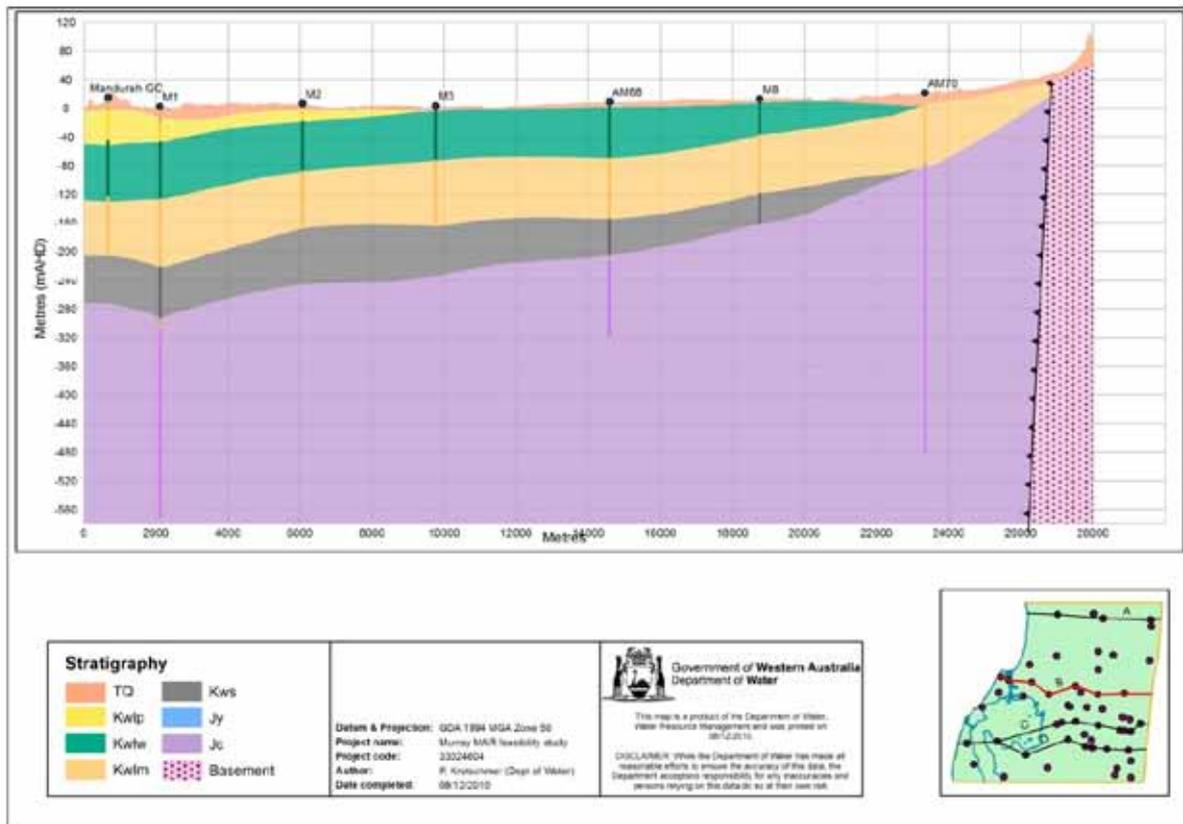
Figure 2.3 (top) and Figure 2.4 (bottom) Cross-sections of the revised geology interpretation
