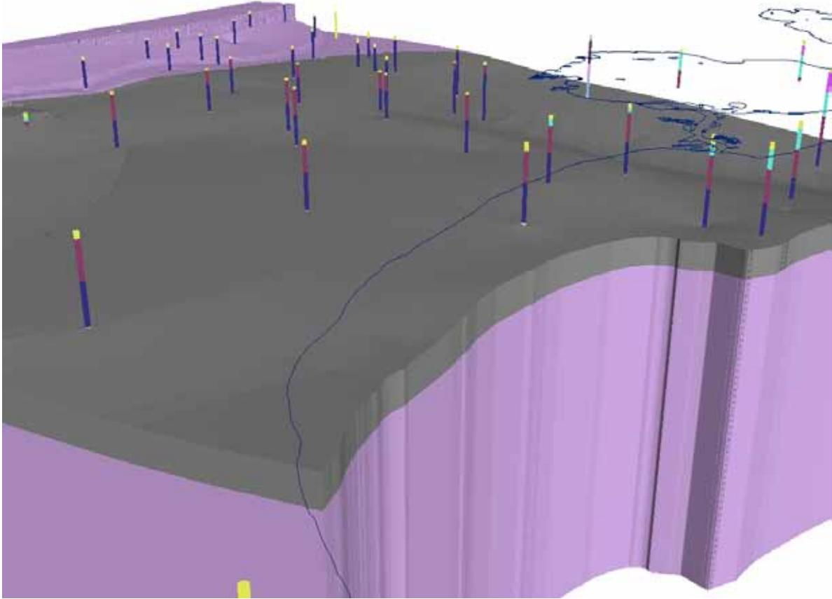
*Figure A.3 An example of the surface for the South Perth Shale (grey) fitting through the picks in the bores. The South Perth Shale is pink in the bores (just visible at the base of some bores), the Mariginiup Member is marked dark blue, and the Wanneroo Member dark red. The underlying purple-coloured unit is the Cattamarra Coal Measures.*
