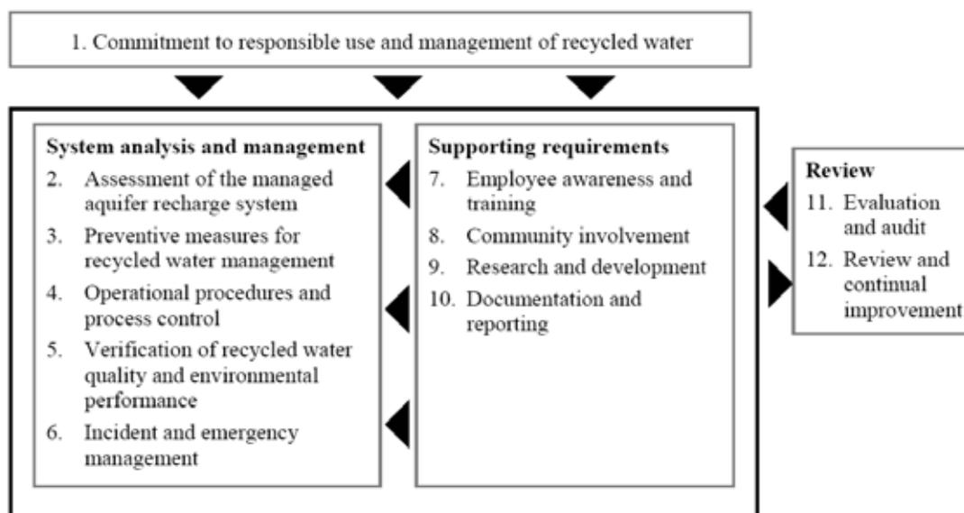
Figure 3.2 The 12 elements of the risk management plan (NRMMC-EPHC-AHMC 2006).
