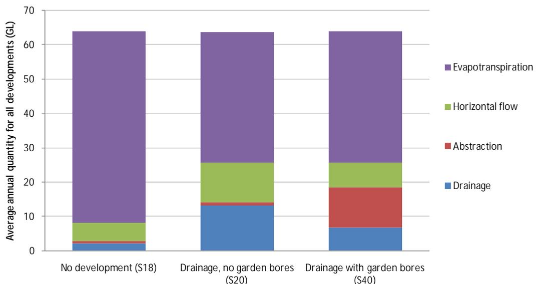
Figure 2.14 Water balance for the future medium climate scenario with no development, and development with drainage at ground level with and without garden bore extraction (source: Hall et al. 2010c)
