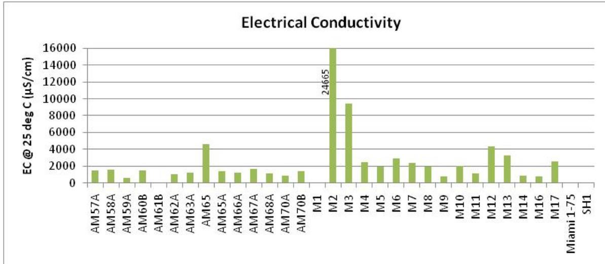
Chart B.1 Electrical conductivity values in groundwater within the Leederville Aquifer
