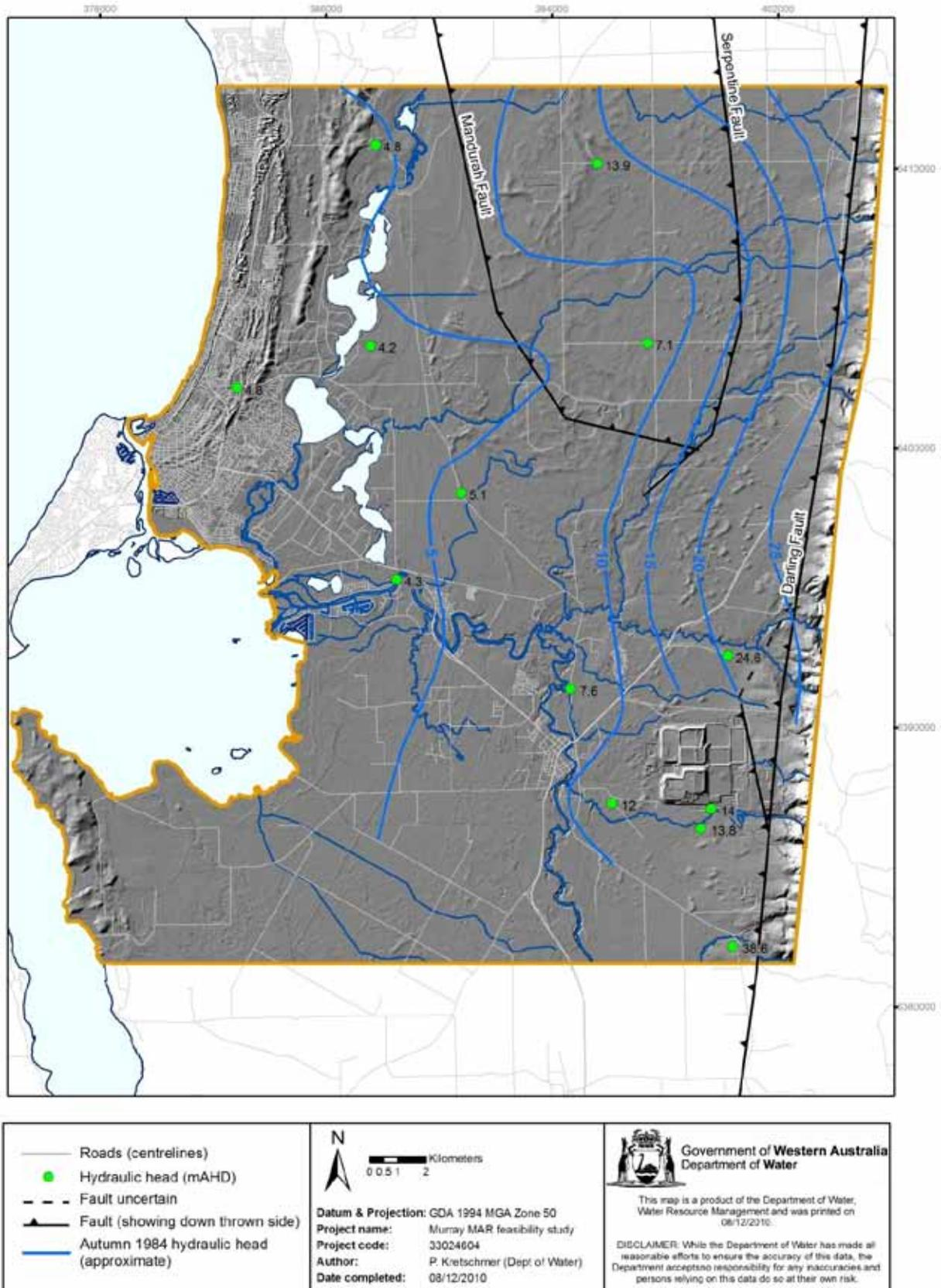
Figure 2.7 Leederville Aquifer hydraulic head contours in autumn 1984
