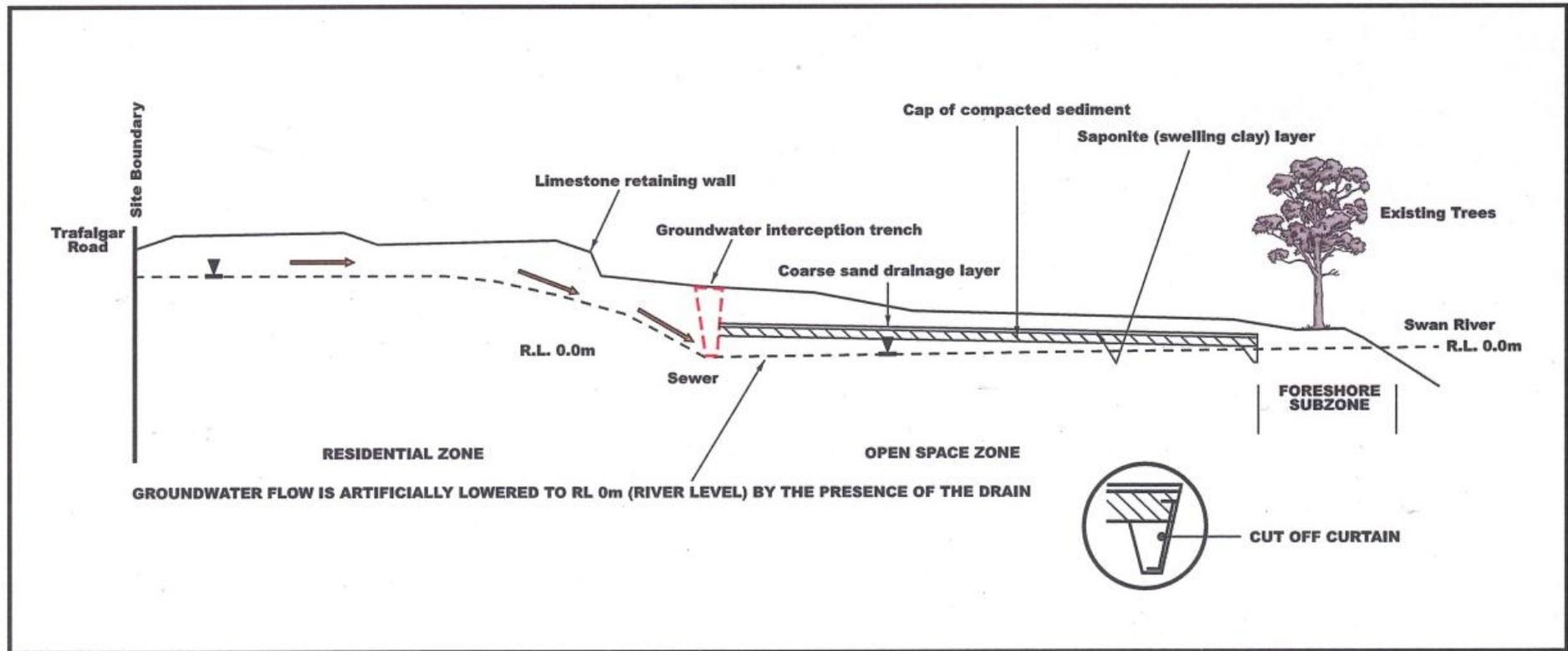
Figure 23 Schematic representation of function of containment area showing cut-off curtain, groundwater interception drain and capping layer (source: ENV 2011a).
