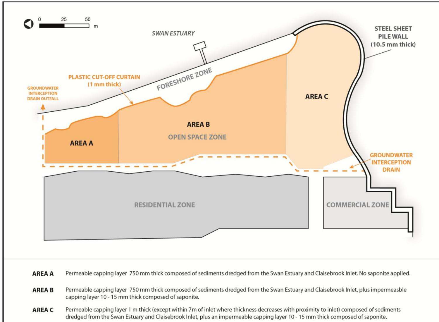
Figure 22 Capping layer composition and thickness (modified from Camp Scott Furphy 1996b).
