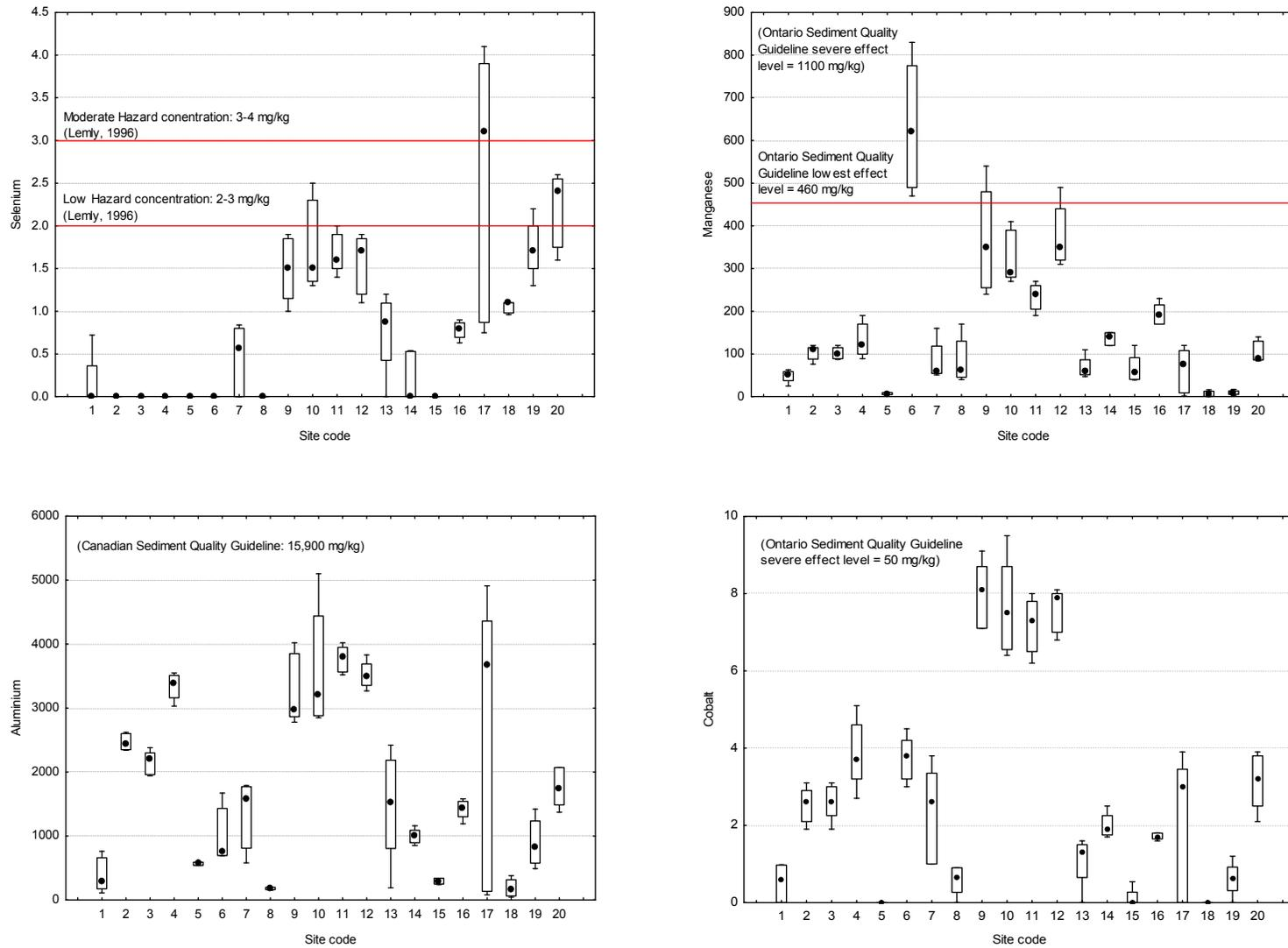
**Figure 5** Median bioavailable selenium, manganese, aluminium and cobalt concentrations (mg/kg dry weight) in sediments at 20 sites within the Swan Canning system. Sites 1-16: Swan sites; Sites 17-20: Canning sites. Bars indicate data range; box indicates 20th - 80th percentile range. ANZECC ISQGs do not currently exist for selenium, manganese, aluminium, and cobalt. Alternative guidelines have been provided.
