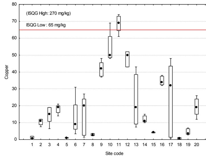
**Figure 3** Median bioavailable zinc, mercury, lead and copper concentrations (mg/kg dry weight) in sediments at 20 sites within the Swan Canning system. Sites 1-16: Swan sites; Sites 17-20: Canning sites. Bars indicate data range; box indicates 20<sup>th</sup> - 80<sup>th</sup> percentile range. ISQG Low: Trigger Value for adverse biological effects; ISQG High: adverse biological effects expected to occur more frequently.
