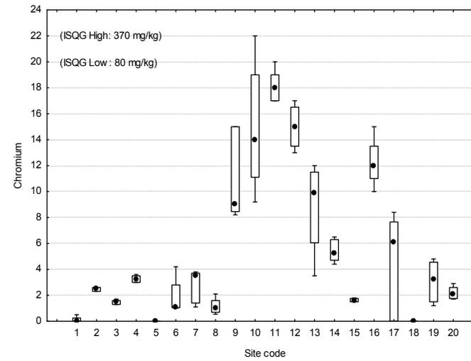
**Figure 4** Median bioavailable arsenic, cadmium, nickel and chromium concentrations (mg/kg dry weight) in sediments at 20 sites within the Swan Canning system. Sites 1-16: Swan sites; Sites 17-20: Canning sites. Bars indicate data range; box indicates 20th - 80th percentile range. ISQG Low: Trigger Value for adverse biological effects; ISQG High: adverse biological effects expected to occur more frequently.
