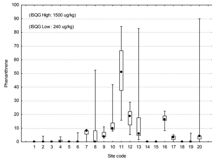
**Figure 8** Median Low Molecular Weight PAH concentrations cont'd ( $\mu\text{g}/\text{kg}$  dry weight normalised to 1% organic carbon) in sediments at 20 sites within the Swan Canning system. Sites 1-16: Swan sites; Sites 17-20: Canning sites. Bars indicate data range; box indicates 40th - 60th percentile range. ISQG Low: Trigger Value for adverse biological effects; ISQG High: adverse biological effects expected to occur more frequently.
