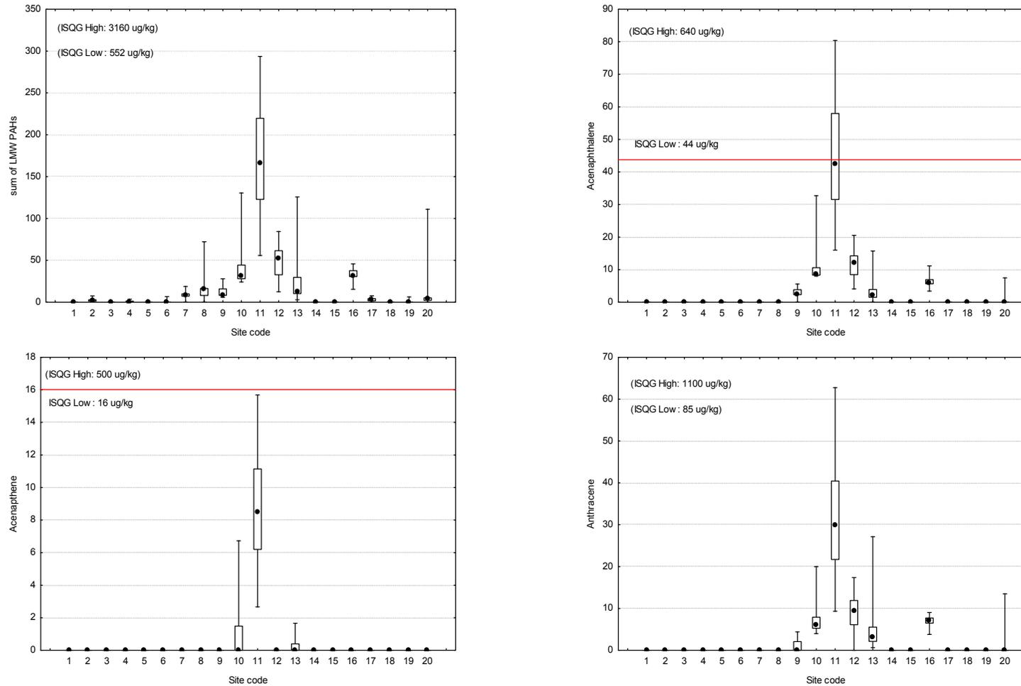
**Figure 7** Median Low Molecular Weight PAH concentrations ( $\mu\text{g}/\text{kg}$  dry weight normalised to 1% organic carbon) in sediments at 20 sites within the Swan Canning system. Sites 1-16: Swan sites; Sites 17-20: Canning sites. Bars indicate data range; box indicates 40th - 60th percentile range. ISQG Low: Trigger Value for adverse biological effects; ISQG High: adverse biological effects expected to occur more frequently.
