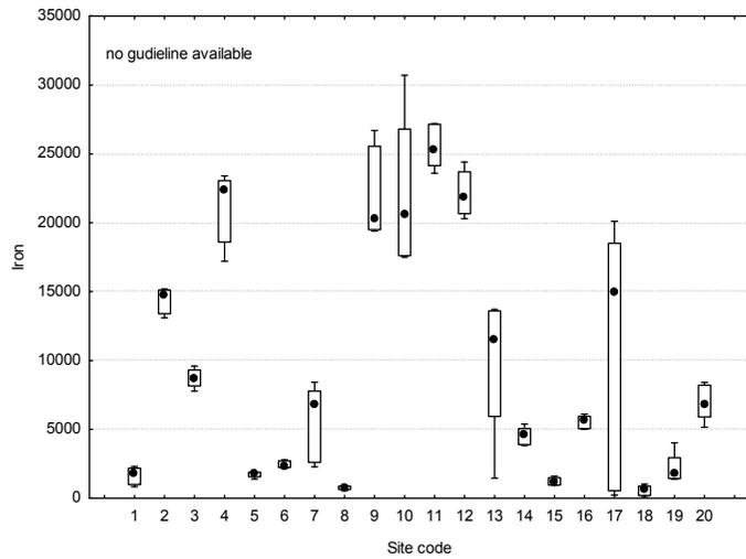
**Figure 6** Median bioavailable iron concentrations (mg/kg dry weight) in sediments at 20 sites within the Swan Canning system. Sites 1-16: Swan sites; Sites 17-20: Canning sites. Bars indicate data range; box indicates 20th - 80th percentile range. Guidelines do not currently exist for iron.
