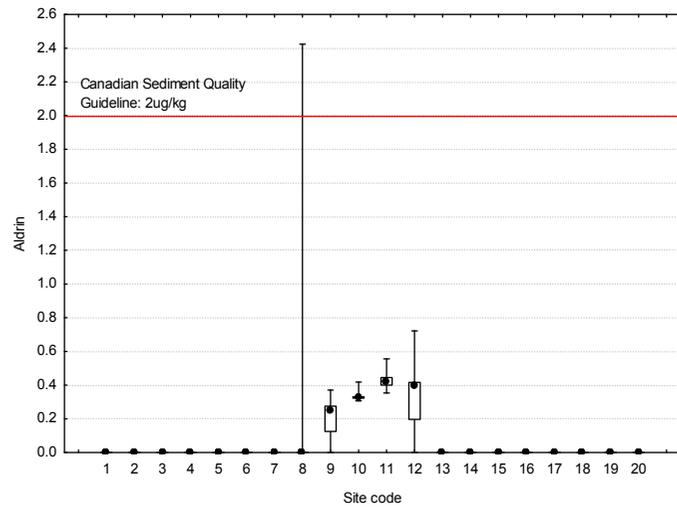
**Figure 12** Median aldrin concentration ( $\mu\text{g}/\text{kg}$  dry weight normalised to 1% organic carbon) in sediments at 20 sites within the Swan Canning system. Sites 1-16: Swan sites; Sites 17-20: Canning sites. Bars indicate data range; box indicates 40th - 60th percentile range. ANZECC ISQGs do not currently exist for aldrin. An alternative guideline has been provided.
