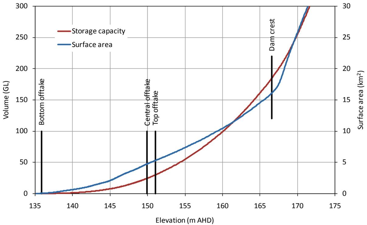
Figure 1 Wellington Reservoir surface area–elevation–storage capacity relationship
