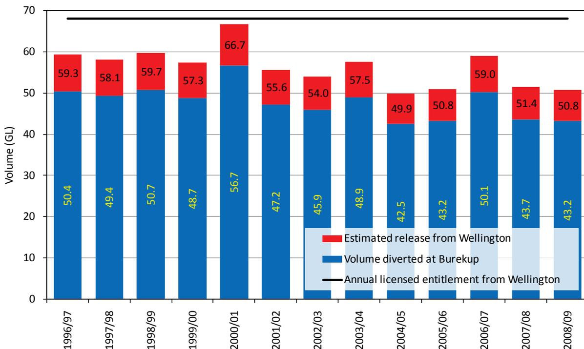
Figure 5 Annual irrigation diversion at Burekup Weir and release from Wellington Reservoir
