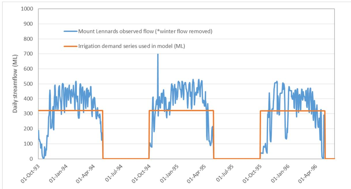
*Figure 10 Summer irrigation demand from Wellington Reservoir, modelled and observed*
