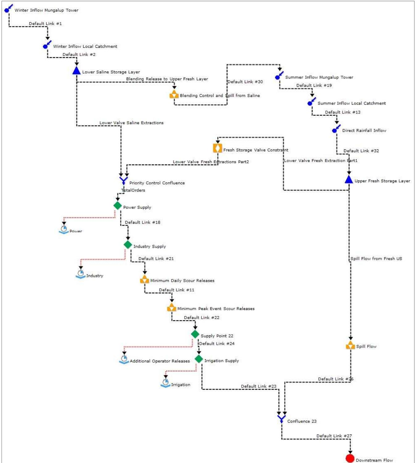
Figure 4 Wellington Reservoir schematic model in eWater Source
