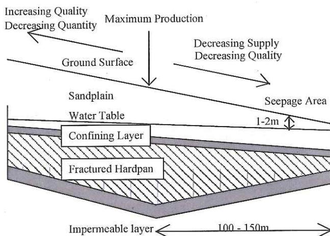
Figure 2. Profile of sandplain seeps with maximum potential for development into water supplies.
