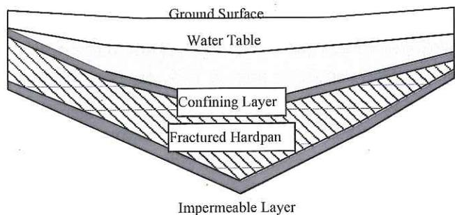
Figure 3. Cross-section across the face of a sandplain seep developed for a water supply.
