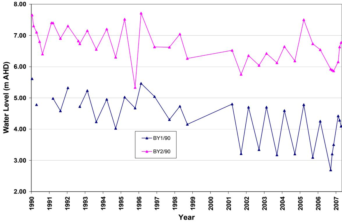
**Figure 12 Hydrograph of Superficial monitoring bore BY2/90 and Yarragadee monitoring bore BY1/90, approximately 200 m to the south of the Harewoods Rd site**
