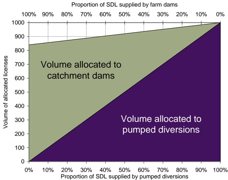
■ **Figure 9-1 Hypothetical relationship between volume of an SDL of 1,000 ML distributed between pumped diversions and farm dams.**
