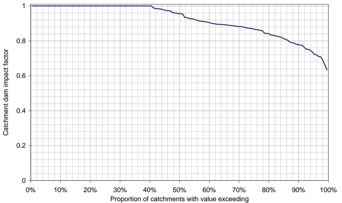
■ **Figure 9-5 Frequency exceedance plot of the volume of farm dam and pumped diversion with an equivalent impact for 142 gauged catchments**
