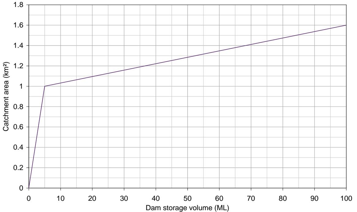
■ **Figure 9-4 Assumed relationship between dam storage volume and its catchment area for catchment dams in this study**
