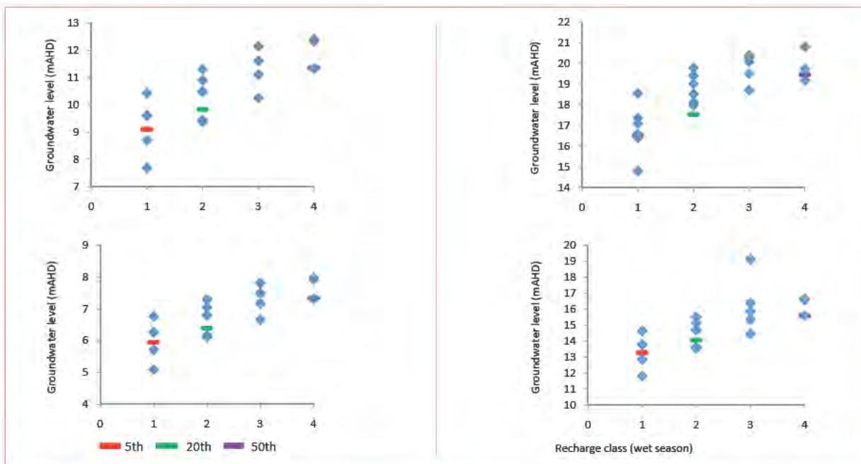
**Figure 12** Observed minimum annual groundwater levels for each recharge class at a) bore 2B, b) bore 8A, c) bore 15A and d) bore 22A
