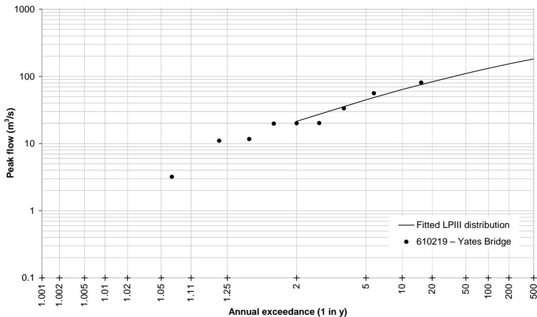
Figure 9 Flood-frequency plot for Capel River at Yates Bridge (610219)
