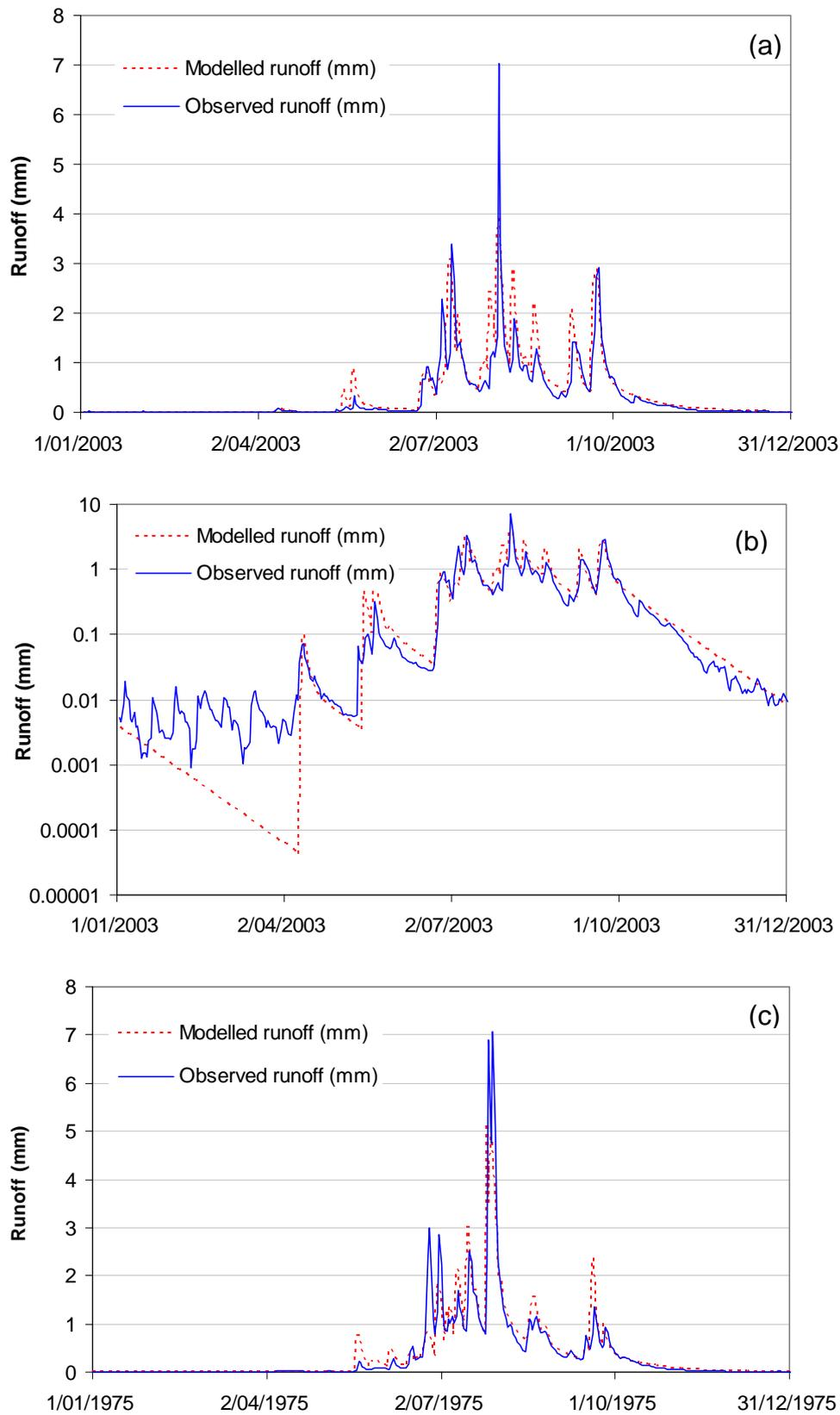
Figure 7 Comparison of observed and modelled daily flows for a calibration year (2003) - normal scale (a) and log-scale y axis (b) - and a verification year (1975) (c)
