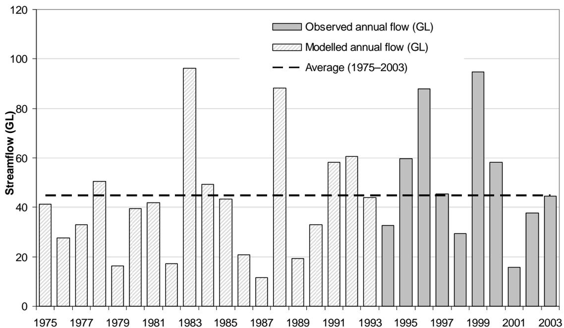
*Figure 18 Modelled and observed annual streamflow record for Capel River at Capel Railway Bridge (610010)*
