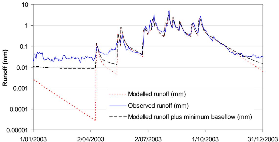
Figure 17 Comparison of observed, AWBM-modelled and modelled plus minimum daily flow for a calibration year (2003) (log-scale y axis)
