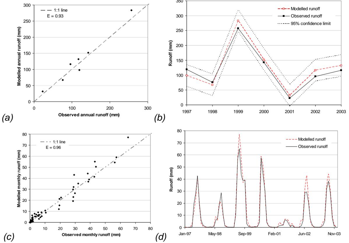
Figure 6 Observed versus modelled runoff at Yates Bridge, results for (a,b) annual timescale and (c,d) monthly timescale
