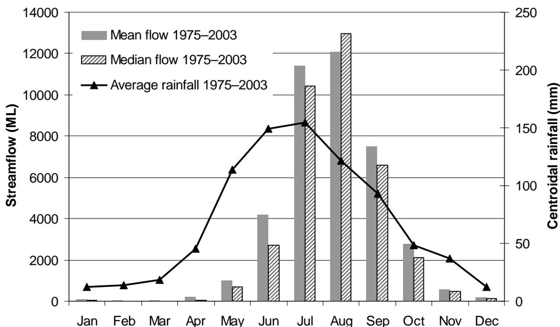
Figure 10 Average and median monthly streamflow for Capel River at Yates Bridge and average centroidal rainfall
