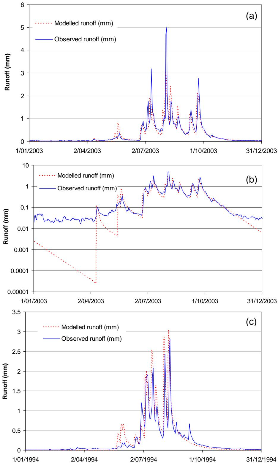
Figure 16 Comparison of observed and modelled daily flows for a calibration year (2003) - normal scale (a) and log-scale y axis (b) - and a verification year (1994) (c)
