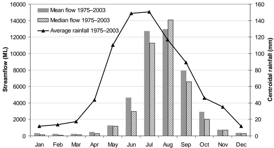
Figure 20 Average and median monthly streamflow for Capel River at Capel Railway Bridge and average centroidal rainfall
