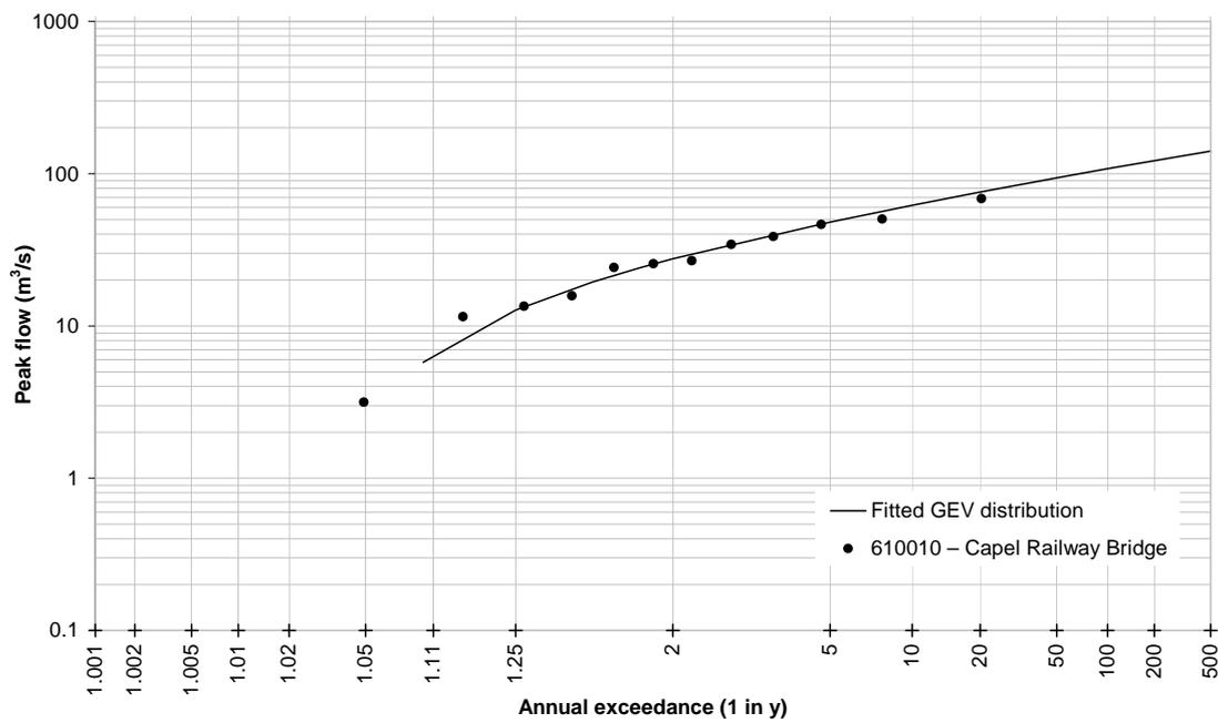
Figure 19 Flood-frequency plot for Capel River at Capel Railway Bridge (610010)
