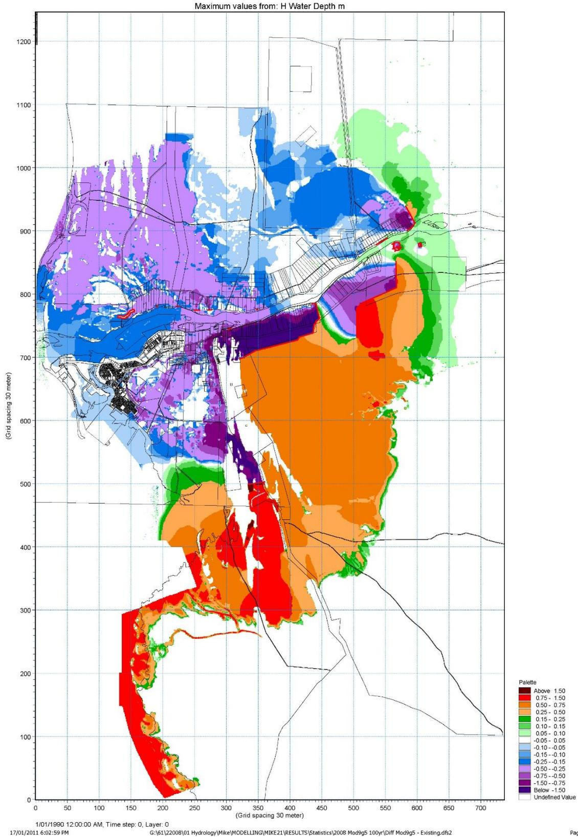
Figure 29 Modelled impact of levees constructed in 2015 on peak flood levels for the one per cent (1 in 100) AEP flood
