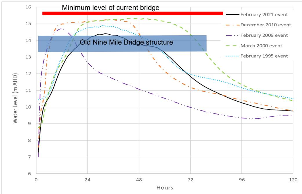
Figure 12 Comparison of recorded water levels at DWER’s streamflow gauging station at Nine Mile Bridge\*
