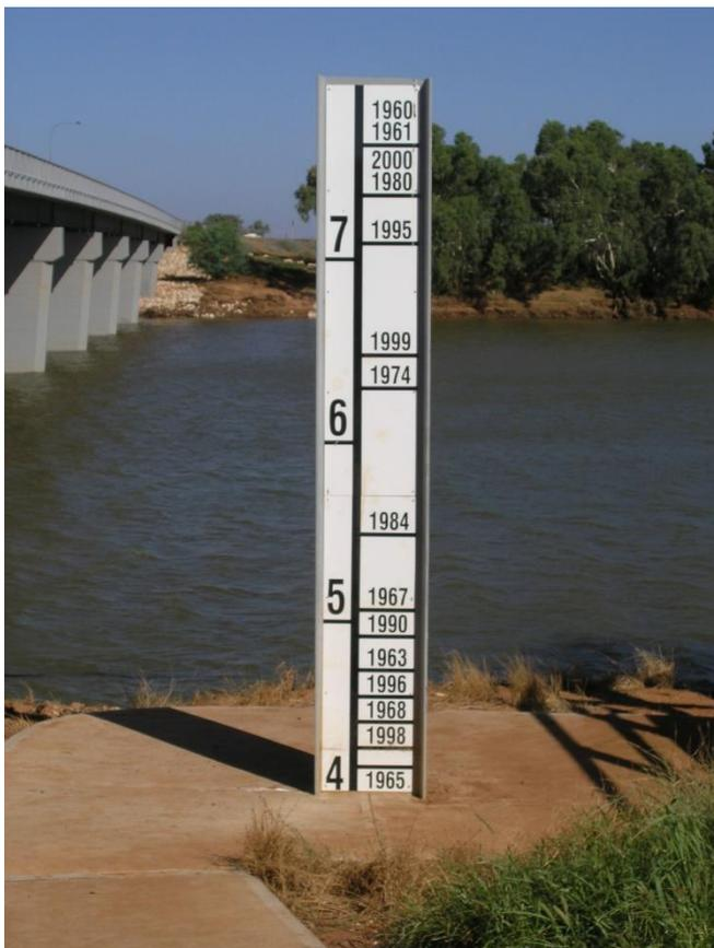
*Figure 33 Staff gauge installed downstream of the Nine Mile Bridge*
