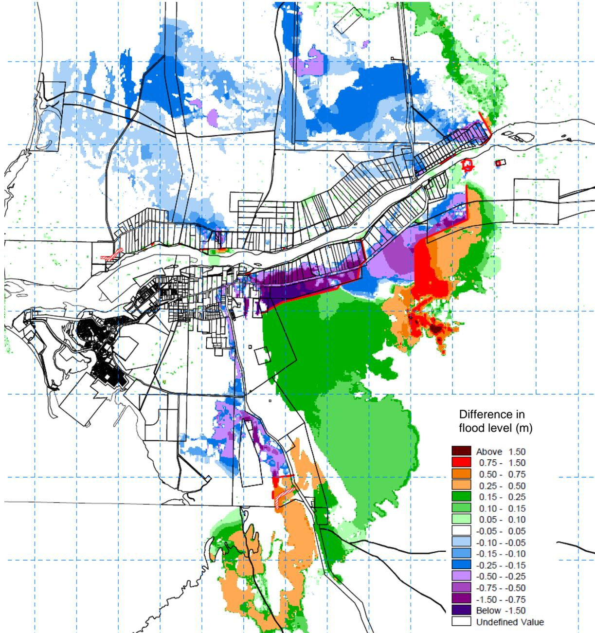
Figure 28 Modelled impact of levees constructed in 2015 on peak flood levels for the 1995 flood
