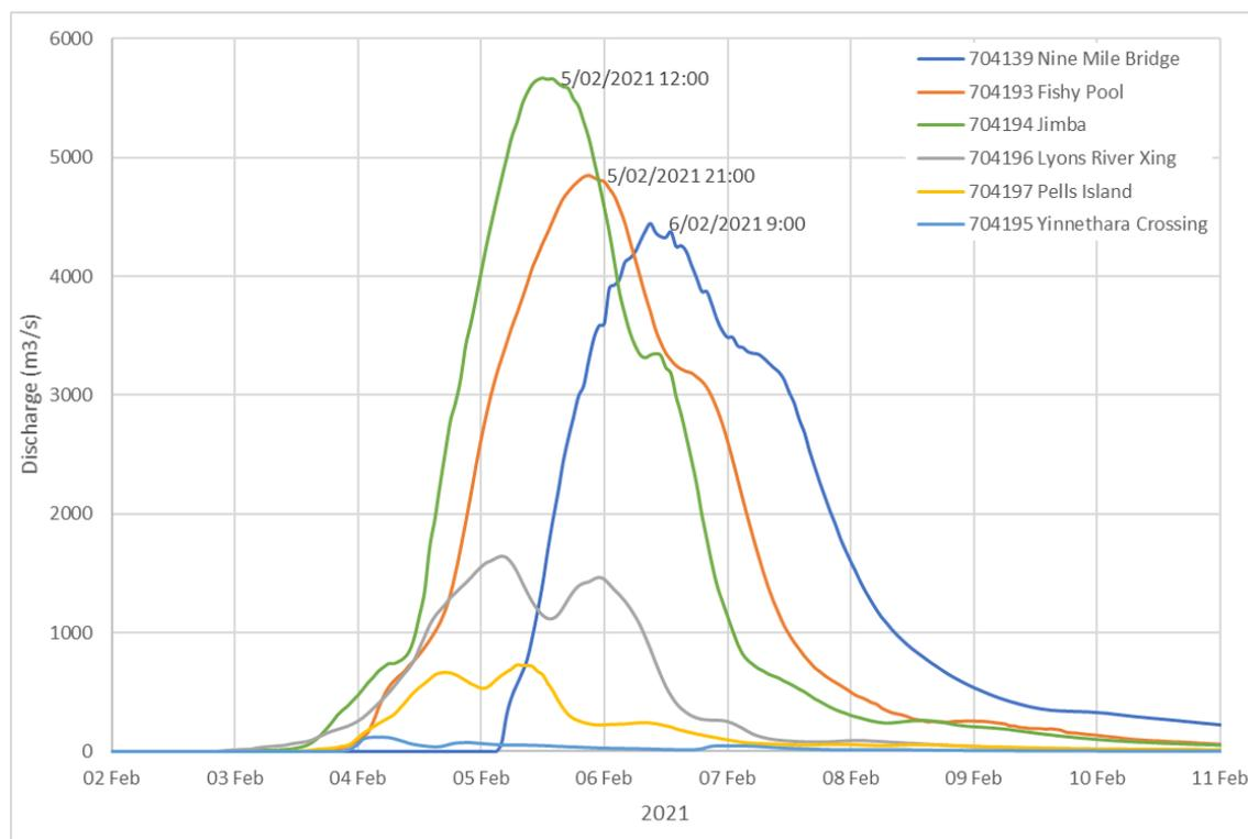
Figure 10 Streamflow at DWER's streamflow gauges in the Gascoyne River catchment during the February 2021 event
