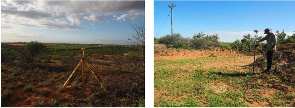
*Figure 16 RTK survey (left: base station set up at Landgate survey benchmark, right: rover unit and flood debris mark)*
