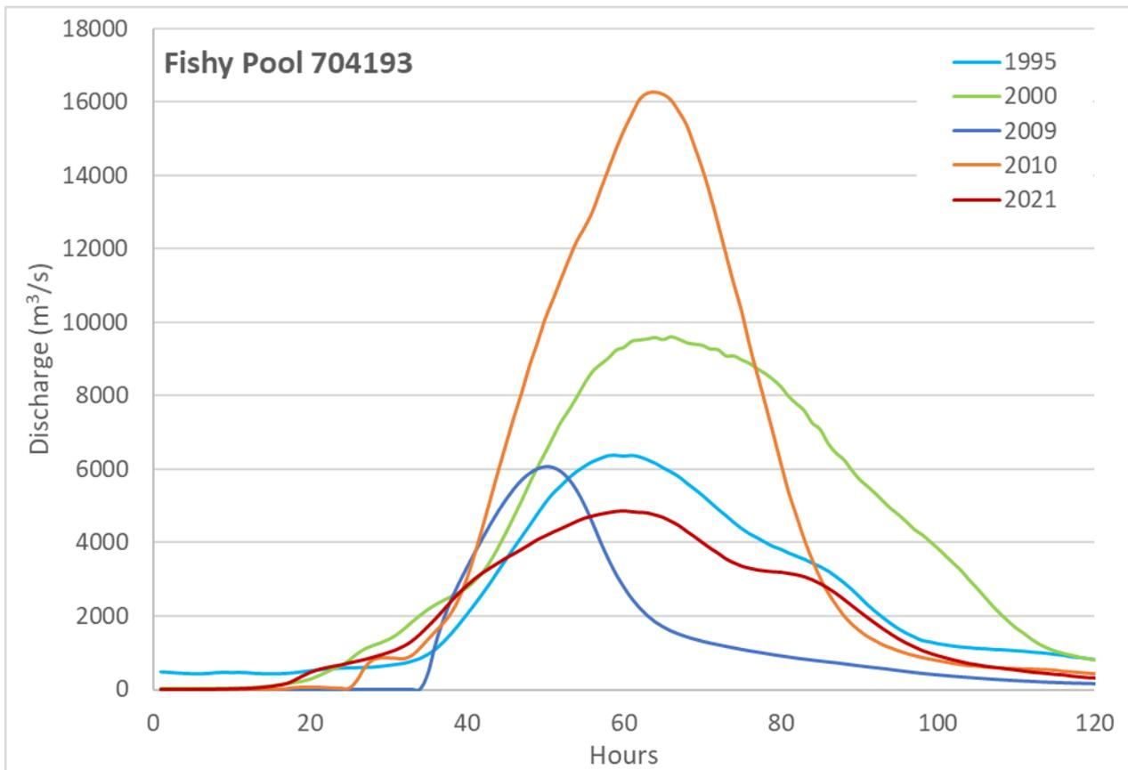
Figure 11 Comparison of the February 2021 streamflow to other major events at DWER’s streamflow gauge on the Gascoyne River at Fishy Pool
