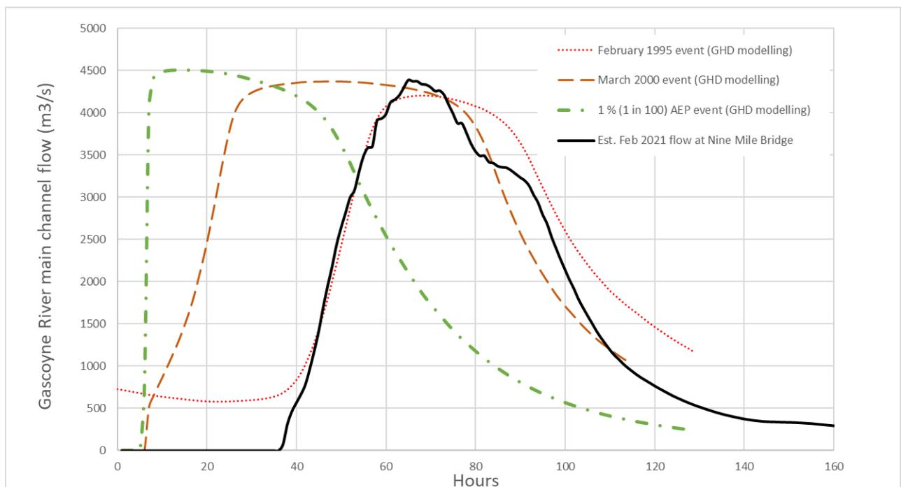
*Figure 30 Comparison of recorded 2021<sup>#</sup> flow with modelled Gascoyne River main channel flows in a cross-section at Research Road*
