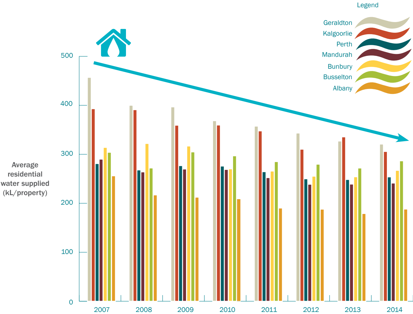
Figure 6 | Average scheme water use per residential property in Western Australia's major urban centres
