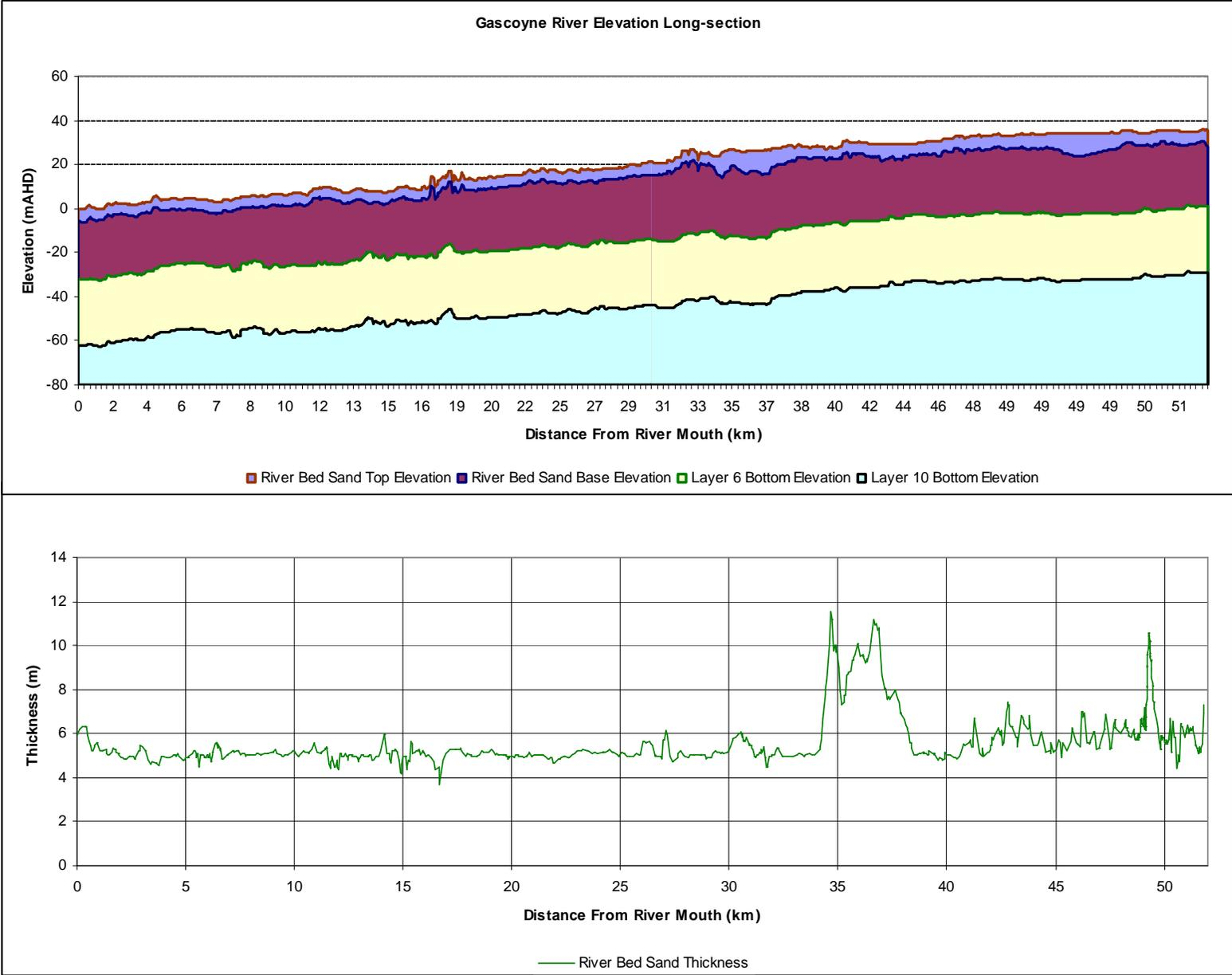
Figure 7: River Bed Sand Top and Bottom Elevations and Thickness
