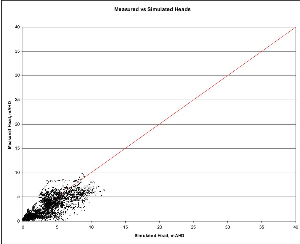
Figure 30: Verification Measured vs. Simulated Heads
