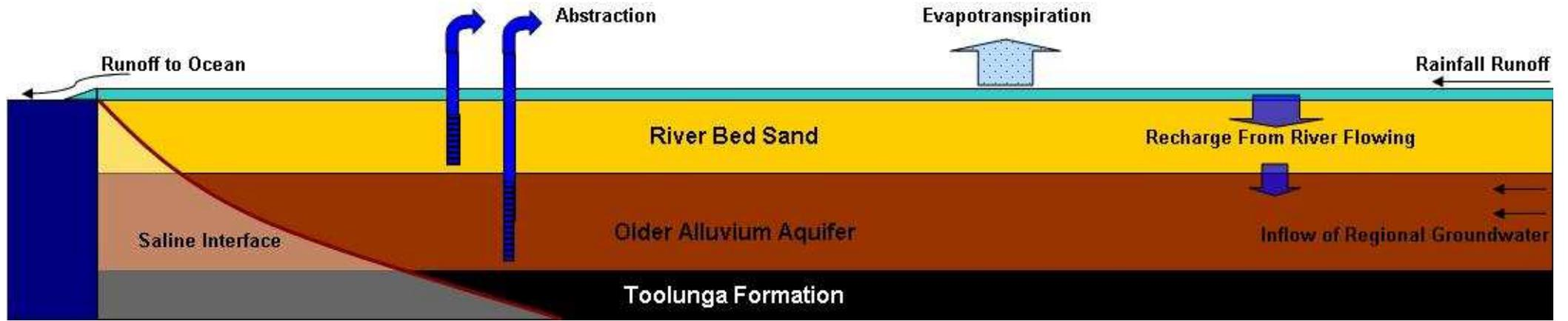
Figure 10: Solute Transport Conceptual Hydrogeology – Long Section
