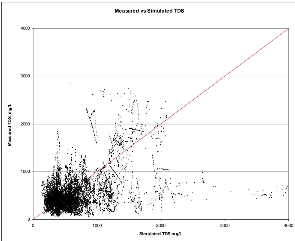
Figure 31: Verification Measured vs. Simulated Concentrations
