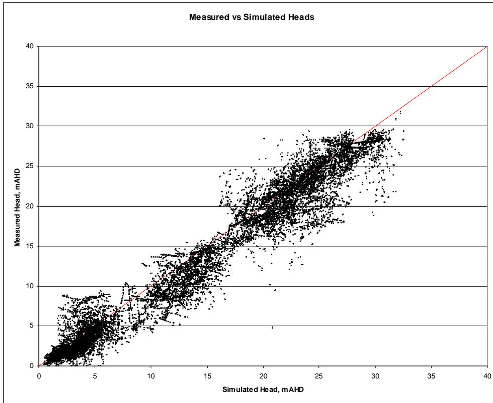
**Figure 28: Calibration: Measured vs. Simulated Heads**
