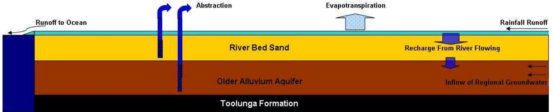
Figure 8: Flow Conceptual Hydrogeology
