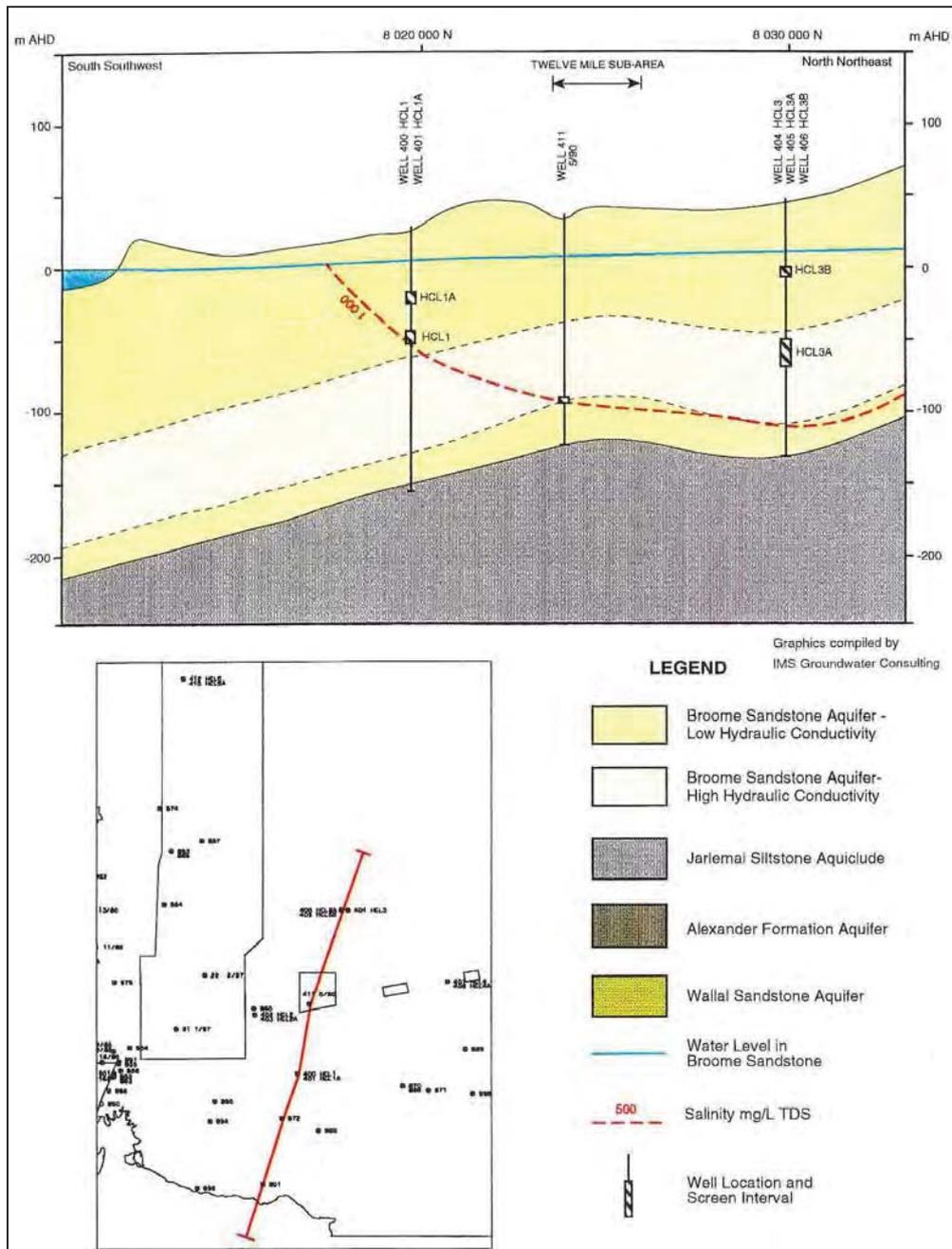
Figure 4: Shallow hydrogeological cross-section of 12 Mile subarea (WAWA 1994)
