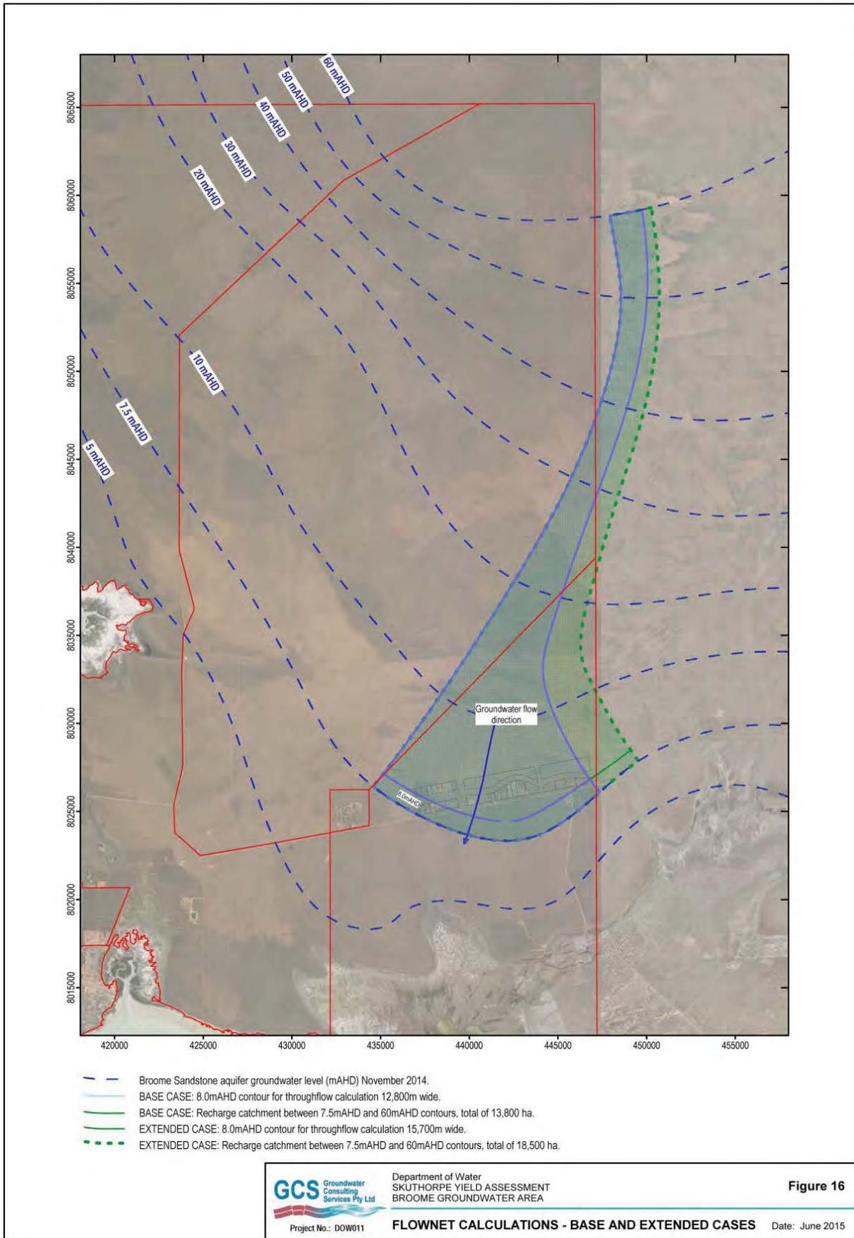
Figure 10: Flow-net calculations for base and extended scenarios
