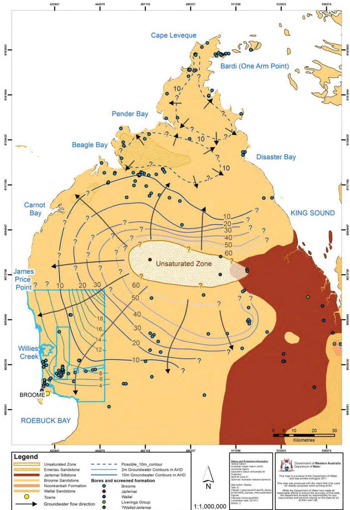
Figure 3: Location of aquifers and regional groundwater flow, Dampier Peninsula (note: contours use maximum water levels; Searle 2011)
