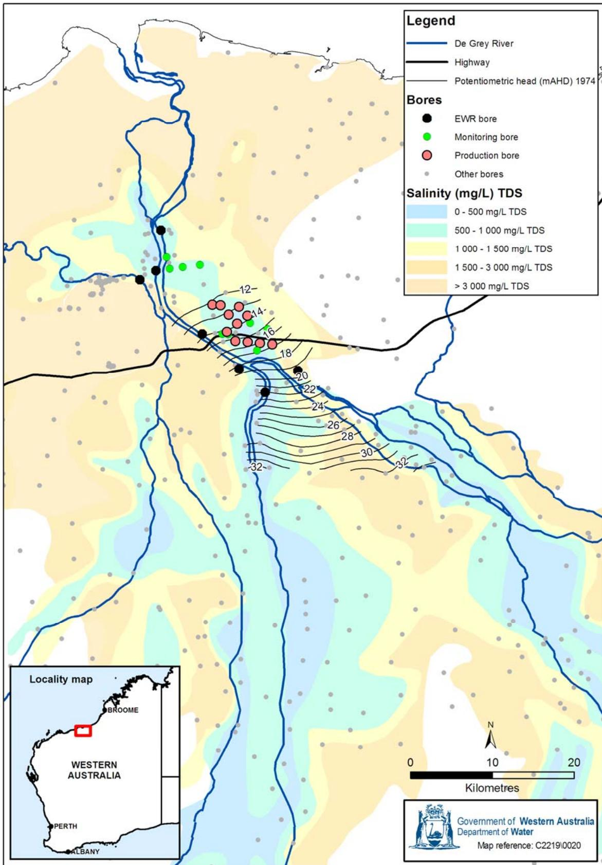
Figure 7 De Grey alluvial aquifer salinity levels
