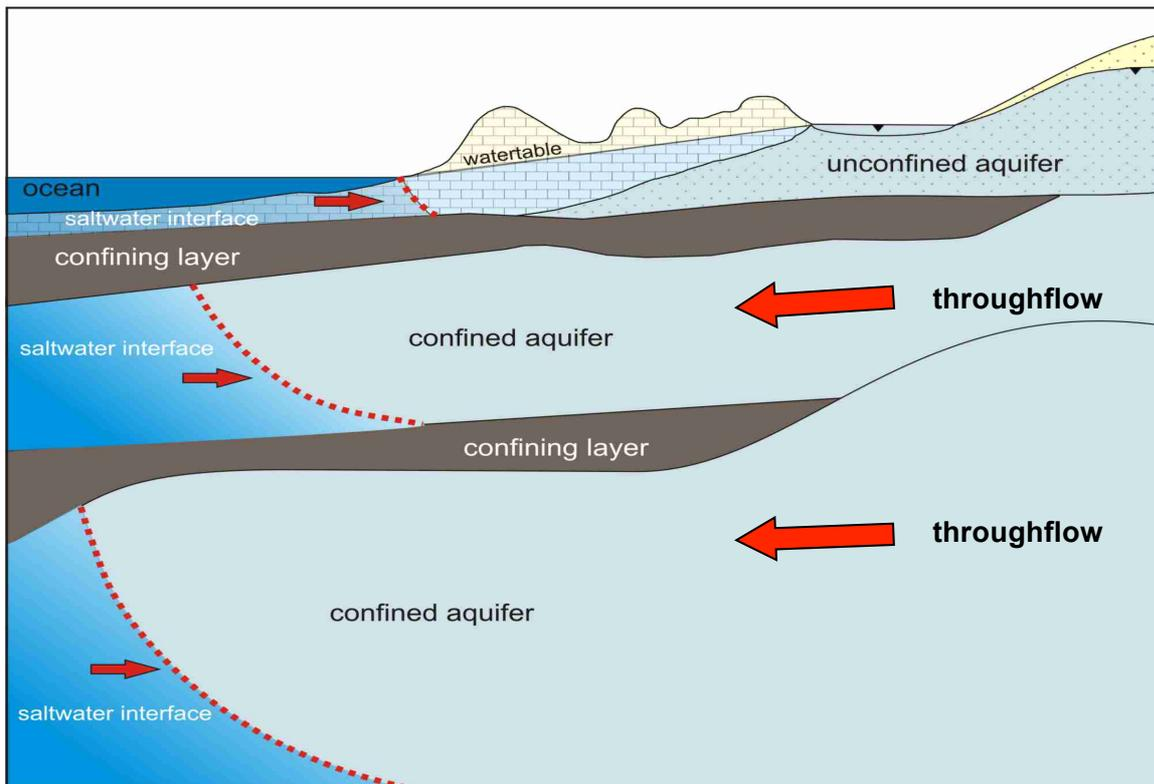
*Figure 20 Schematic of seawater interface in a layered aquifer system similar to the plan area*
