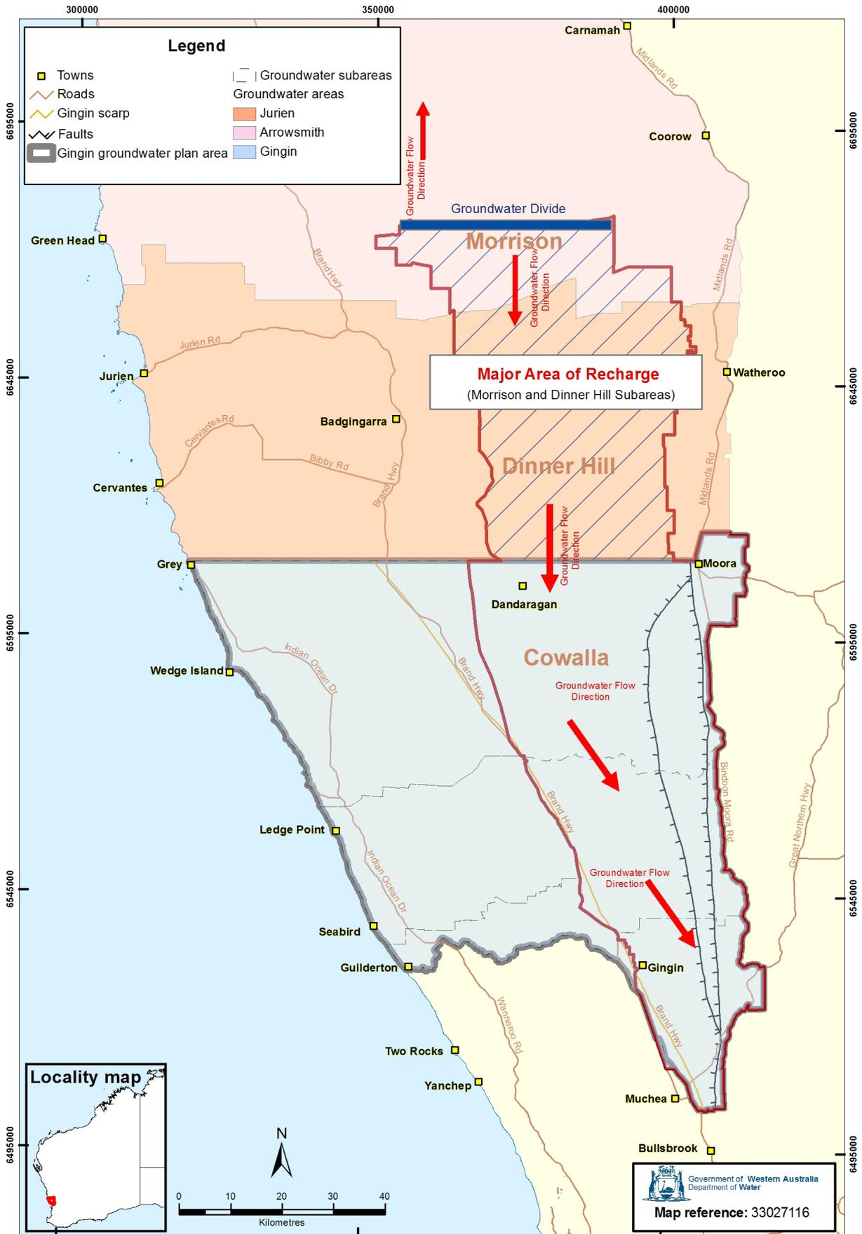
Figure 13 Groundwater recharge and flow within the Leederville-Parmelia aquifer
