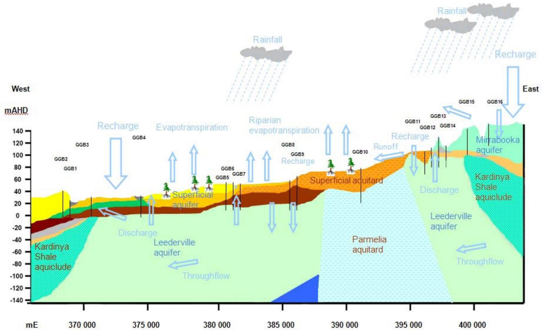
Figure 4 Conceptual model of the hydrogeology in the Gingin groundwater area
