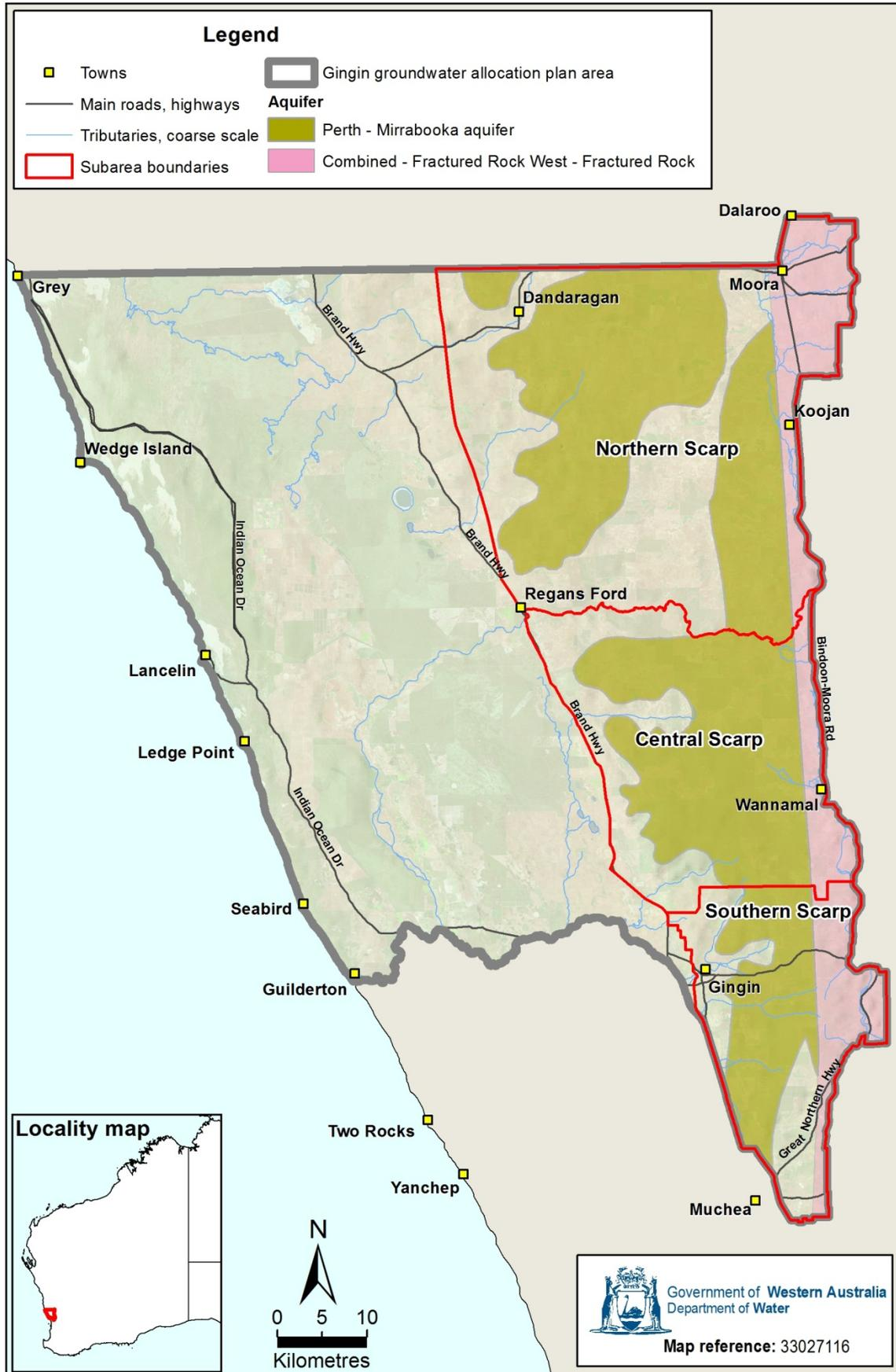
Figure 6 Subareas covering the Mirrabooka and fractured rock aquifers
