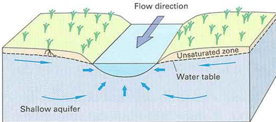
Figure 18 Schematic of areas where baseflow occurs (Winter et al. 1998)
