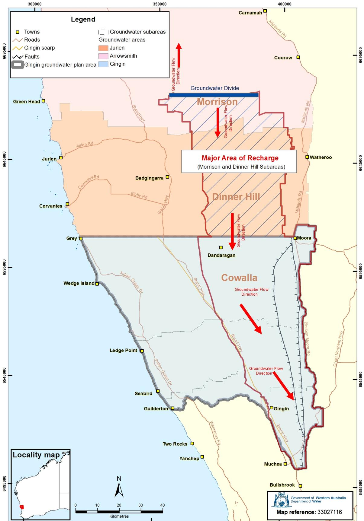
Figure 21 Groundwater recharge and flow within the Leederville-Parmelia aquifer
