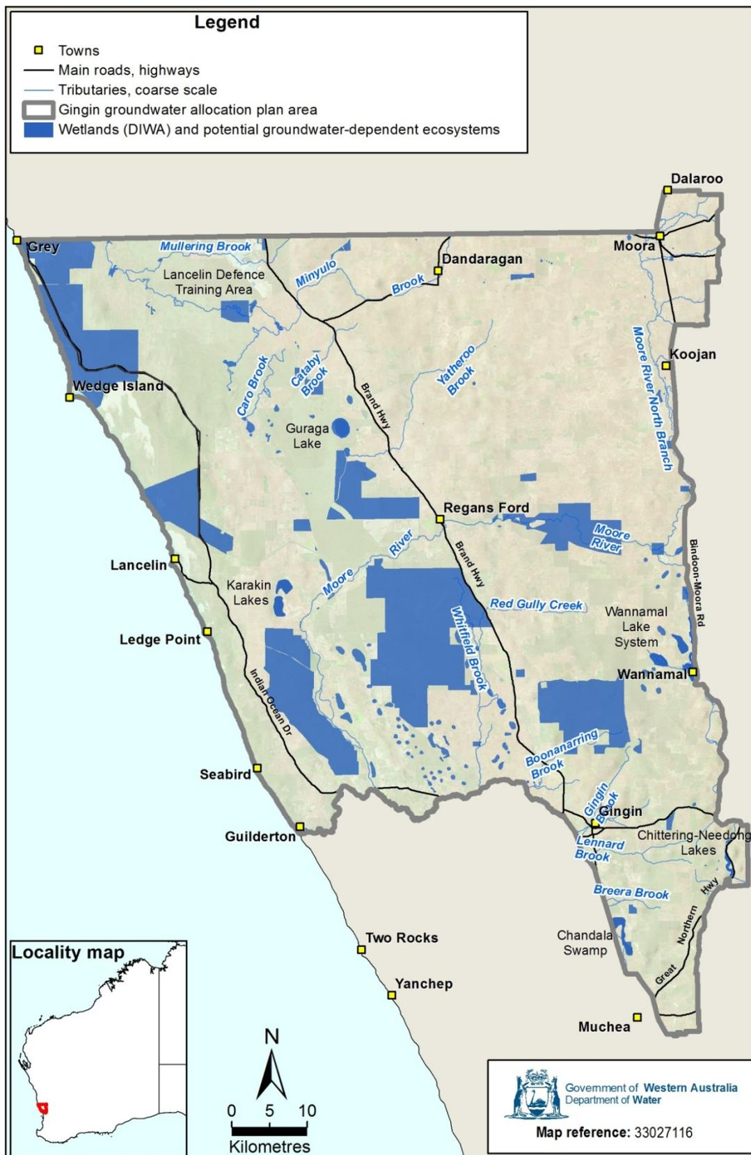
Figure 17 Groundwater-dependent ecosystems in the plan area derived by overlying remnant vegetation and wetlands on depth-to-groundwater data
