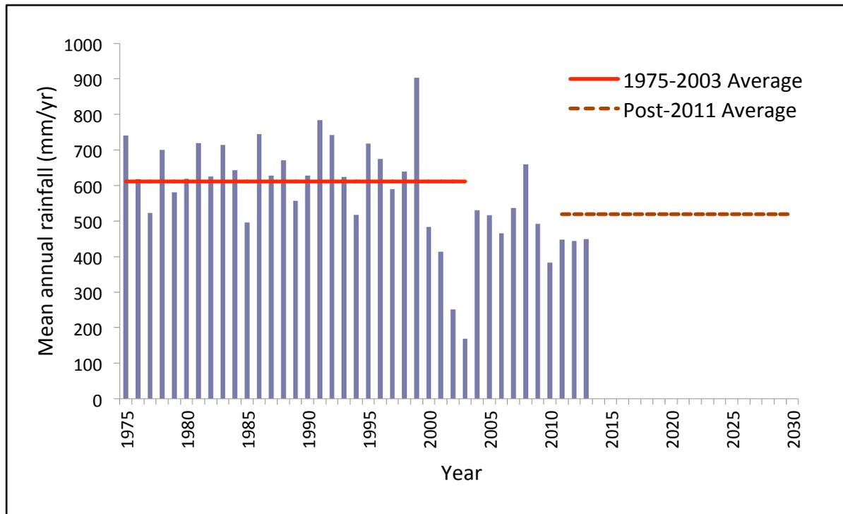
*Figure 12 Plots showing the future dry climate scenario used to revise allocation limits (15 per cent reduced mean annual rainfall to 2030 illustrated using Bureau of Meteorology station at Gingin town site)*
