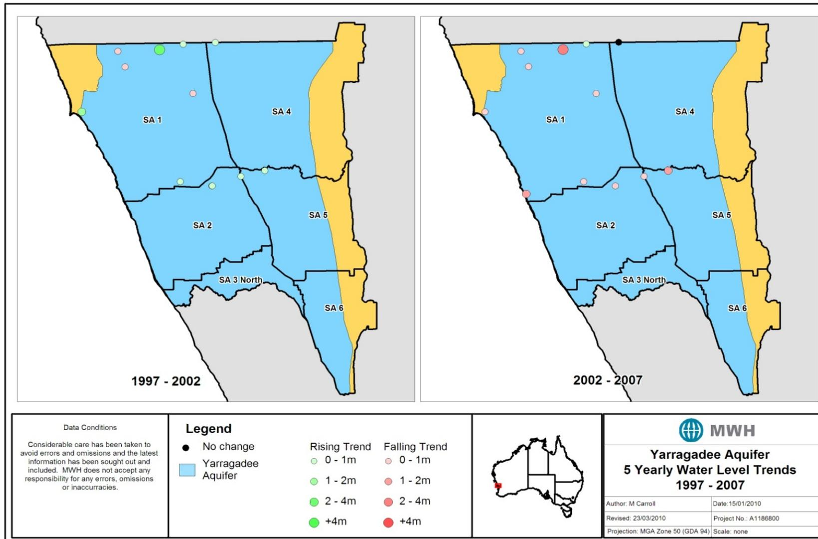
Figure 16 Groundwater trends within the Yarragadee aquifer in the Gingin groundwater area (MWH 2010)
