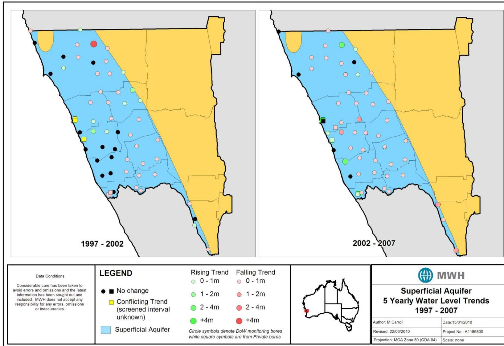
Figure 14 Groundwater trends within the superficial aquifer in the Gingin groundwater area (MWH 2010)
