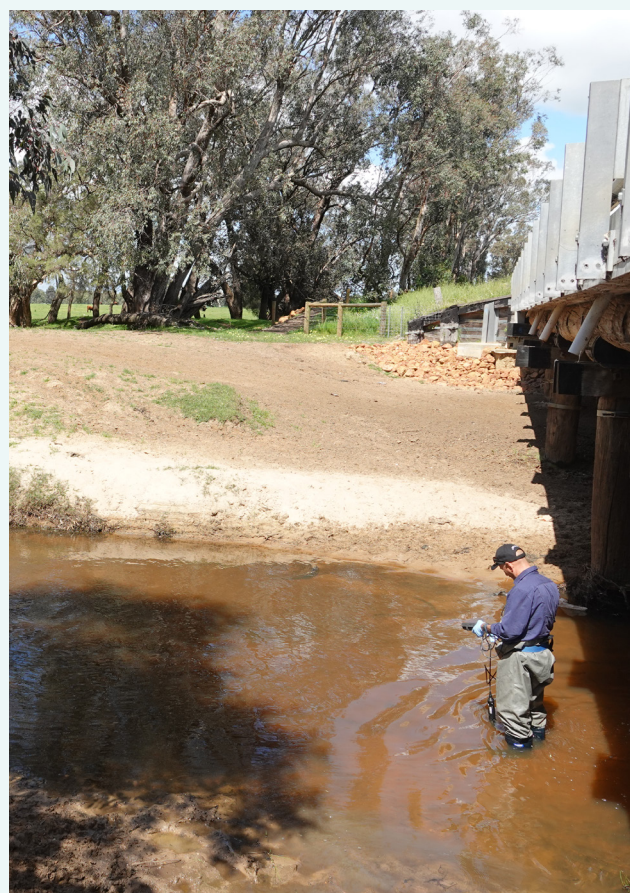
Using an in-situ probe to measure pH and salinity at the South Dandalup River sampling site, September 2018.
