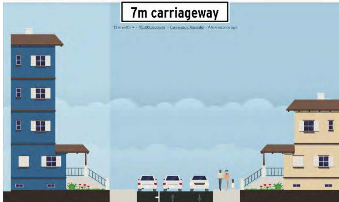
Figure 24: Access Street – Diagram of physical determinants for width based on Liveable Neighbourhoods
