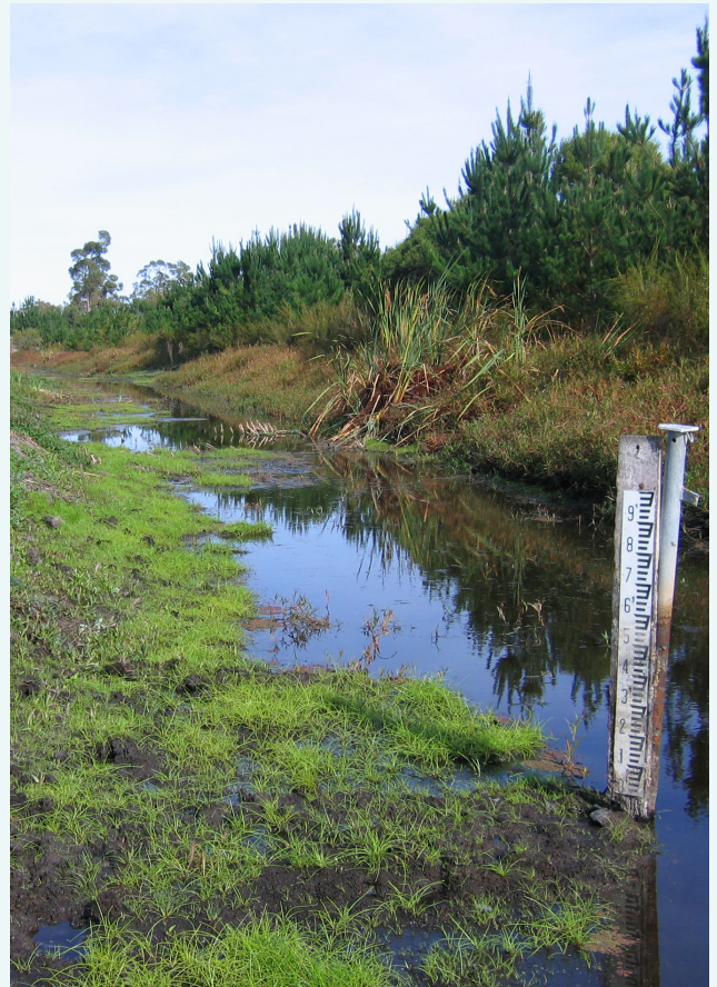
A staff gauge at the Meredith Drain sampling site, May 2020.
