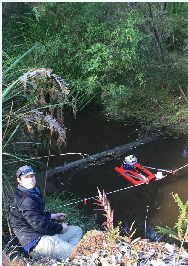
Collecting discharge measurements using a StreamPro Acoustic Doppler Current Profiler, July 2016.
