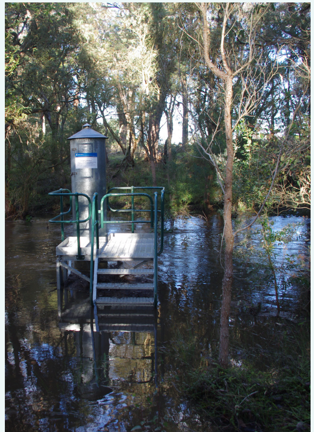
The King River gauging station submerged during high flows, June 2012. Note the difference in water levels with the photograph on the previous page.
