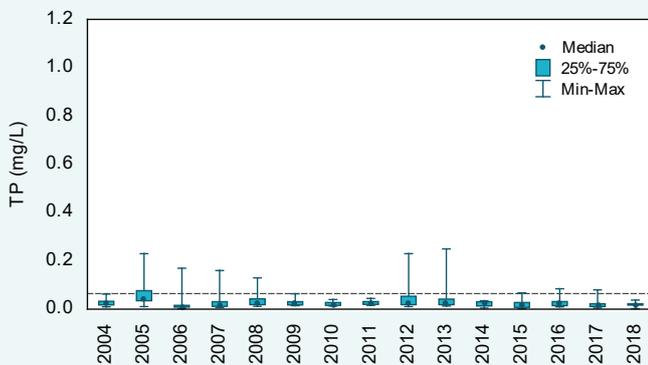
Total phosphorus concentrations, 2004–18 at site 602004. The dashed line is the ANZECC trigger value for lowland rivers.
