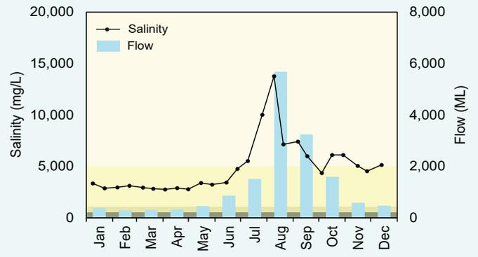
2018 salinity concentrations and monthly discharge at site 602004. The shading refers to the SWRWQA classification bands.
