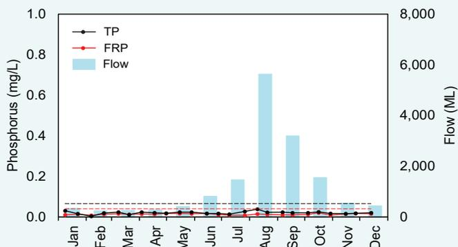
2018 phosphorus concentrations and monthly discharge at 602004. The dashed lines are the ANZECC trigger values for the different P species in lowland rivers.
