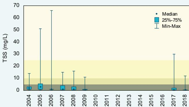
Total suspended solids concentrations, 2004–18 at site 602004. The shading refers to the SWRWQA classification bands.
