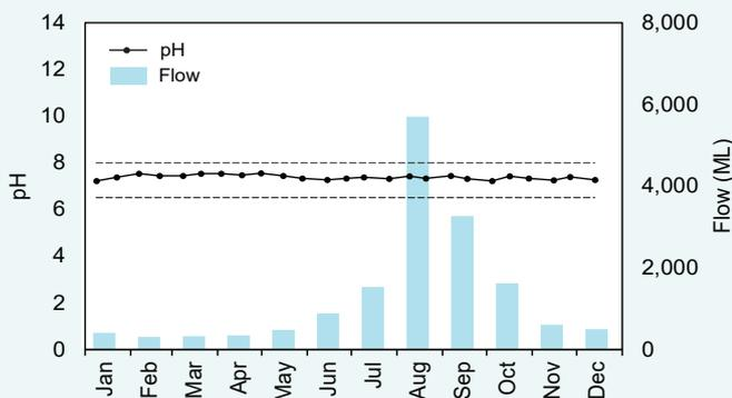
2018 pH levels and monthly discharge at 602004. The dashed lines are the upper and lower ANZECC trigger values for lowland rivers.
