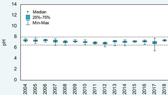
pH levels, 2004–18 at site 602004. The dashed lines are the upper and lower ANZECC trigger values for lowland rivers.
