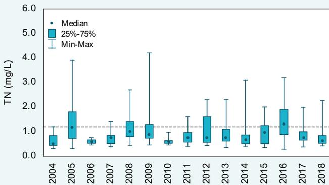
Total nitrogen concentrations, 2004–18 at site 602004. The dashed line is the ANZECC trigger value for lowland rivers.
