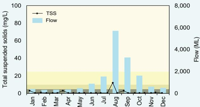
2018 total suspended solids concentrations and monthly discharge at 602004. The shading refers to the SWRWQA classification bands.
