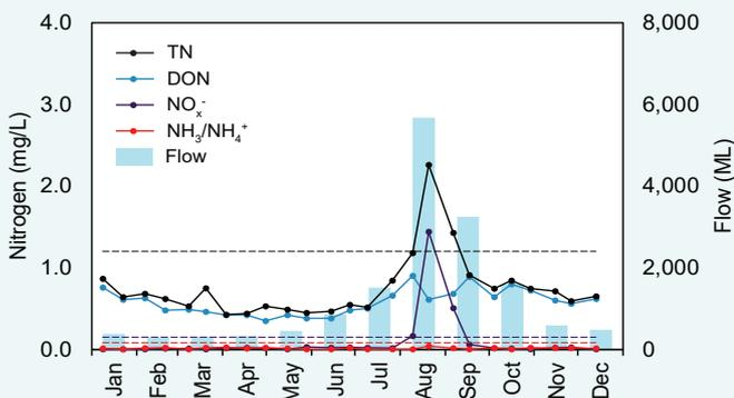
2018 nitrogen concentrations and monthly discharge at 602004. The dashed lines are the ANZECC trigger values for lowland rivers for the different N species.
