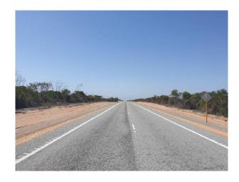
The project saw the road widened to a 9-metre seal on an 11-metre formation, along with resealing work and the installation of audible edge lines. Initial design work included the extension of three culverts and the clearing of some vegetation to accommodate the widening in some sections, along with construction of an embankment.
