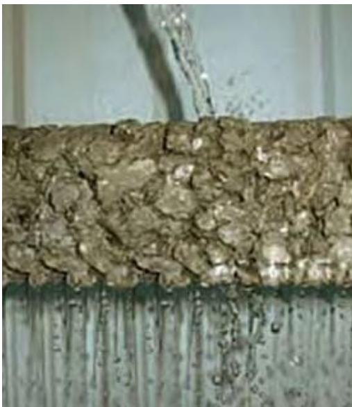
Infiltration through pervious paving. (Source: Washington Aggregates and Concrete Association 2006.)
