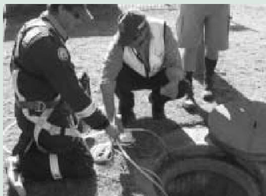
Figure 23. Testing of an industrial site stormwater drain for illicit discharges. (Photograph: former Department of Environment.)
