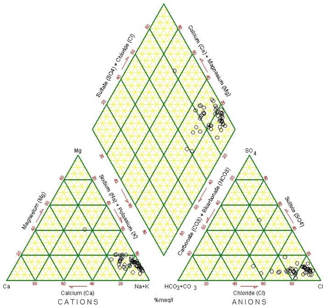
Figure 92 Cattamarra aquifer: hydrochemical trilinear diagram
