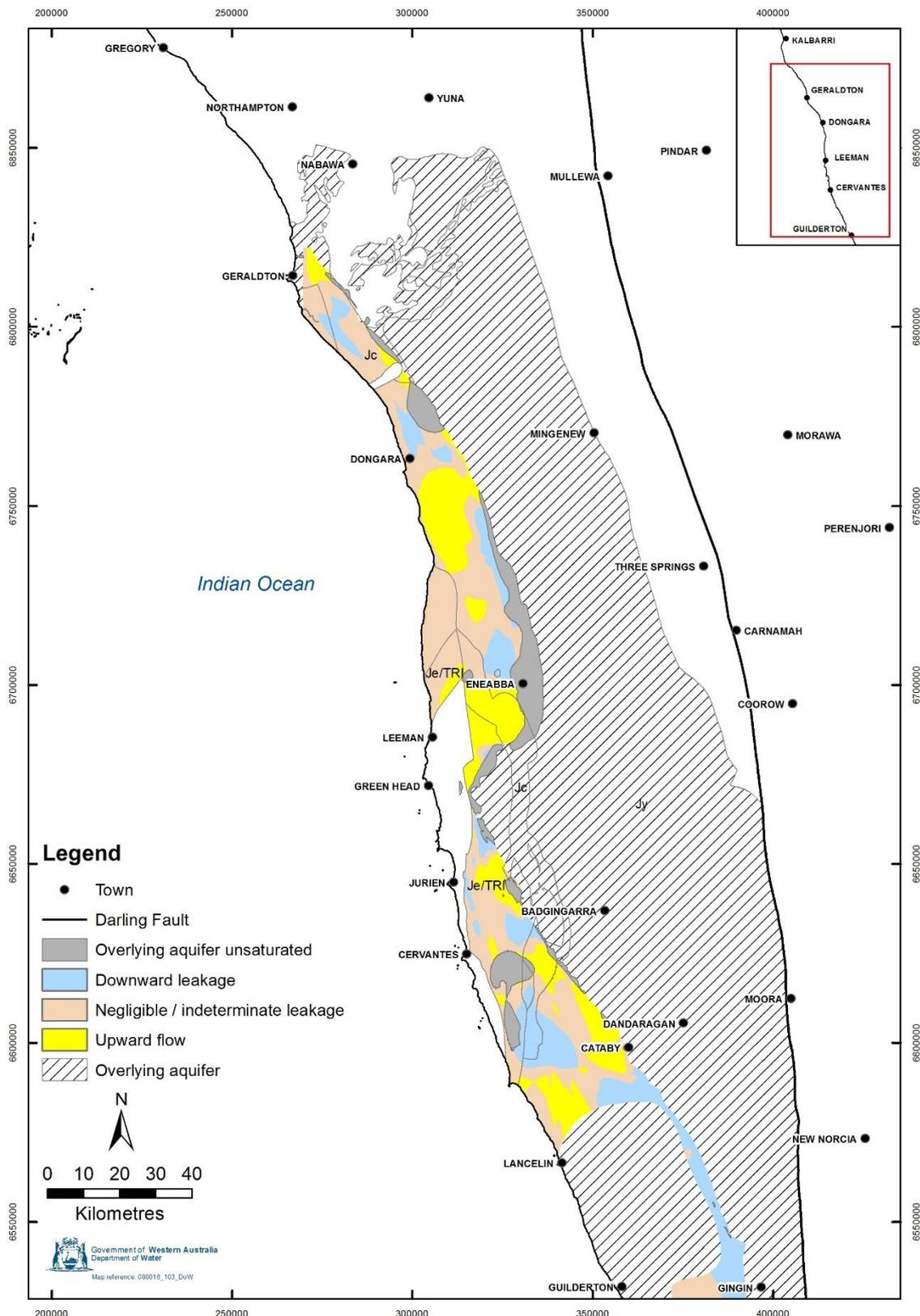
Figure 84 Vertical leakage between Yarragadee, Cattamarra and Eneabba–Lesueur aquifers and overlying Superficial and/or Leederville aquifer(s)
