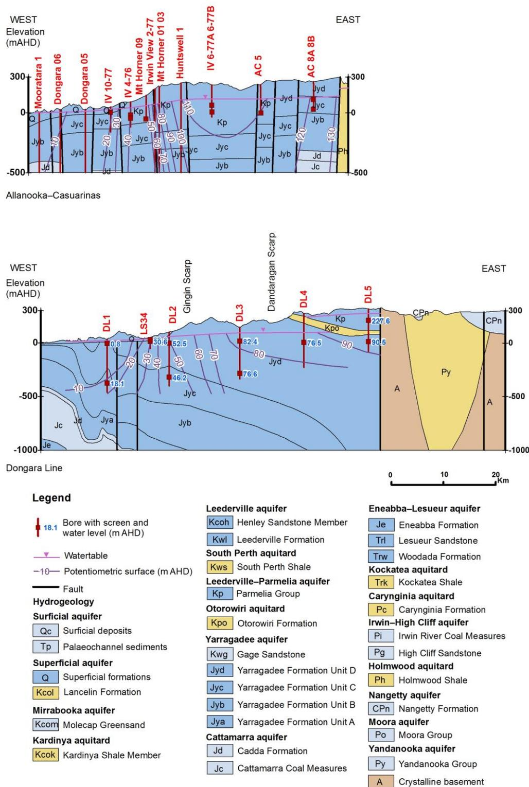
Figure 55 Hydrogeological cross-sections (hydraulic head)
