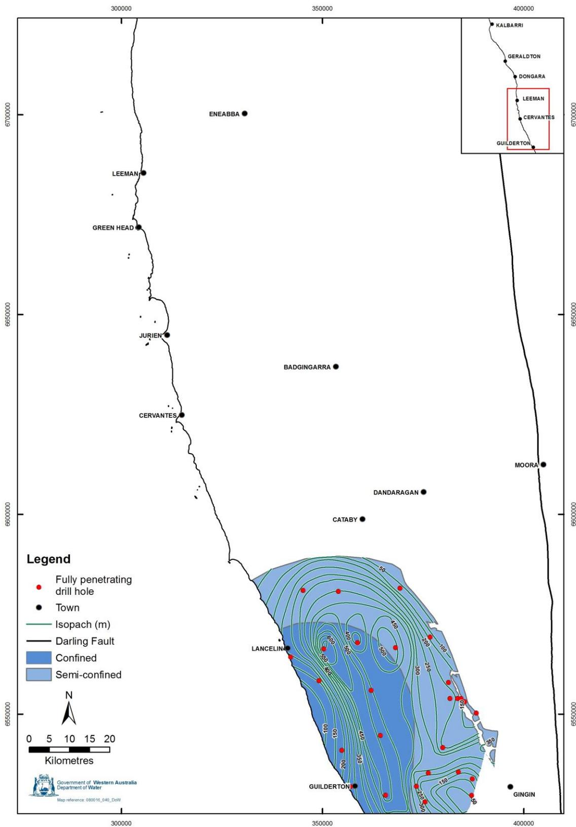
Figure 68 Leederville aquifer: aquifer thickness
