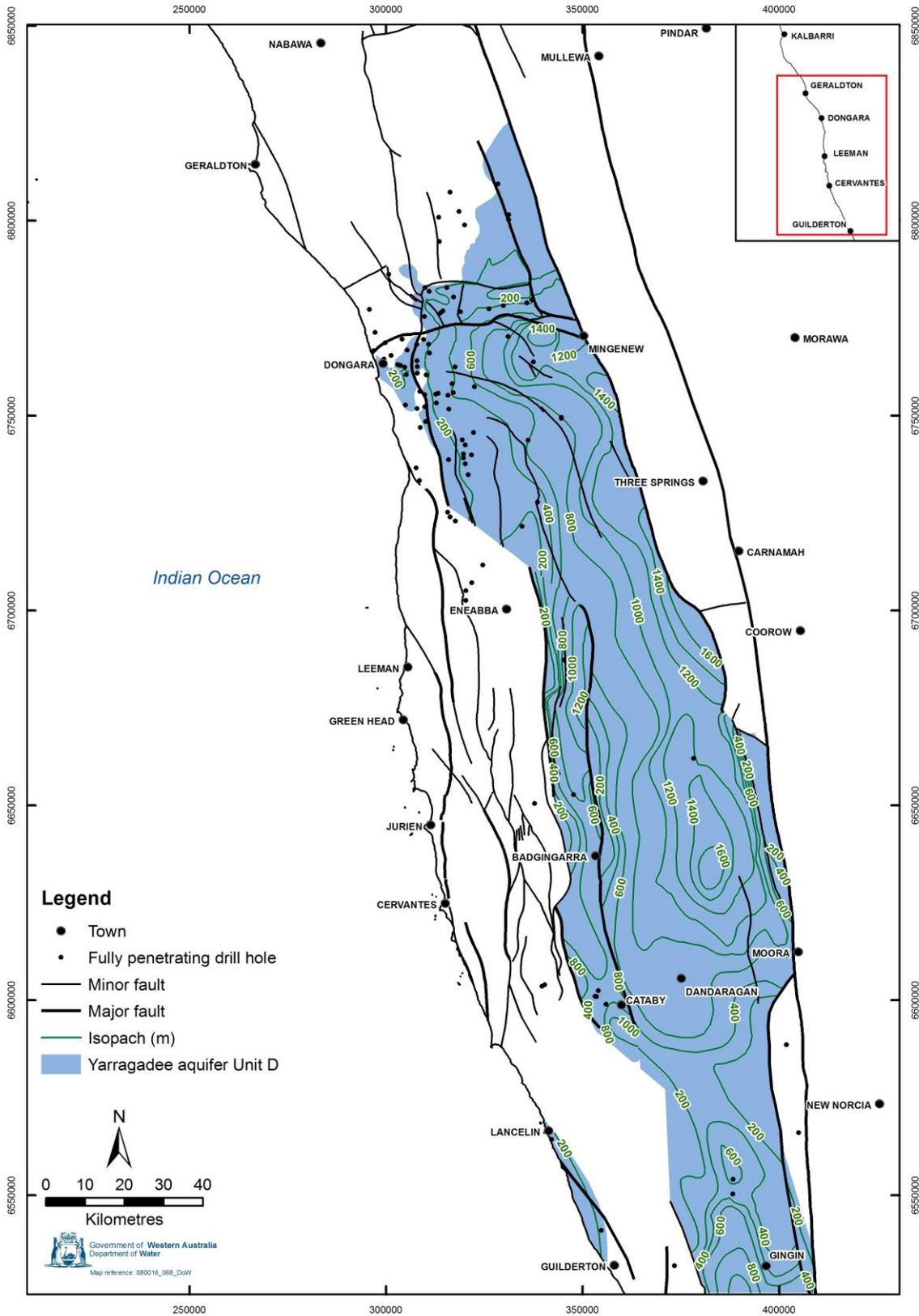
Figure 80 Yarragadee aquifer Unit D: aquifer thickness
