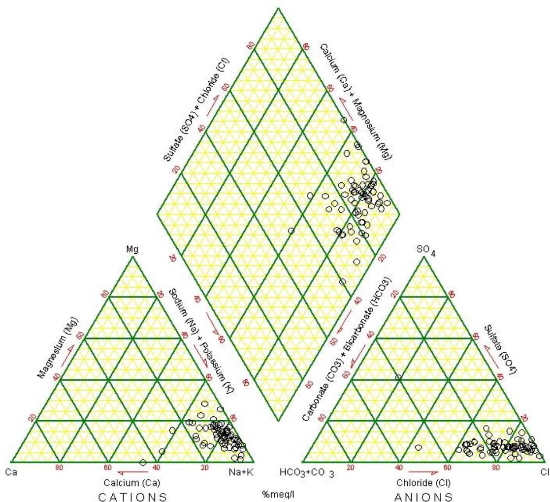
Figure 88 Yarragadee aquifer: hydrochemical trilinear diagram
