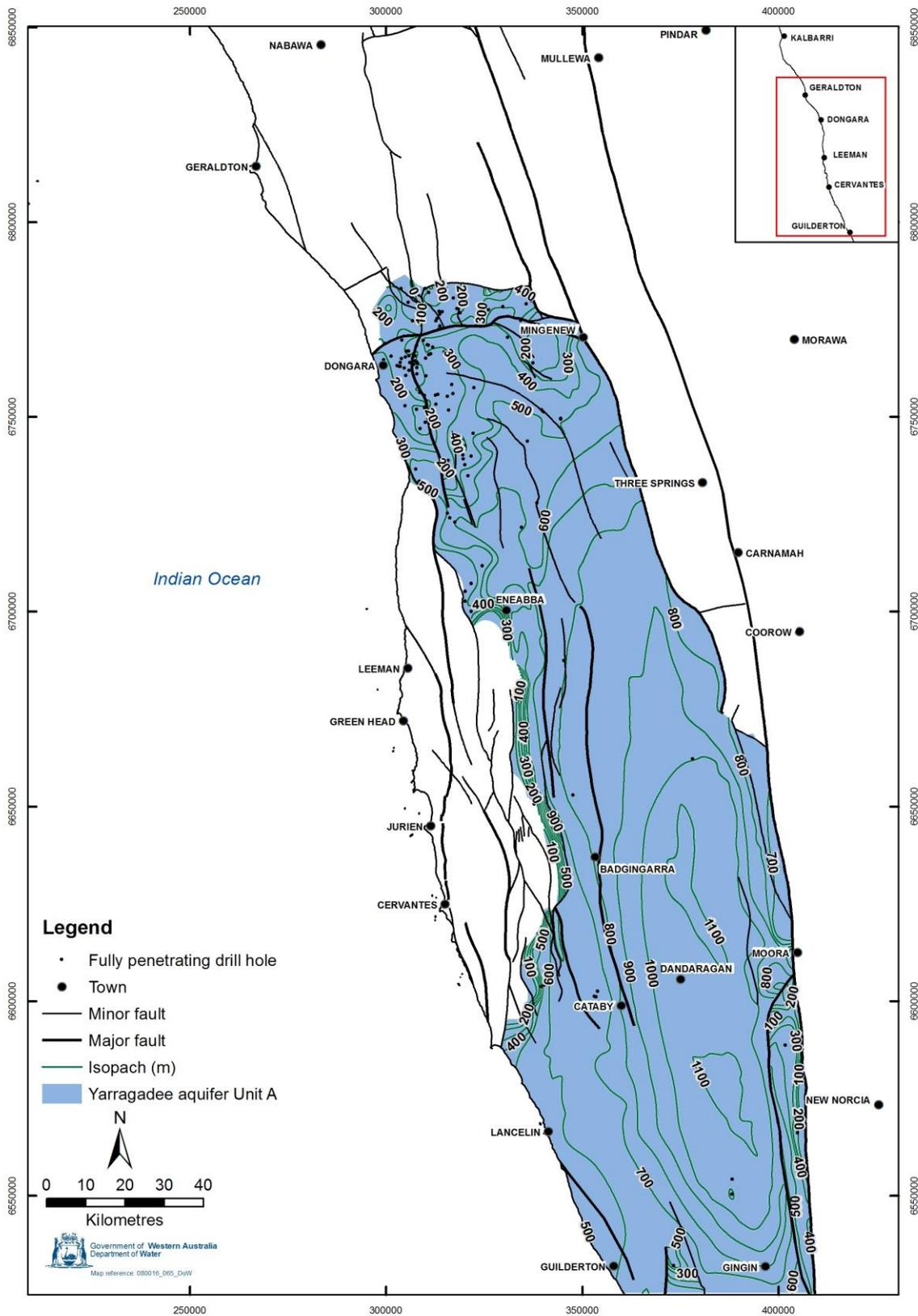
Figure 83 Yarragadee aquifer Unit A: aquifer thickness
