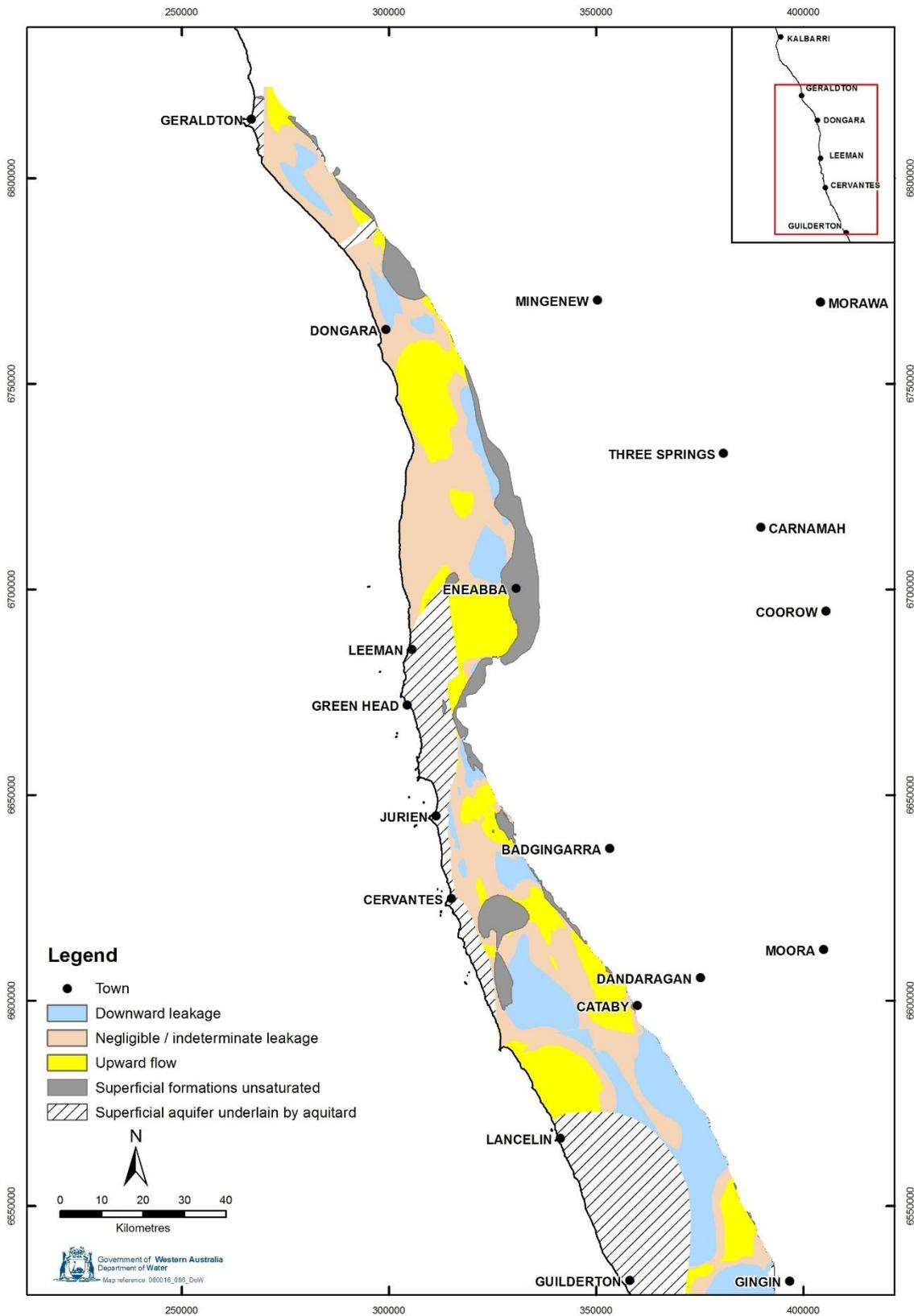
Figure 64 Direction of vertical leakage between Superficial aquifer and underlying aquifers (Leederville, Yarragadee, Cattamarra and Eneabba–Lesueur)
