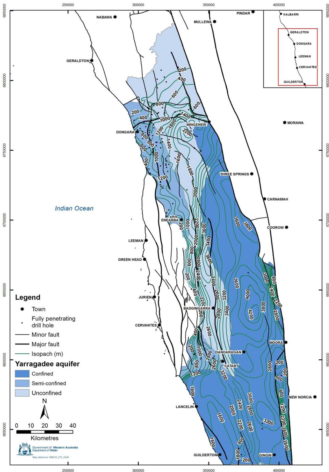
Figure 79 Yarragadee aquifer: saturated aquifer thickness
