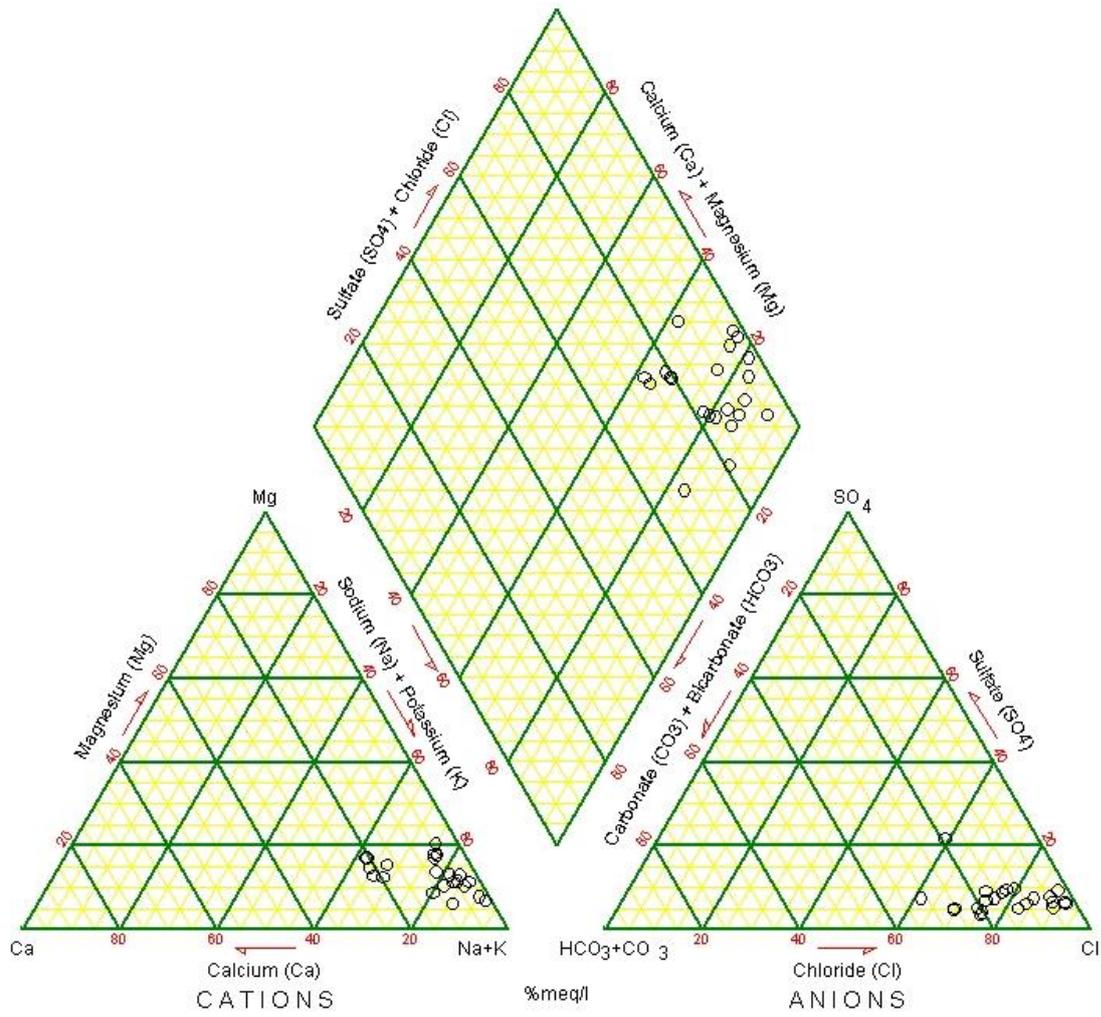
Figure 73 Leederville aquifer: hydrochemical trilinear diagram
