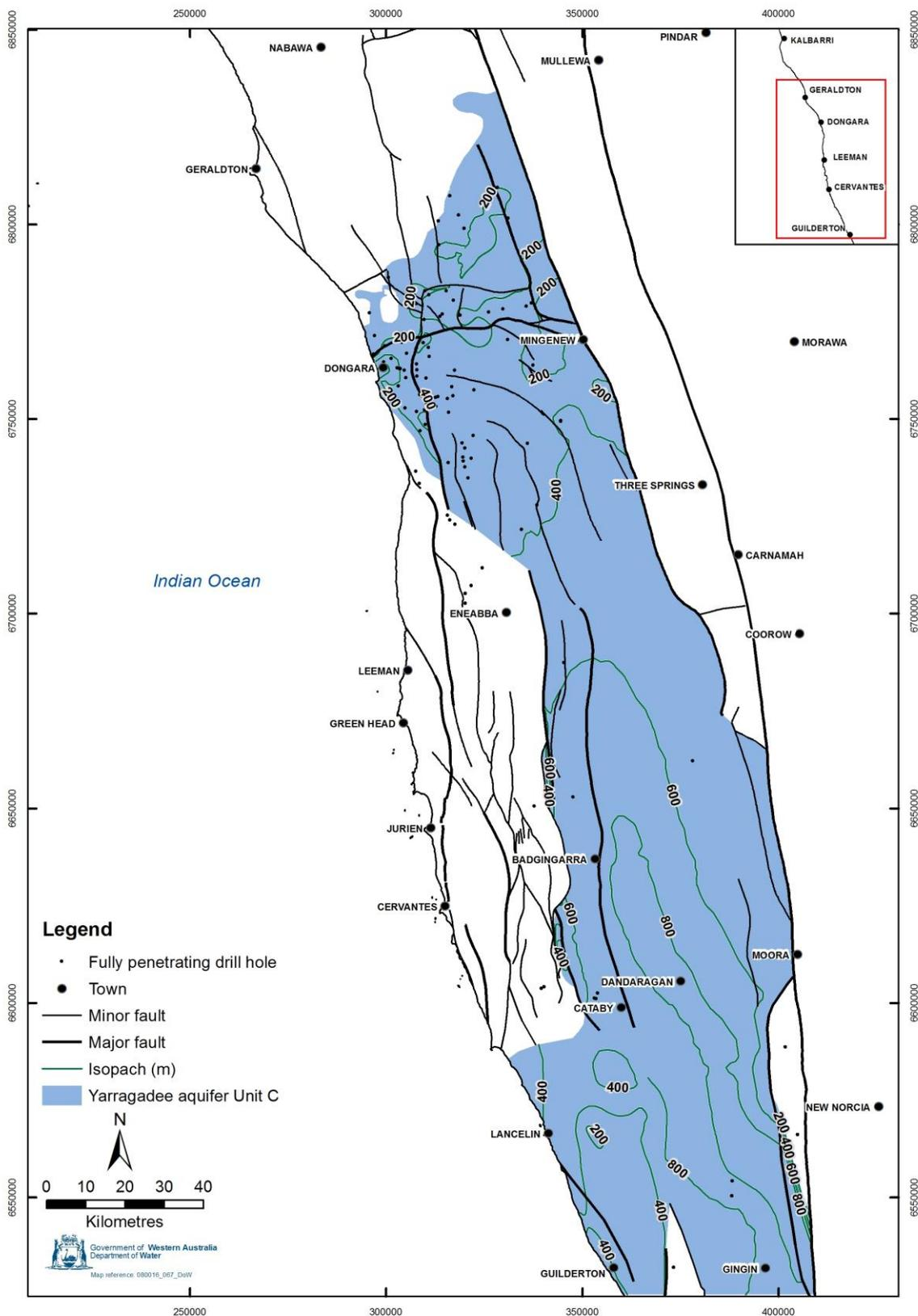
Figure 81 Yarragadee aquifer Unit C: aquifer thickness
