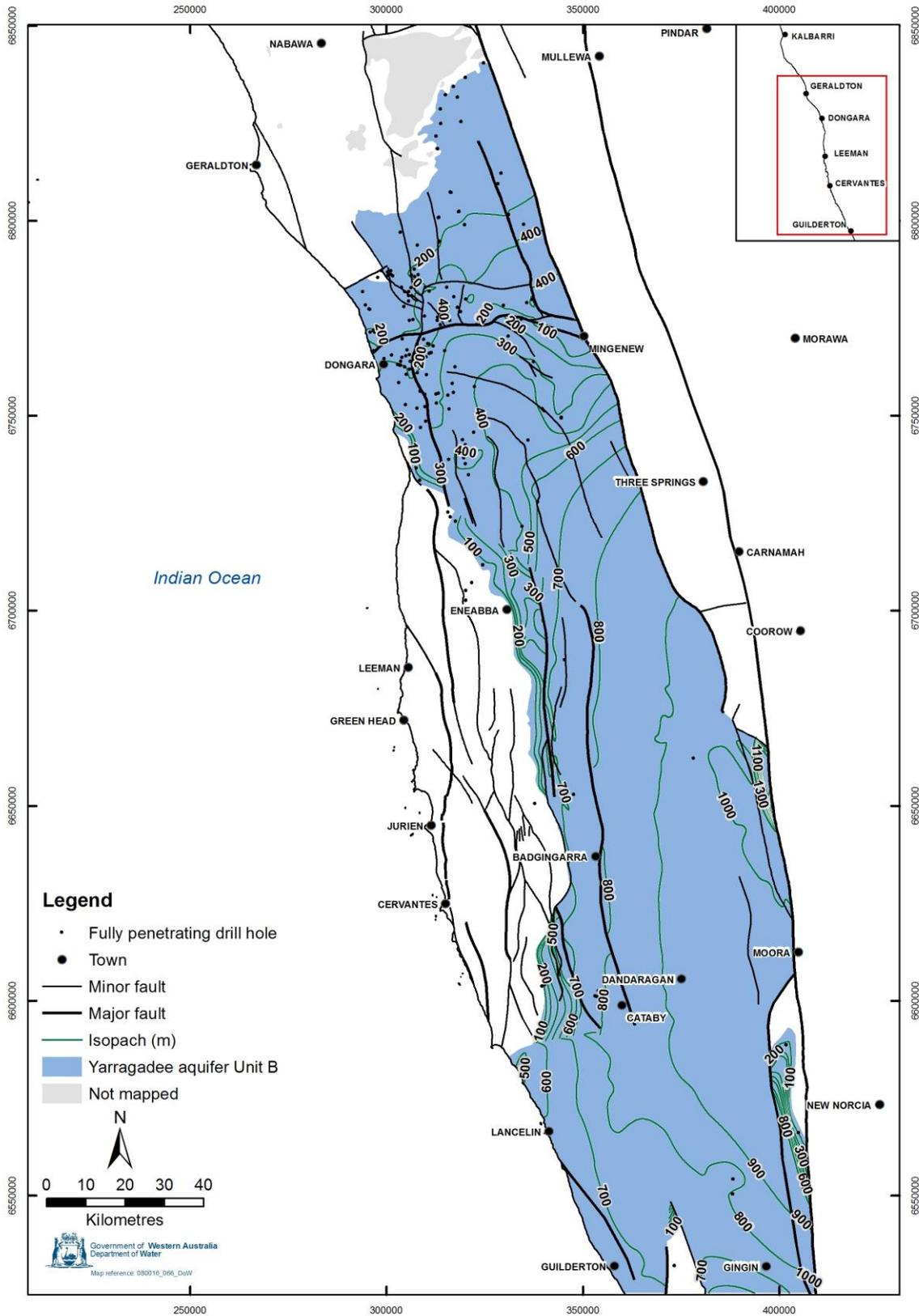
Figure 82 Yarragadee aquifer Unit B: aquifer thickness
