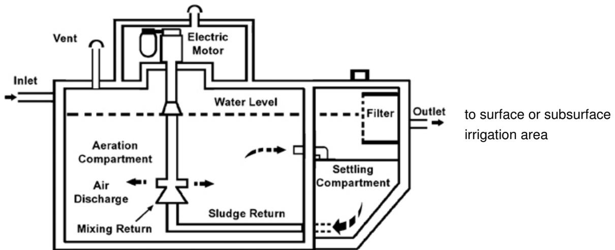
Figure 2: Diagram of typical aerobic treatment unit (without effluent disinfection)
