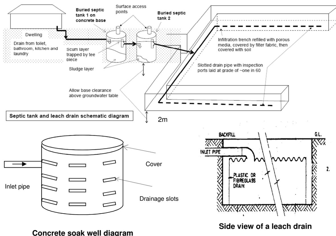
Figure 1: Conventional domestic septic tank and effluent disposal systems
