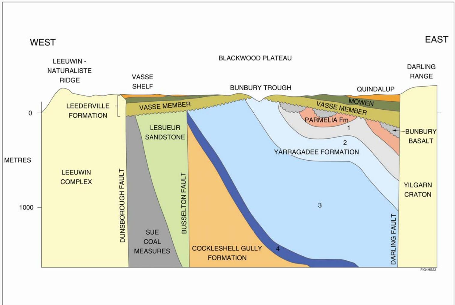
Figure 4: Geological structure
