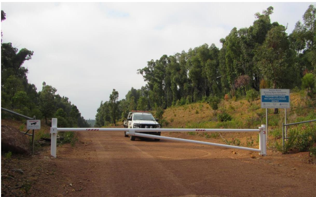
Figure C2 Typical boom gate and fencing
