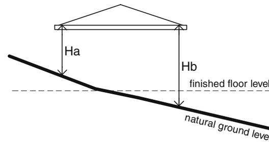
**Figure 5c – Elevation – sloped site**
