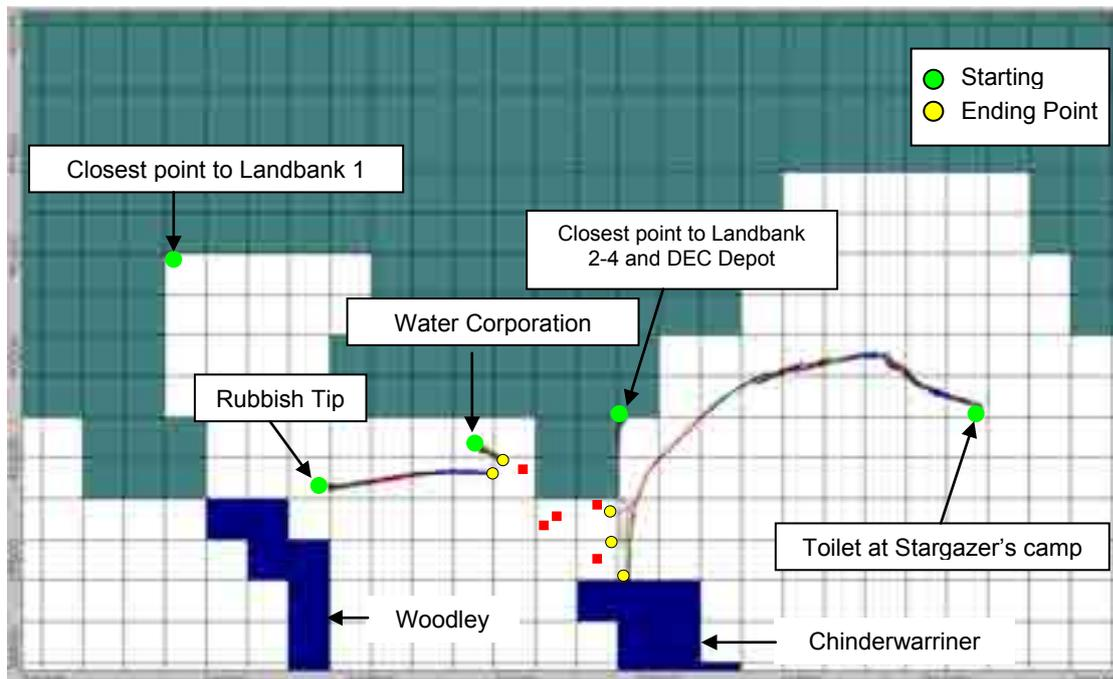
Results for the Rubbish Tip and the Water Corporation Depot sites are shown in Figure 79. The result shows that particles originating from the Water Corporation Depot site are expected to reach the nearest production well after about 120 days. Note that the particles terminate once they enter a cell containing a pumping well. Particles originating from the Rubbish Tip take about 220 days before they reach a production well.
