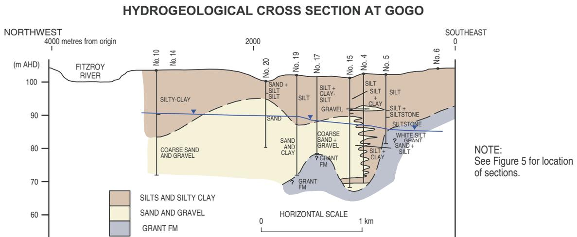
Figure 11. Hydrogeological sections at Willare, Fitzroy Barrage and Gogo
