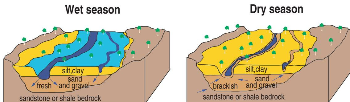
Figure 13. Conceptual model of the alluvial aquifer
