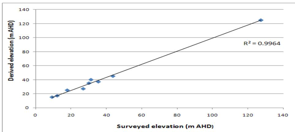
Figure 2 Comparison of surveyed and derived elevations.
