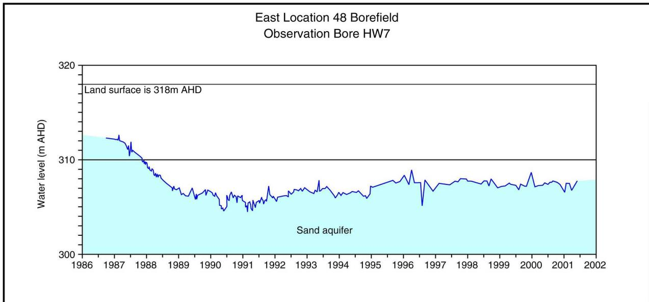
**Figure 9 Unconfined aquifer response in Bore HW7— East Location 48 Borefield.**
