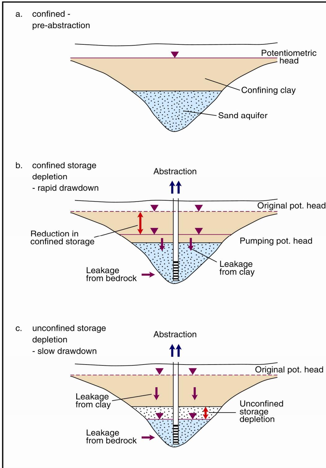
Figure 3 Diagrammatic section showing transition to unconfined state.
