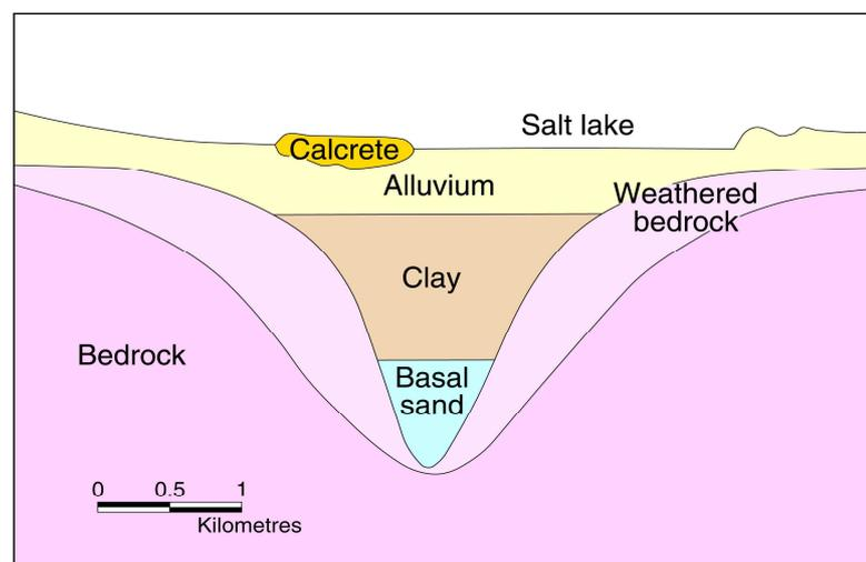
*Figure 2 Palaeochannel cross section*
