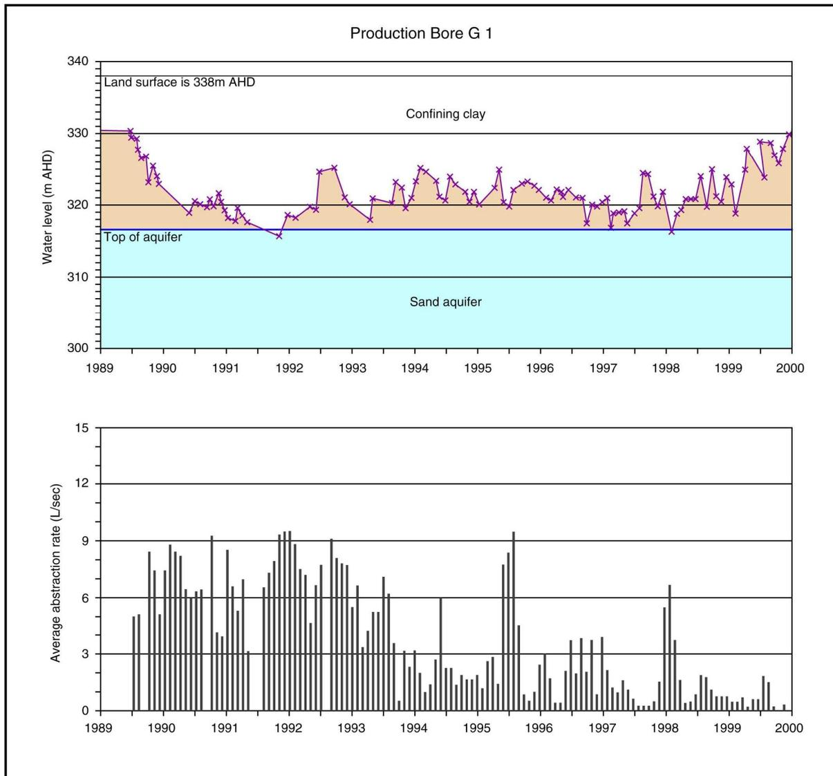
*Figure 7 Confined aquifer response in Bore G1 – KCGM Gidji Borefield. Note that blue line represents top of aquifer. Sourced from Peter Clifton and Associates (2000c)*
