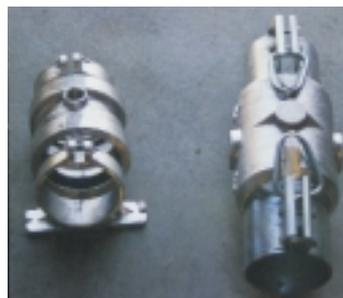
*Latch type aluminium pipe couplings (right) are less prone to failure than the twist type (left).*
