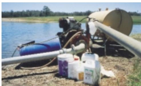
*This suction feed chemigation system, located close to a dam and unprotected, is poor practice because it presents a water pollution hazard.*
