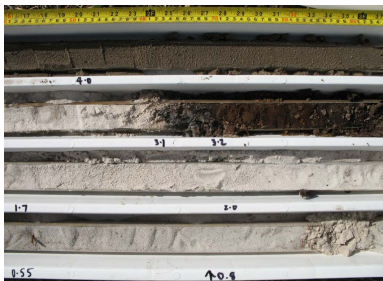
Figure 17 NTH_EC (Bassendean Sand) sharp change to ferruginised sand near the water table (Groundwater level 2.6 m bgl on 17 April 2007)
