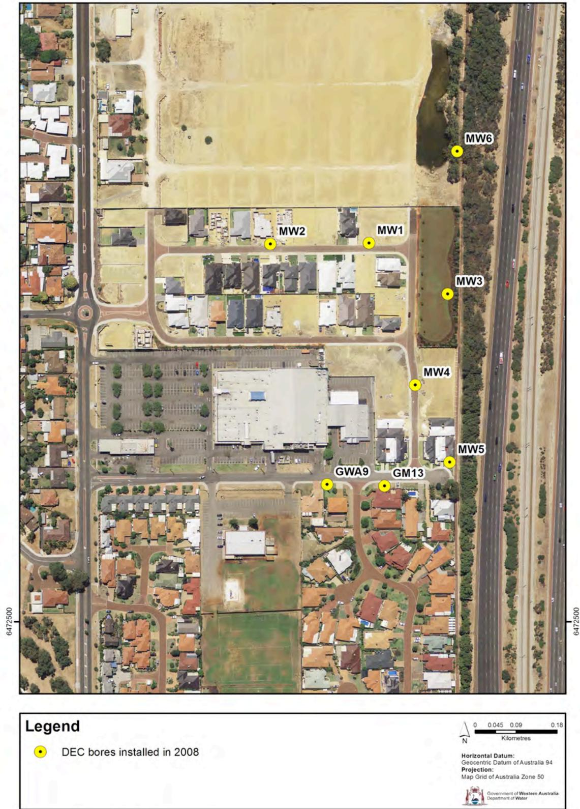
Figure 18 Groundwater monitoring bores installed by DEC in November 2008
