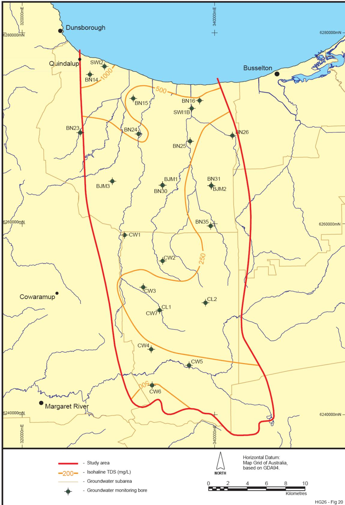
Figure 20 Isohalines for intermediate bores in the Leederville aquifer
