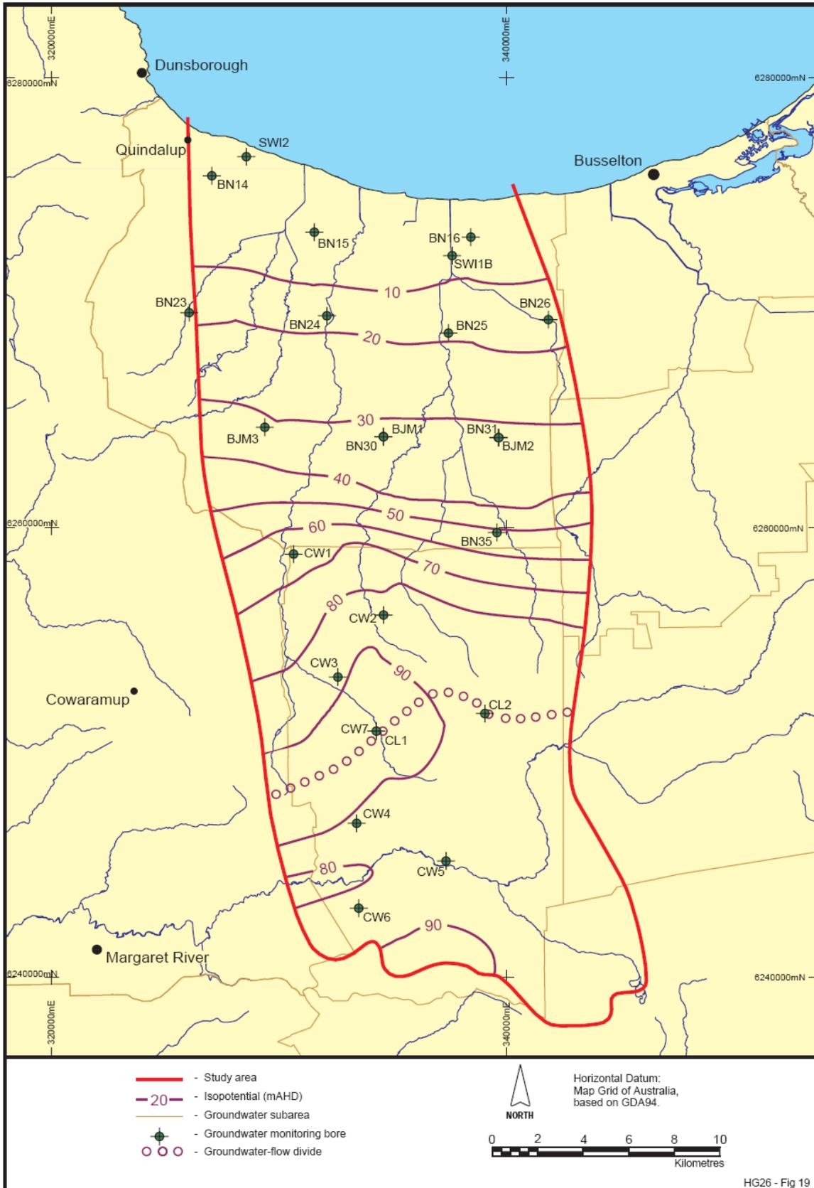
Figure 19 Isopotentials for deep bores in the Leederville aquifer
