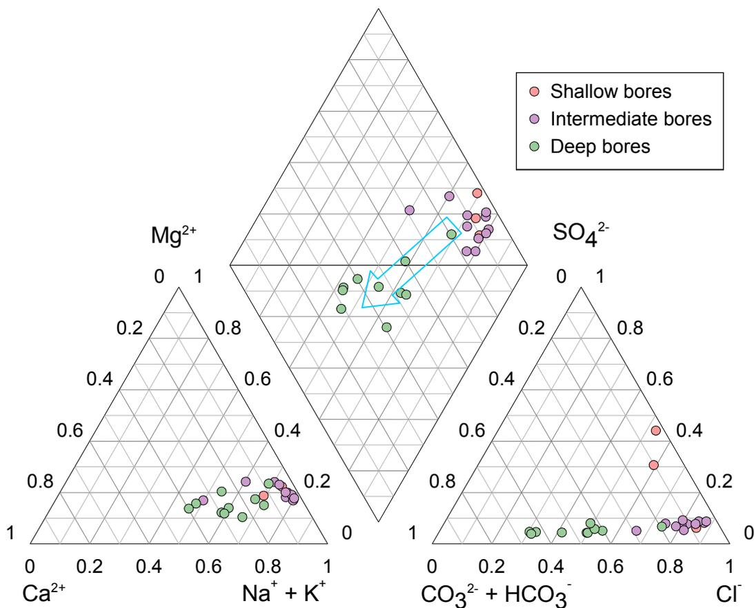
Figure 23 Piper trilinear diagram of selected chemical analyses of groundwaters
