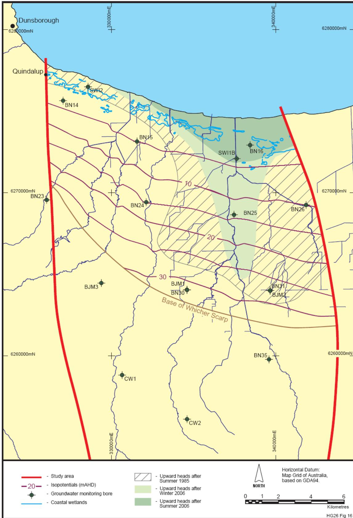
Figure 16 Watertable contours in the superficial aquifer
