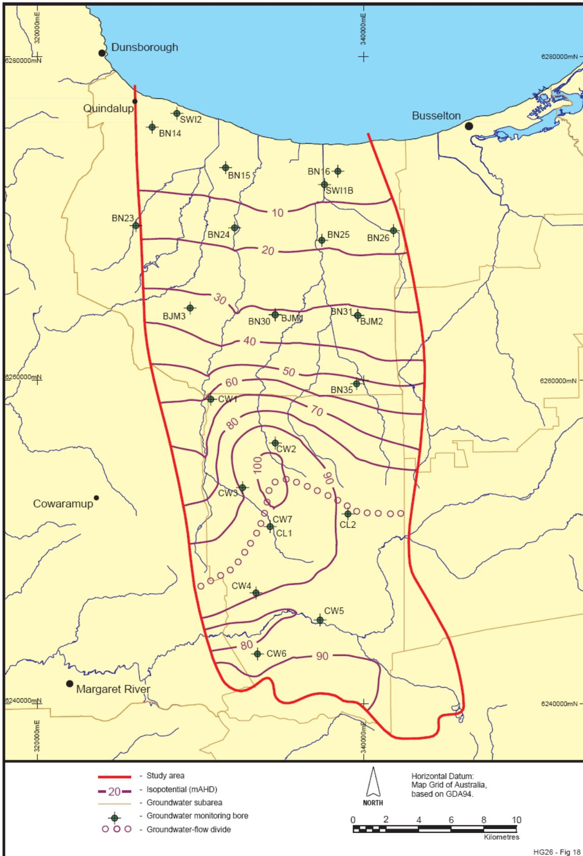
Figure 18 Isopotentials for intermediate bores in the Leederville aquifer
