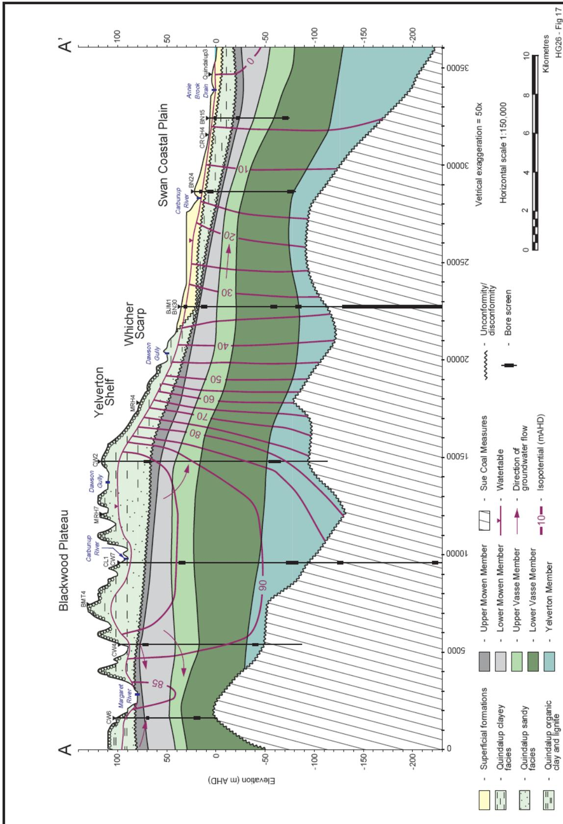
Figure 17 Schematic hydrogeological section A-A'
