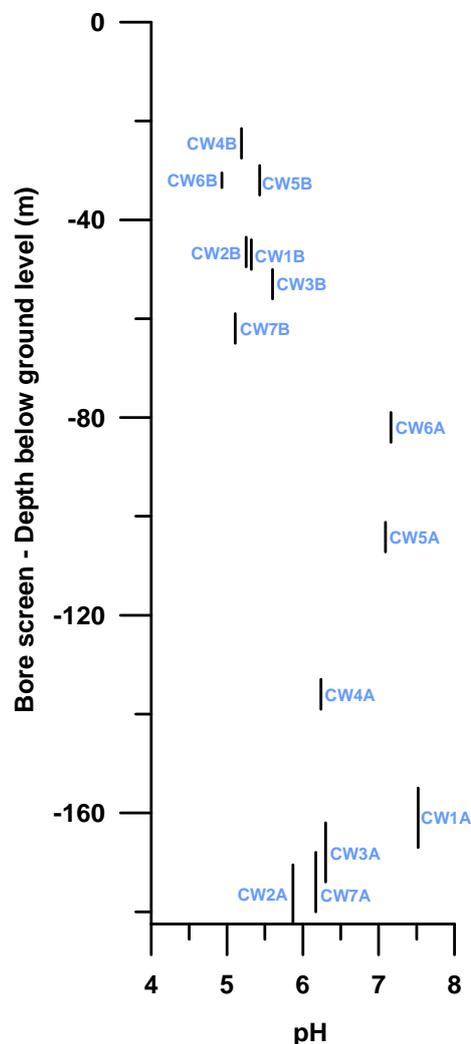
Figure 24 Plot of pH and depth in selected bores
