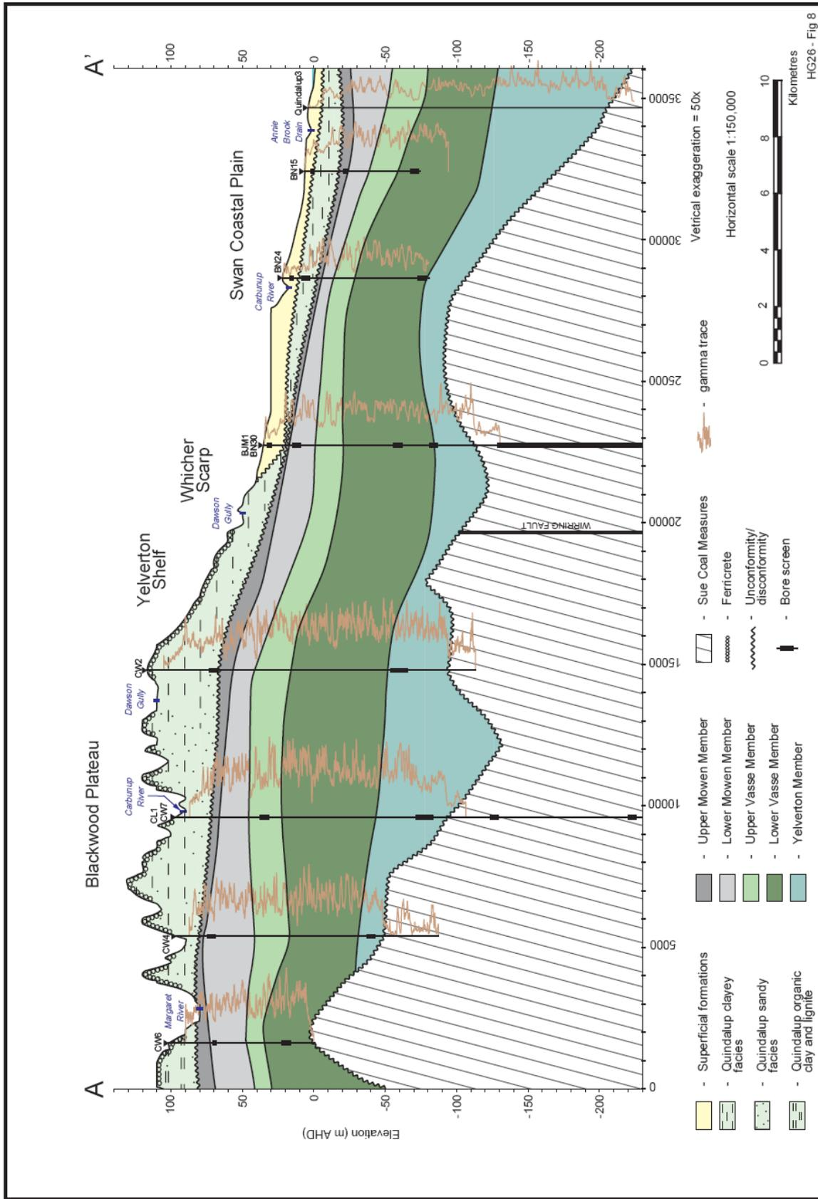
Figure 8 Stratigraphical cross-section A-A'
