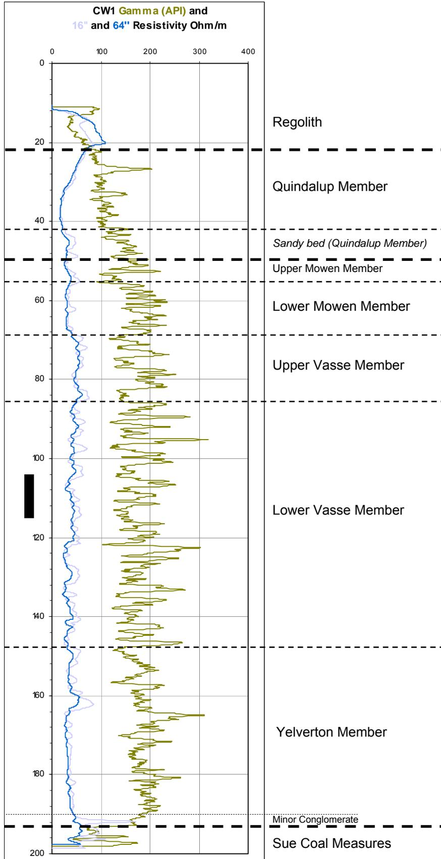
Figure 10 Geophysical log of Bore CW1
