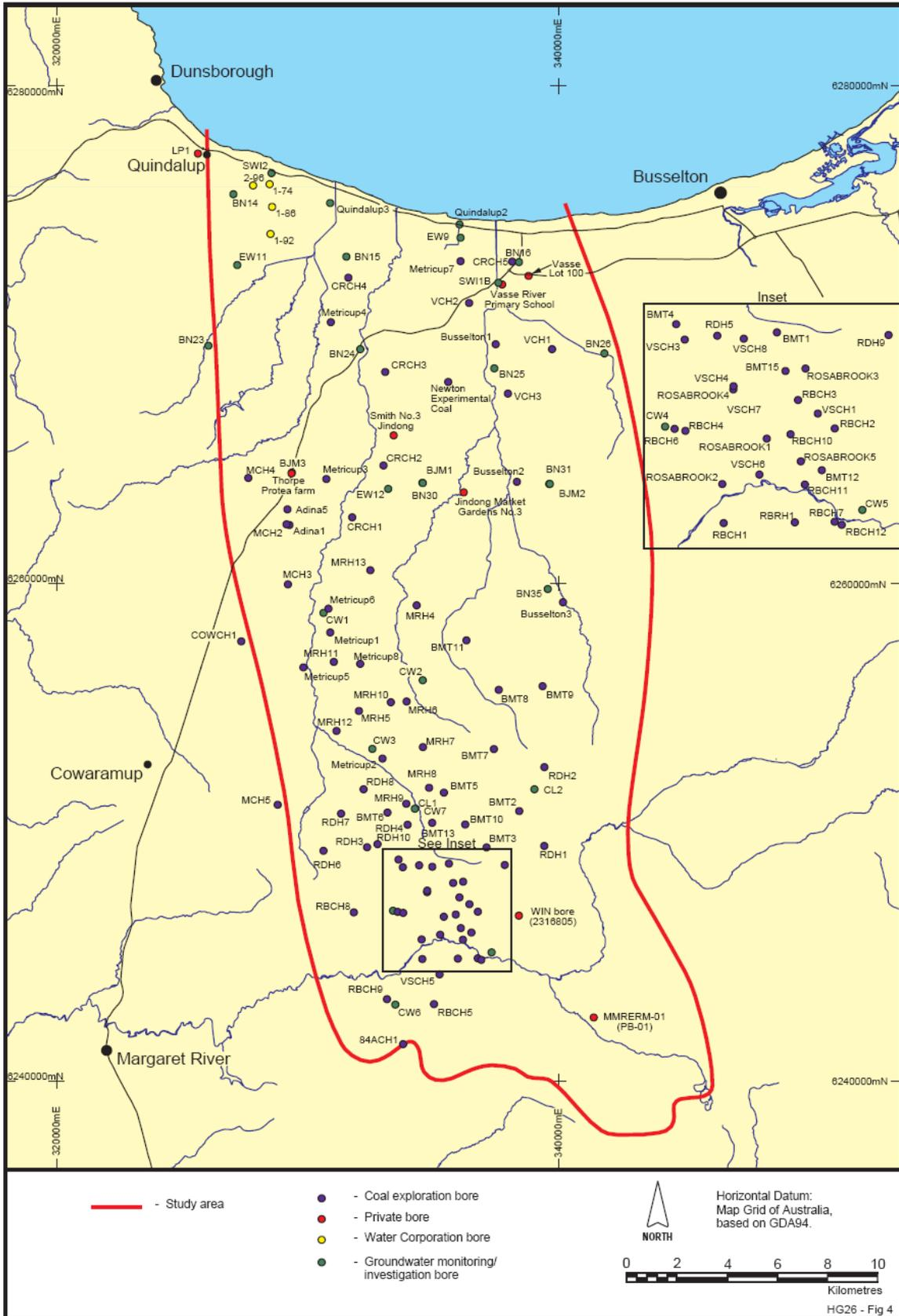
Figure 4 Groundwater monitoring bores and coal exploration drill holes
