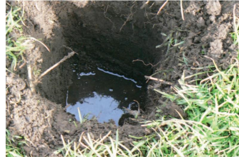
Test hole to check water depth
