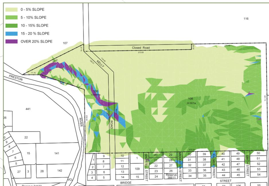
Figure 5 - Slope Analysis Plan
