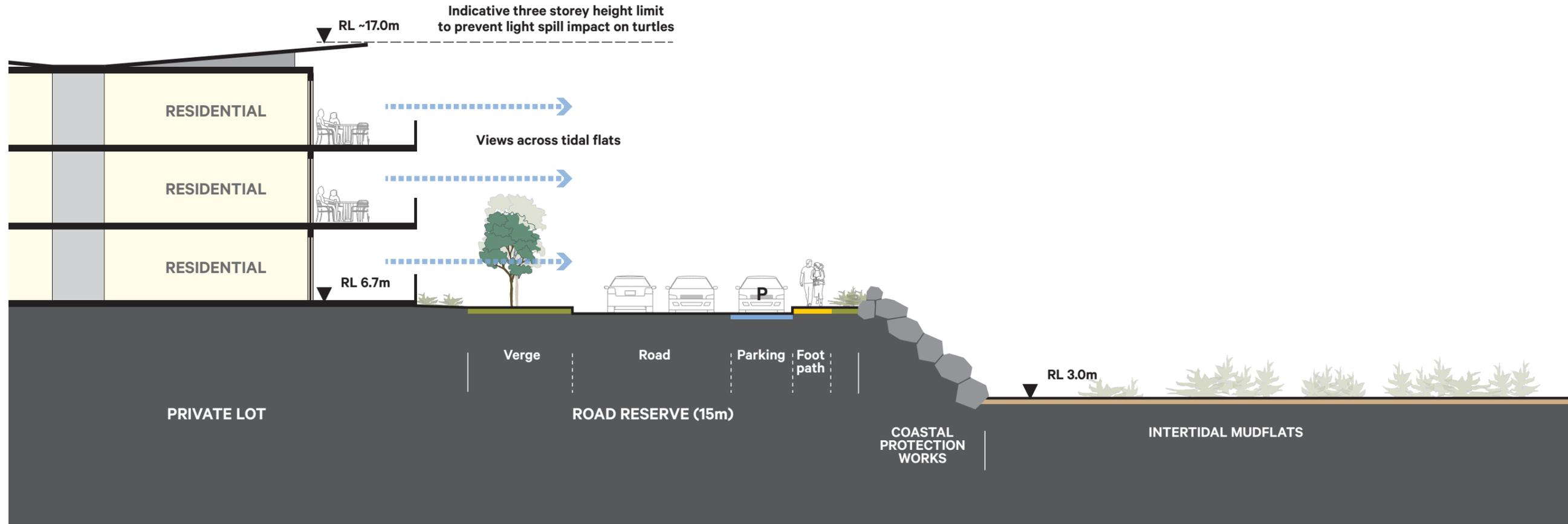
Indicative section showing relationship of road, pedestrian footpath, coastal protection works and level change to mudflats.
