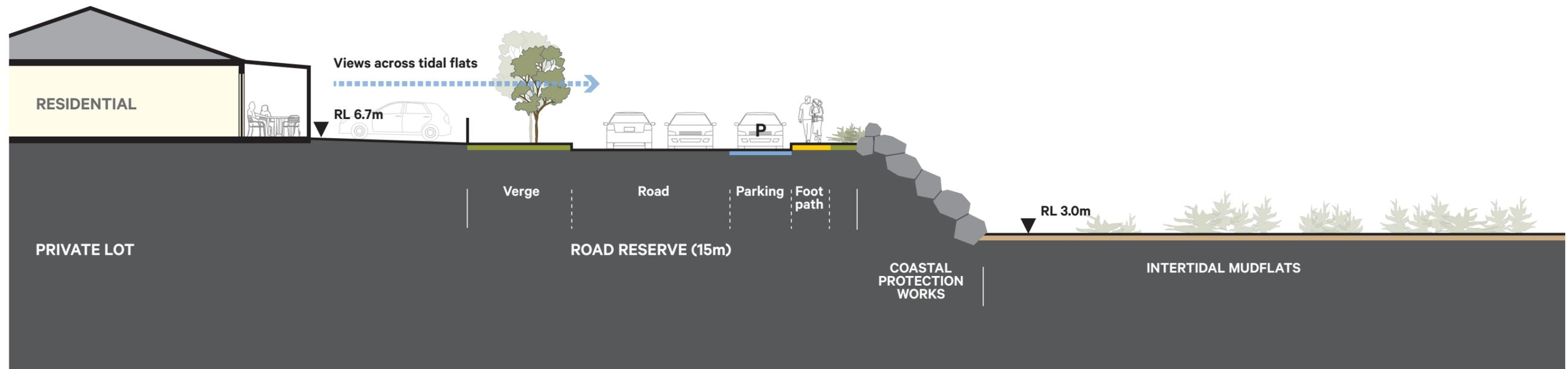
Indicative section showing relationship of road, pedestrian footpath, coastal protection works and level change to mudflats.
