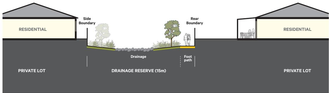
Indicative section showing arrangement of drainage link and footpath to proposed dwellings.
