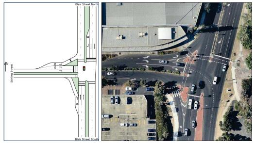
Figure 6-4 Indicative Layout for the Blair Street/Stirling Street Intersection
