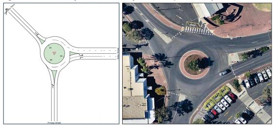
Figure 6-6 Indicative Layout for the Carmody Place/Prinsep Street/Haley Street Intersection
