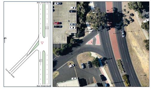
Figure 6-7 Indicative Layout for the Cornwall Street/Blair Street Intersection
