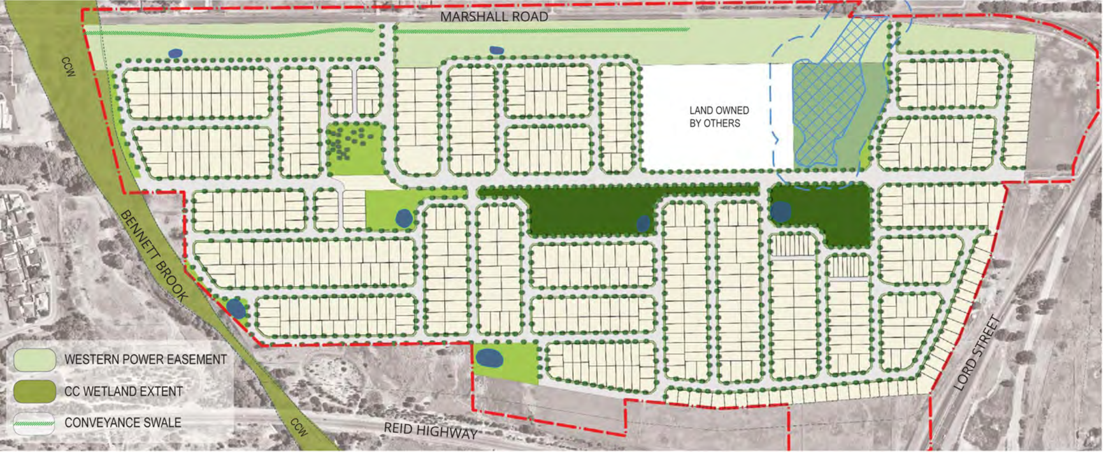
FIGURE 20 - STORM WATER TREATMENT
