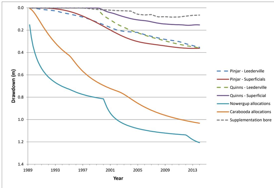
**Figure 7-4 Transient simulation using zone of low hydraulic conductivity in Superficial aquifer west of Lake Nowergup - watertable drawdown, Layer 1 (Superficial aquifer) beneath Lake Nowergup.**
