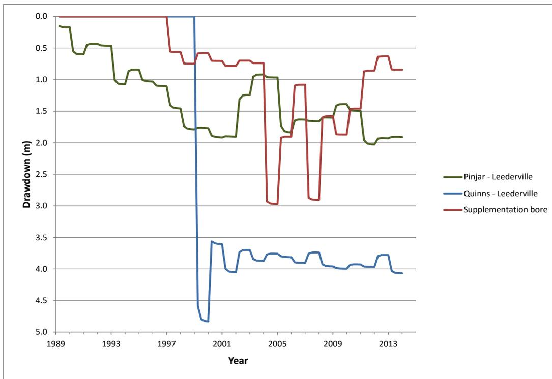
**Figure 7-3 Transient simulation - potentiometric head drawdown, Layer 2 (Leederville aquifer) beneath Lake Nowergup.**
