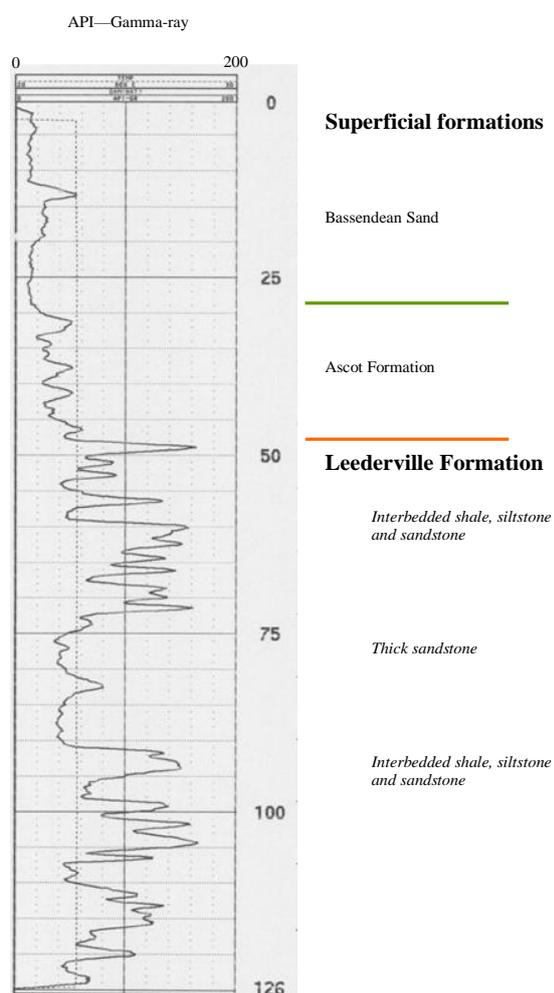
**Figure 3-3 Downhole gamma-ray log bore 2/00.**
