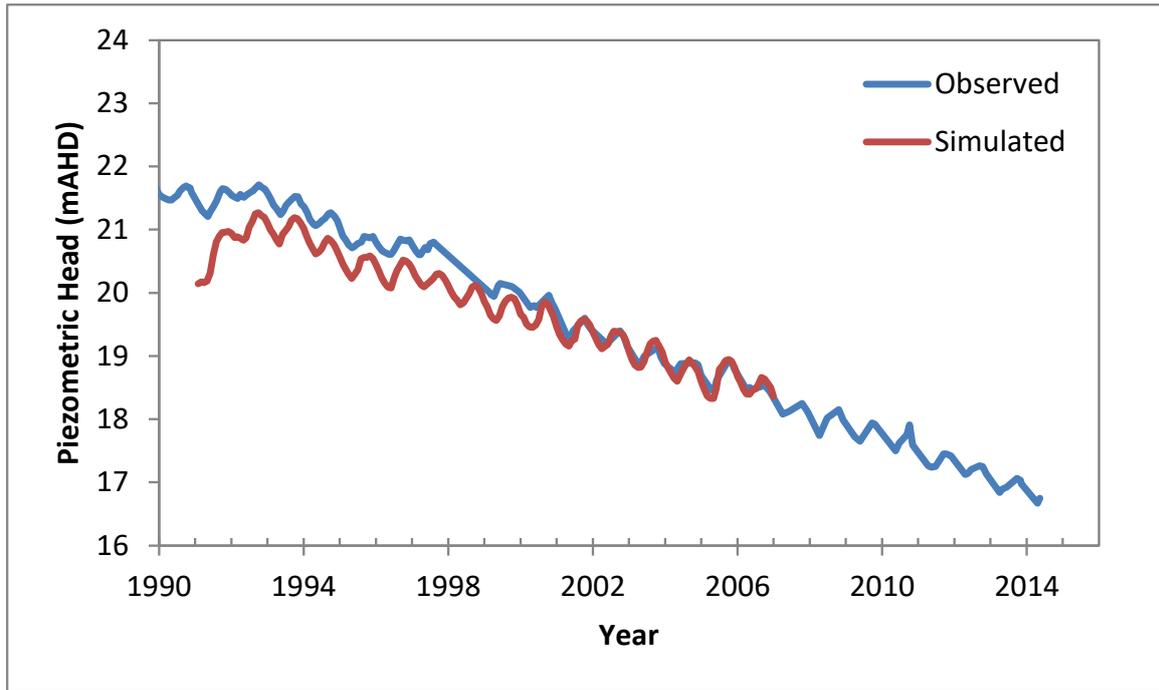
Figure 6-3 Observed and simulated head - Bore PM33, Superficial formations.
