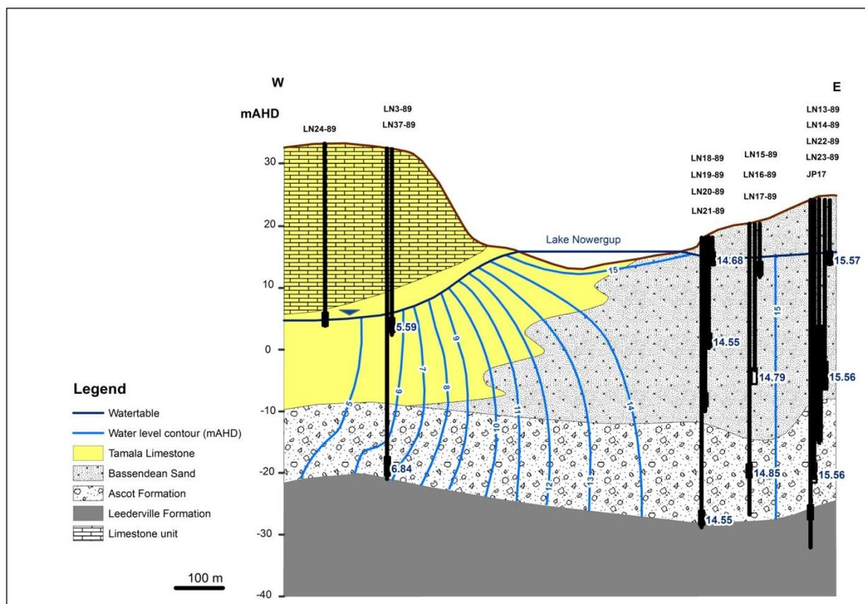
Figure 4-3 Hydrogeological cross-section - Lake Nowergup (2014).
