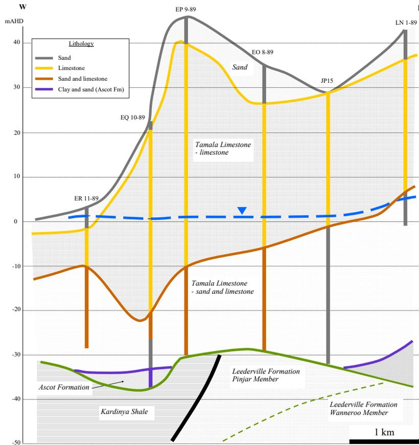
Figure 3-4 East - west geological cross-section west of Lake Nowergup.
