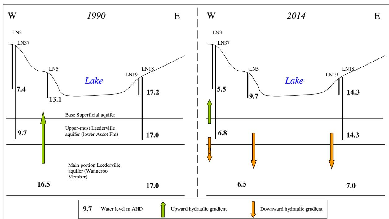
**Figure 5-18 Water levels and hydraulic gradient beneath Lake Nowergup - 1990 and 2014.**
