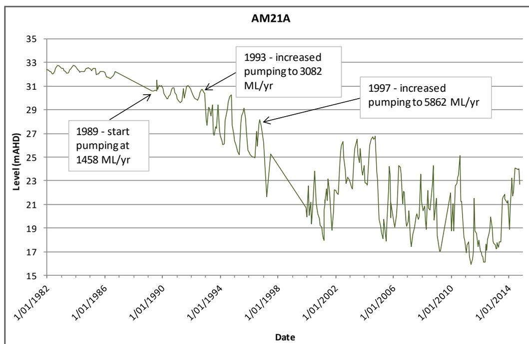
**Figure 5-17 Leederville aquifer hydrograph - Pinjar Leederville borefield operation.**
